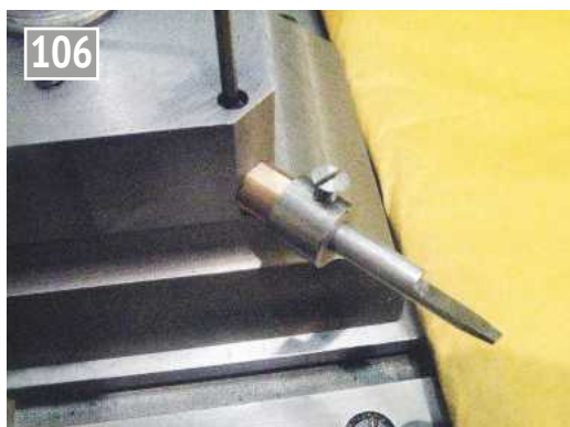
Finding the depth to ream the socket - 1: push the centred end in and lock the collar.
