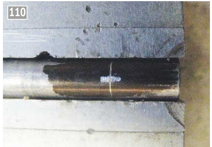
110 Move the caliper to - (minus) 1.1mm and use the caliper to set the size to scribe from the end of the detent pin. Use a diamond burr to mark the top, centre punch and drill. The punch mark is there but lighting makes it invisible.
