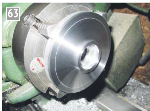
Turning the front bearing plate.
