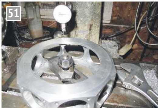
Clocking the reference face square.
