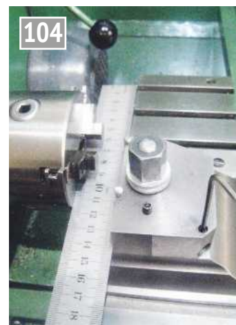
Set the top slide to turn perfectly parallel then set the block square with the ruler trick.
