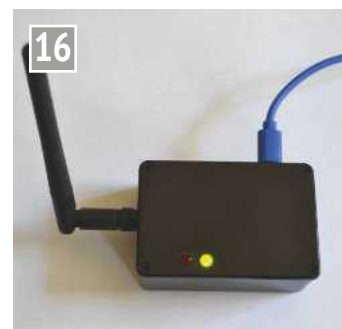
Laptop radio interface, based on a radio module and a USB/SPI interface module.
