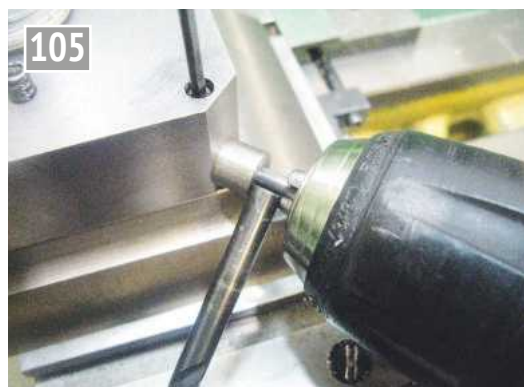
Setting the depth of the pilot hole with a 6mm drill shank.
