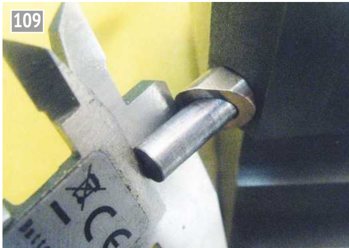
109 Measuring to get the lever arm in the correct position. Record the size and zero the caliper.
