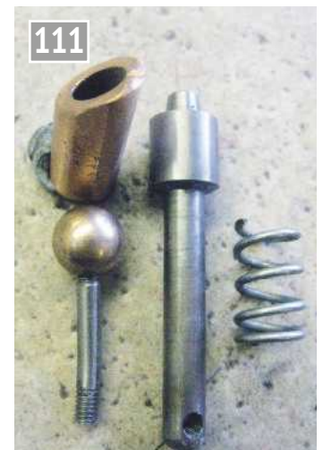
111 The finished detent components. Note the tiny notch - it must be small!
