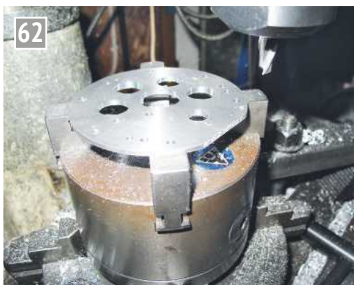
Machining the flat.
