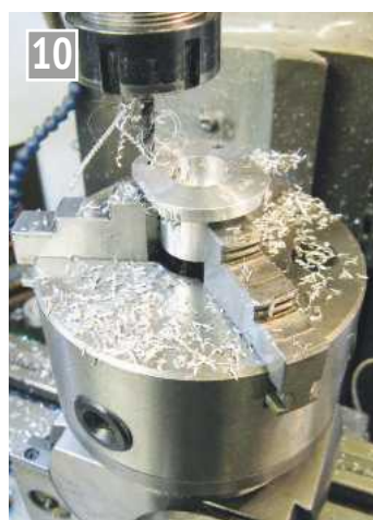
10 Drilling the thrust bearing housing for the mounting screws.
