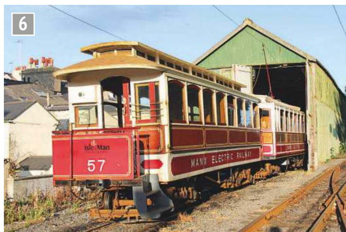
MER cars could almost come from an American Interurban. No 57 at Ramsey. This car was built by the Electric Railway and Tramway Works in 1904. Note the distinctive high clerestory.
