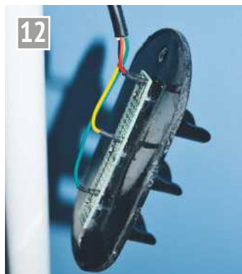
Inside a signal head. The three 10mm LEDs are mounted on a small piece of matrix board.
