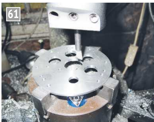
Finish the central offset bore.
