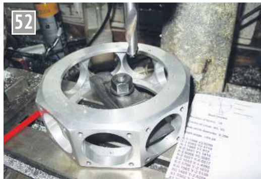
Pitching out the hole centres.
