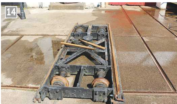
14 Horse tram traverser at depot.
