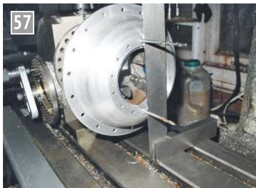
Setting the cover true to previously drilled holes.
