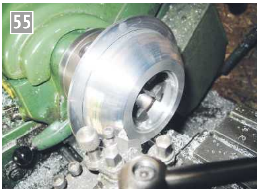
Roughing the outside curve.
