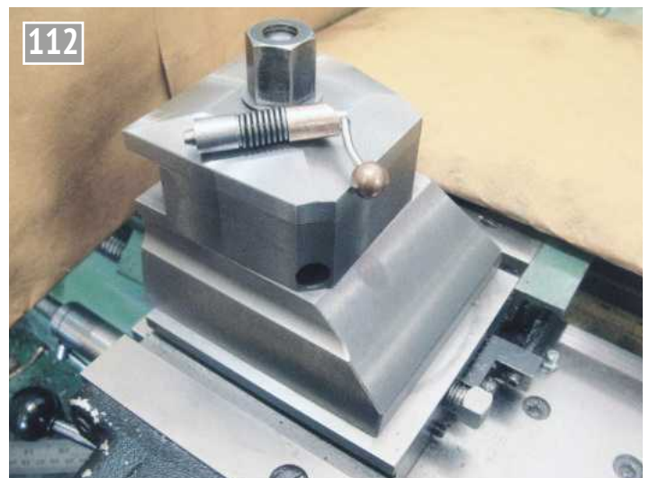
112 The finished tool post and detent pin assembly on my solid mount. I had to change the spring shown in photo 111.
