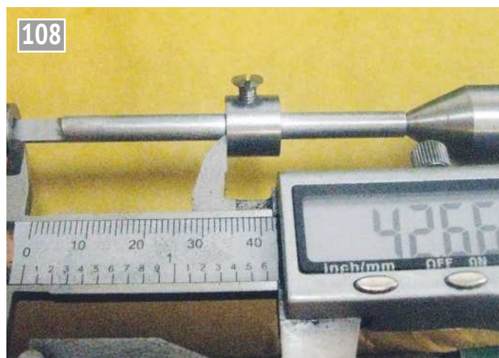
108 Finding the depth to ream the socket – 3: mount the reamer between the special bush and centre. The dimension is irrelevant. The bush and collar size are too small making it difficult as only the tips of the calipers are engaged.
