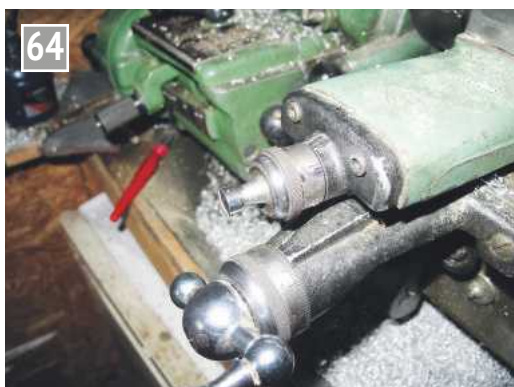
Arrangement of the compound slide to turn the angled face.
