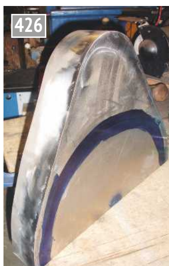
Final drive guard cleaned up.
