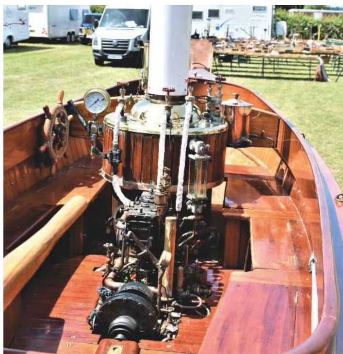
The engine and drive system on Paul Nind's 18 foot steam boat which is fitted with both a tiller and a side mounted steering wheel.
