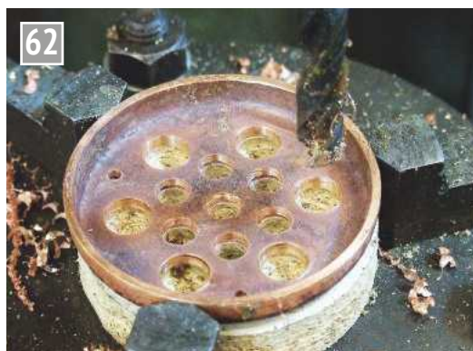
Completed firebox tubeplate.
