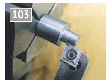
103 Accurately centre the detent pin before turning the taper.
