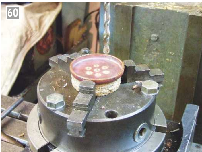
Inner Firetube holes drilled.
