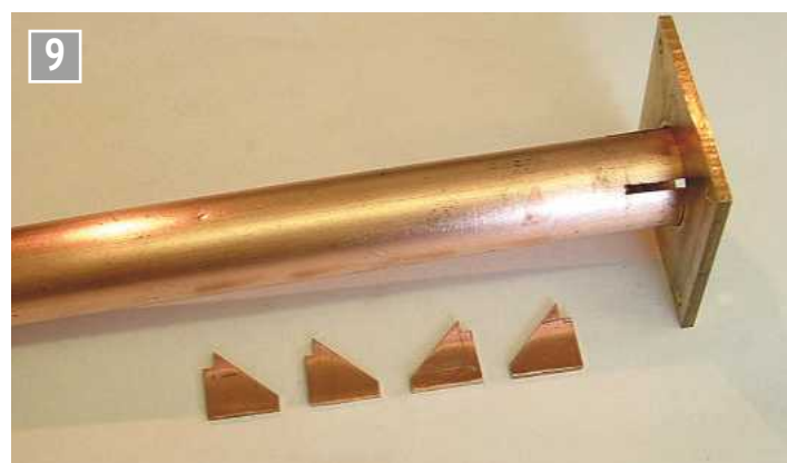
Four slots to accommodate the four stiffeners.
