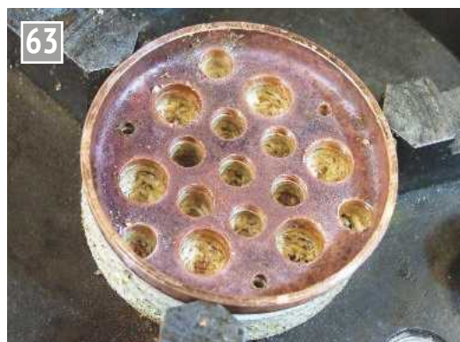
Completed smokeybox tubeplate with additional bush drillings.
