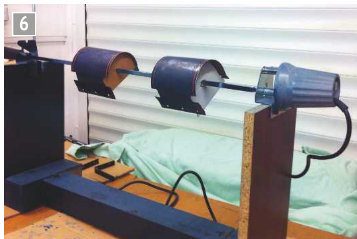
Cylinder cleading had to be painted by hand.
