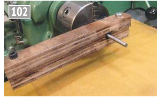
102 Lapping in progress.
