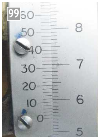
Vernier scale on a height gauge reading 54.36mm (0.02mm resolution).
