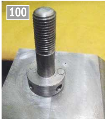
100 Finished indexing ring showing positions of holes - ensure the pin hole will not hit any of the tapped holes in the top slide. If using the pin, only use one grub screw.
