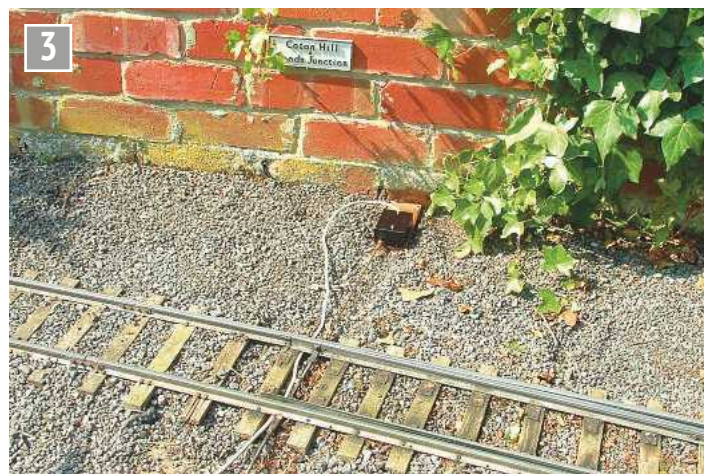
A detector box in position.
