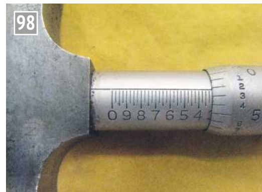
Depth and inside micrometers are numbered from the left.
