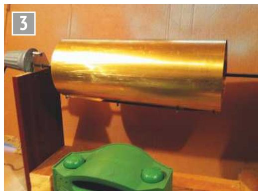
The boiler barrel ready for painting.
