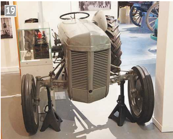
The 'wee grey Fergie' designed by Harry Ferguson incorporated his three point linkage for pulling ploughs. It was especially popular in Ireland. This model was made in 1948 by Standard at Coventry. (Item number 80/68)
