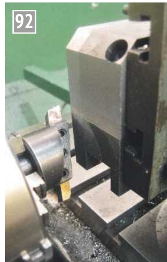
Profiling - vertical slide method.
