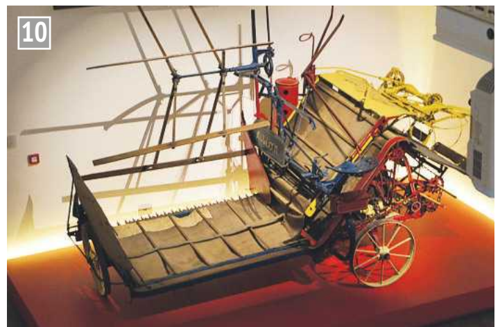
The Albion reaper was made in Leigh, Lancashire and proved highly popular. Similar reaper binders were still used on Herefordshire farms in the 1950's. (Item number 80/69)
