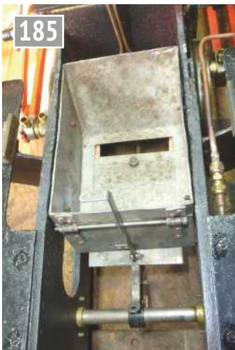
Ashpan with ash door partly open.
