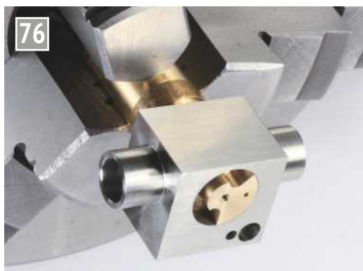
The throttle valve is adjusted to the carburettor case's inner diameter. In front the high/low stop dogs are visible.
