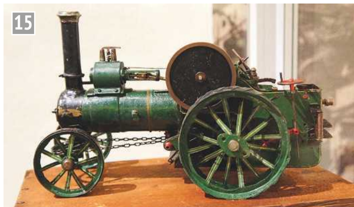
Working model of a single cylinder road locomotive made by George A. Froud in 1921 at the age of 16; the first model engine he made. Scale 1/2 inch : foot (1/24 scale) (Item number 63/183)
