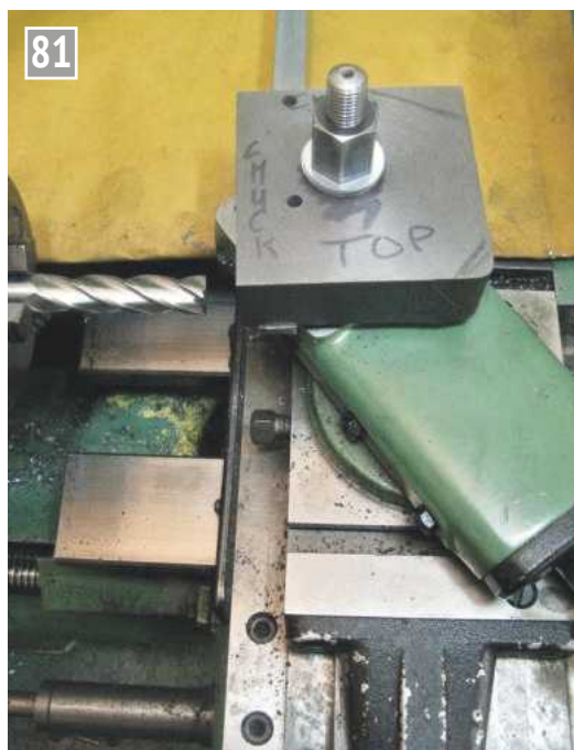
Angling the top slide for milling the step.
