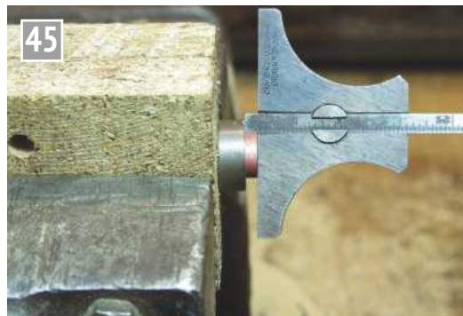
Setting tube protrusion prior to flaring.
