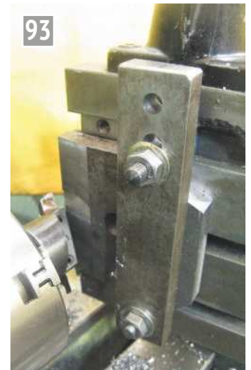
Cutting the cap angles. This makes the unit seem a lot lighter.
