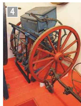
Jethro Tull's invention of the seed drill made seed sowing less wasteful and enabled use of horse drawn hoes to suppress weeds. Many different types were made. (Item number 65/326)
