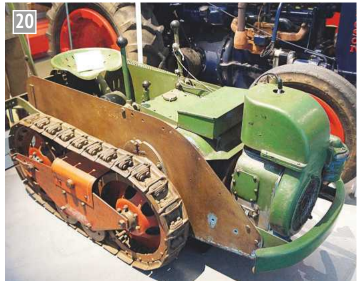
1953 Ransomes MG crawler tractor used in the grounds of a hospital. Larger versions were used in the Fens as they did not consolidate soil like other tractors. (Item number 81/146)
