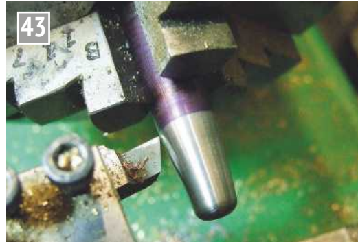
Machining large end of flaring drift.
