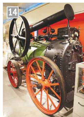
Clayton and Shuttleworth portable steam engine. Hauled by horses between farms to work threshing machines or other equipment. (Item number 51/1284)
