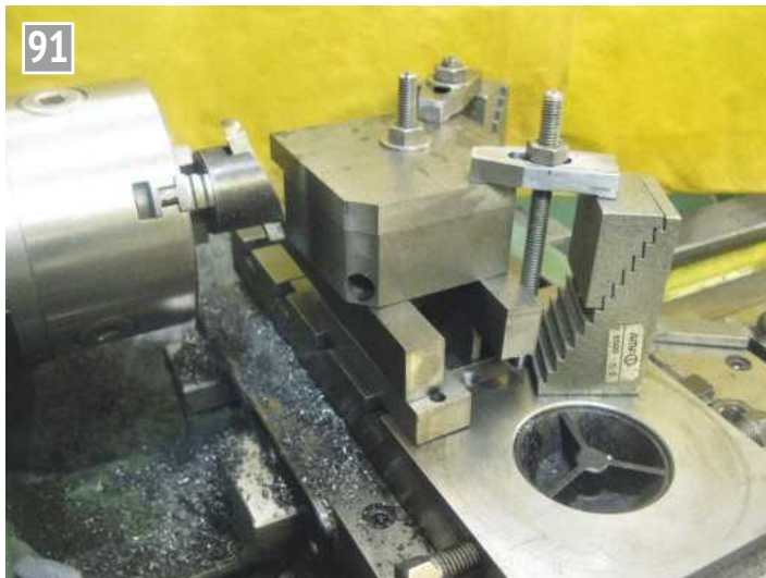
Profiling the block and cap at the same setting - cross slide method.
