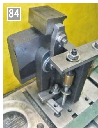
Tail stock view of the use of an angle plate to hold the block for milling the step. Ugly!
