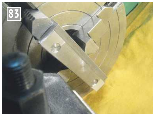
How to face the packing to size, mounted on what will be a tool holder.
