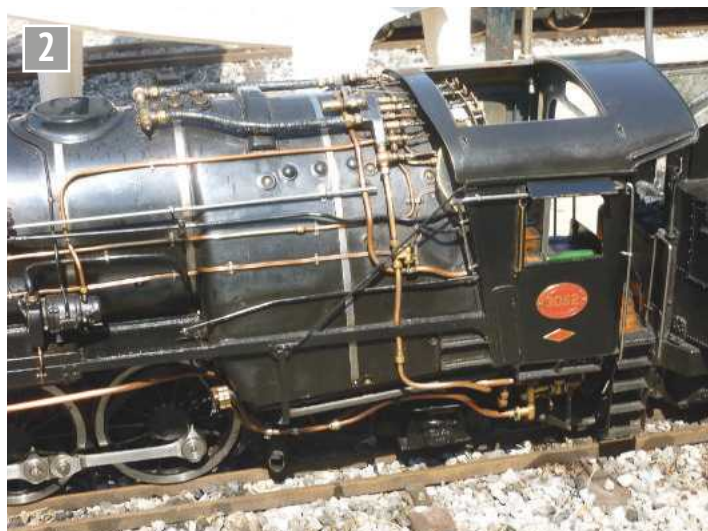
15F piping at GCMES.
