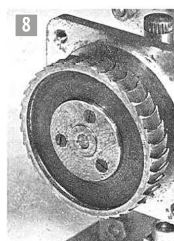
Stumpf type rotor by E.T. Westbury (ref 1).
