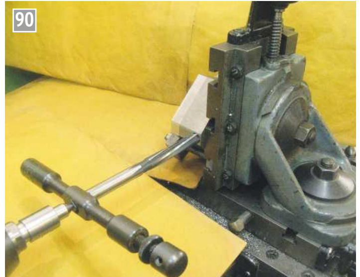
Reaming the hole - pump centre in action again!
