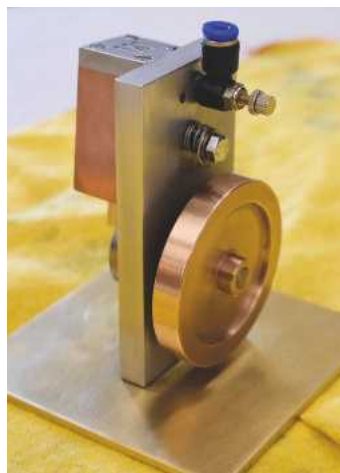
A superb little Oscillating engine built by 12 year old Matthew Kennington.
