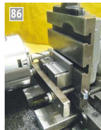
Milling the step the easy way on the vertical slide.
