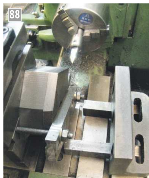
Setting the hole position for the detent pin.
