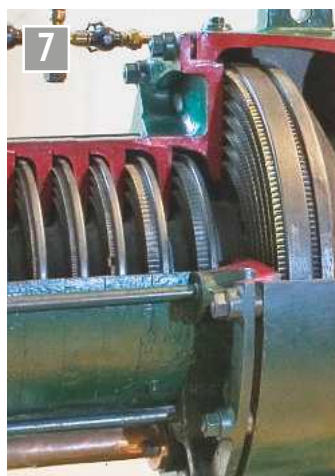
Radial flow turbine built by C.A. Parsons part of a turbogenerator installed at Cambridge in 1892. Now in the London Science Museum. (Image from Science and Society Picture Library.)
