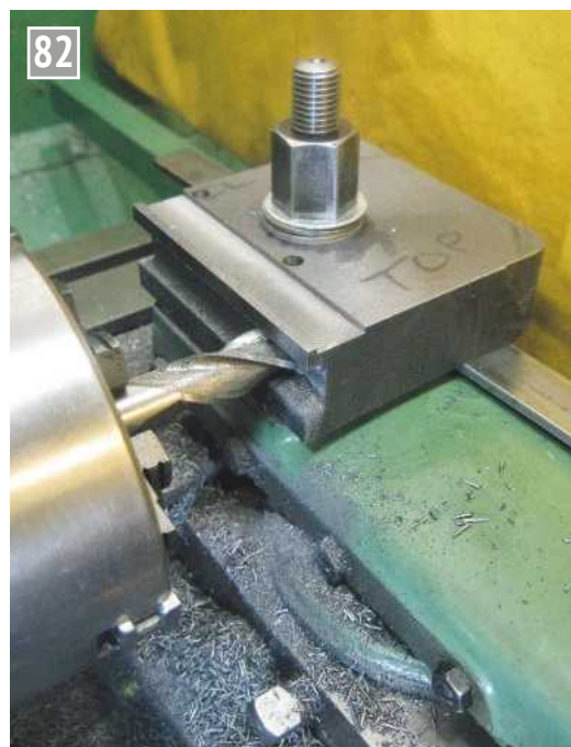
Step milling in progress - note packing strips to set the step height of 6mm.
