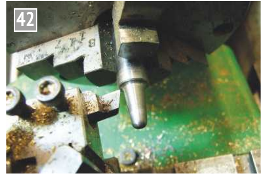
Machining small end of flaring drift.
