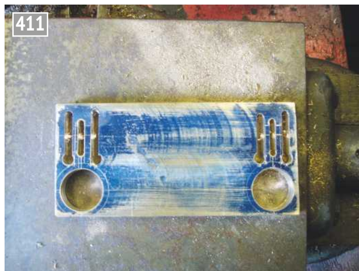
Lever supports ready for finishing.
