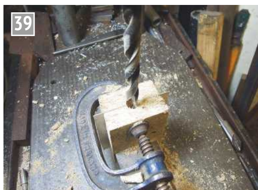
Drilling the tube flaring clamp.
