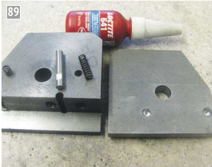
The main block assembly with the Loctite, springs and pins.
