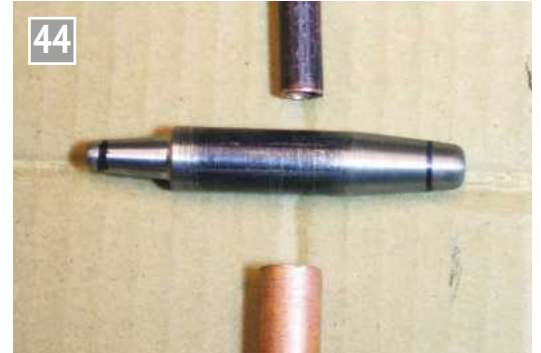
Completed flaring drift.
