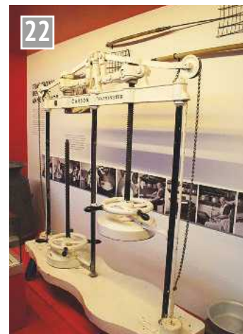
Cast iron cheese press made by Carson of Warminster. Many local foundries produced farm equipment, this was obviously aimed at the Wiltshire dairying market. (tem number 87/31)
