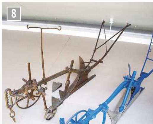
Ransome RHB plough introduced in 1873. Ransomes' invention of the chilled cast iron ploughshare and clever marketing made his firm a leading maker. (Item number 79/34)
