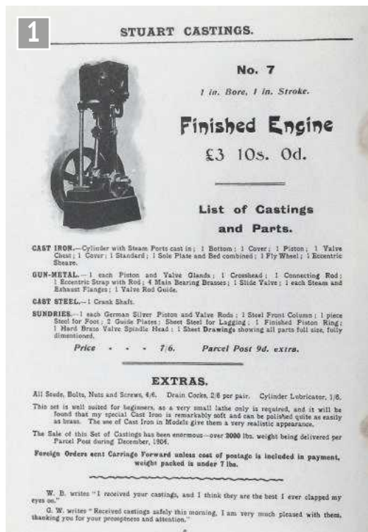
The No. 7 as illustrated in the Stuart Turner 1906 catalogue detailing materials used.
