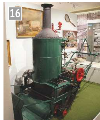
Magnificent steam lawn mower built by Ransomes. (Item number 55/338)
