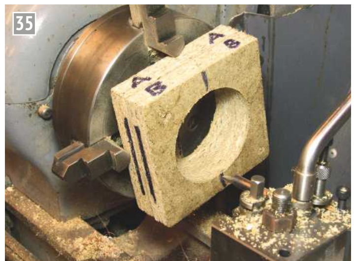
Tube nest plate bored to accept boiler barrel.
