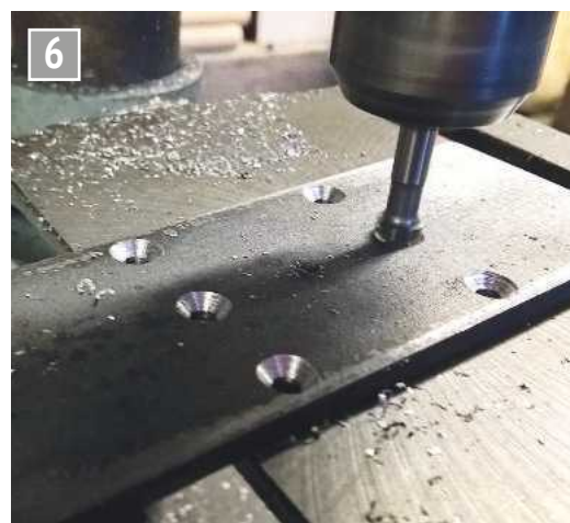
6 Countersinking the fixings for the fixed blocks.
