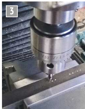
Using the mill to mark out the bearing blocks.
