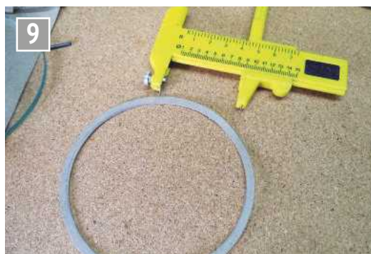
Cardboard packing rings cut out using gasket cutter.
