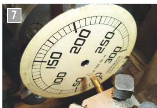
Boring out the enameled face.
