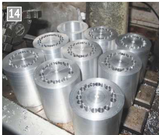
Completed chain drilling.
