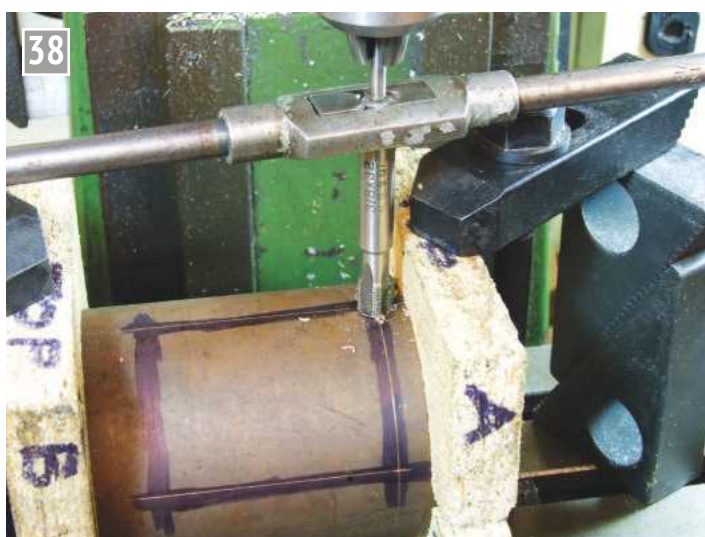
Tapping barrel for bush.
