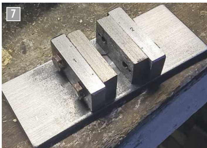
The jig with a pair of bearing blocks attached.
