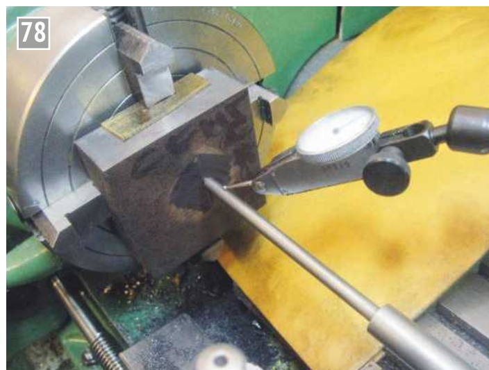
Setting the centre hole true with DTI and wobbler.
