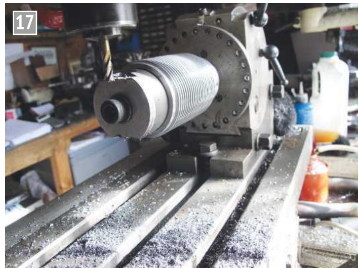
Milling the final assembly.
