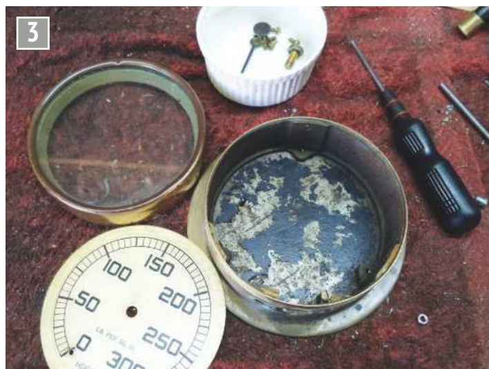
Gauge stripped down.
