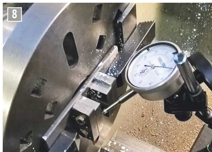
Checking that the bored recess is running true.
