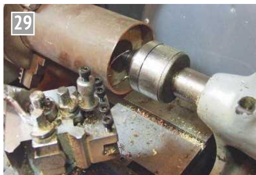
Truing up the barrel end.
