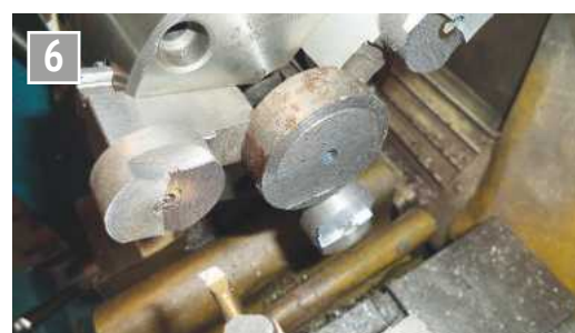
Boring out soft jaw extensions to fit face.
