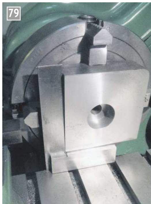
Setting the block chuck face vertical prior to marking out for the pins.
