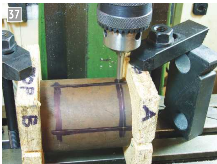
Locating spindle to bush location.
