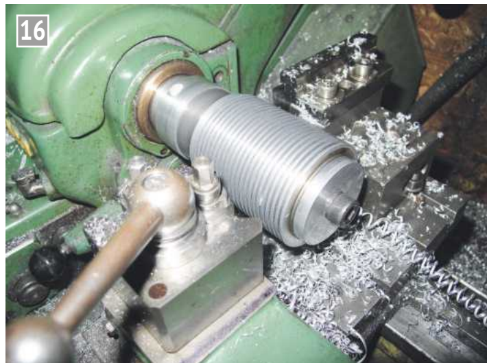
Finish turning the cooling muffs.
