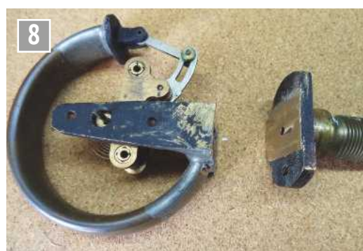
Bourdon tube cut off from pipe thread.
