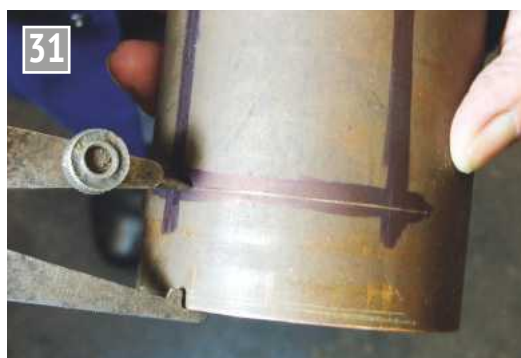
Marking the bush horizontal location.
