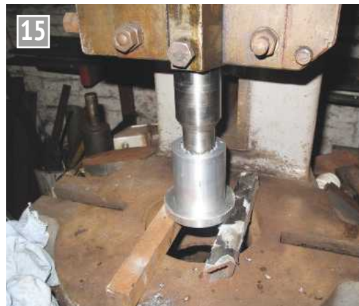
Breaking the webs under a fly press.
