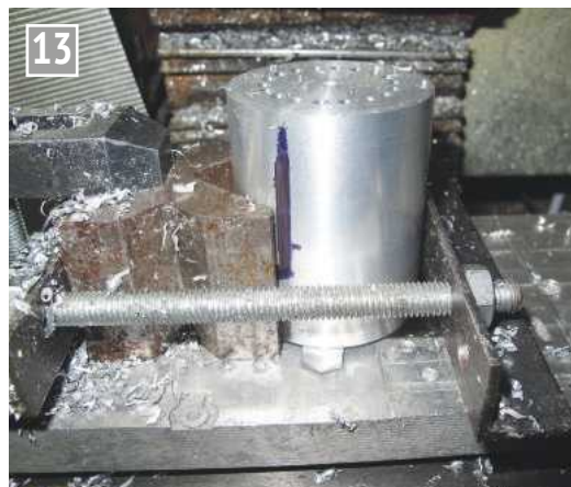
Marking the billet before reversing.
