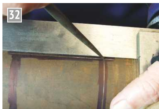
Marking the bush vertical location.
