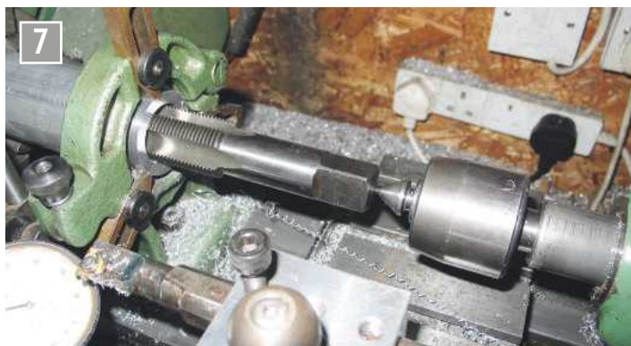
Finishing the thread using a plug tap.
