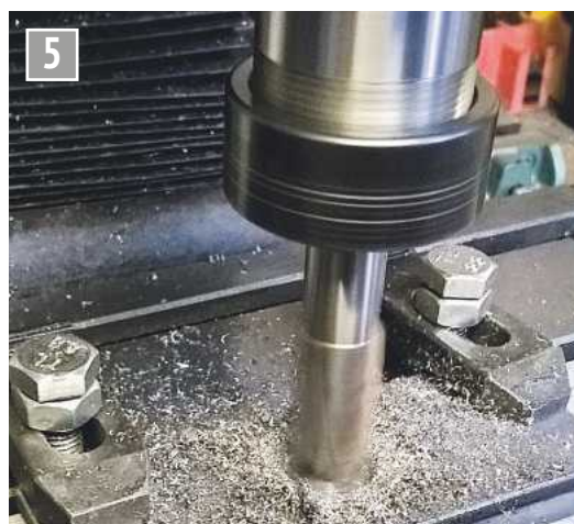
5 Milling out the recess in the plate.
