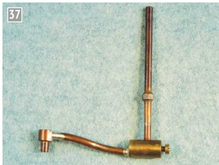
The exhaust pipe assembly.
