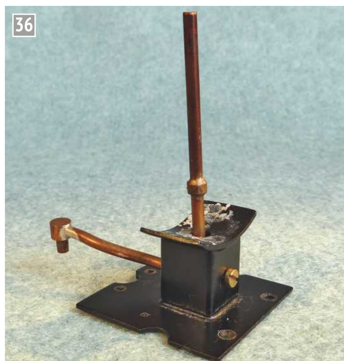
The smokebox support, with exhaust pipe.
