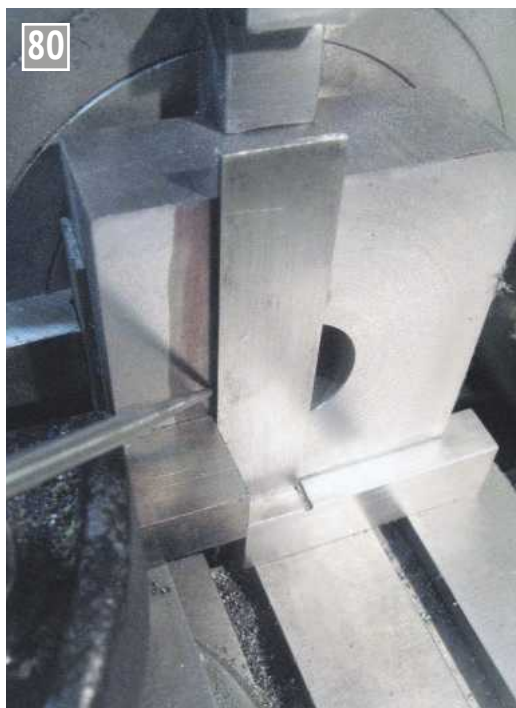
Use the cross-slide dial to mark the exact pin position.
