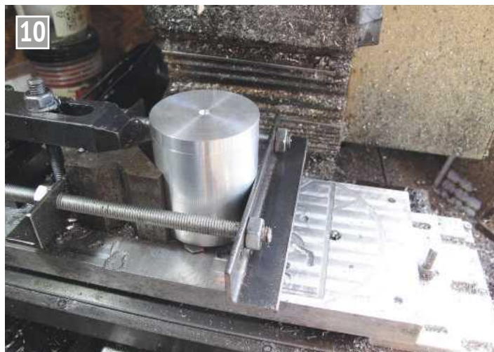
Cooling muff billet secured for chain drilling.
