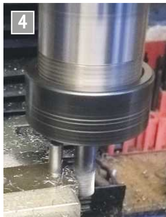
Cleaning up the ends of the bearing block.
