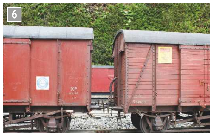
A Diagram 1458 12T Southern Van with working vacuum brake all piped up.
