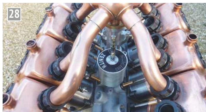
Half scale E.N.V. aviation motor with Zenith carburettor in place.
