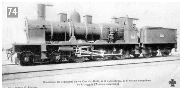
Midi 1424 of the small wheel (1.600m) 1400 class. The first French de Glehn 4-6-0 and the smallest driving wheels anywhere in France at 1.600m.
