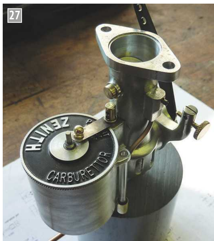
Reproduction half scale Zenith carburettor.
