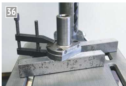
Drilling the holes in the transfer plate, using the original diehead shank as a drilling jig.
