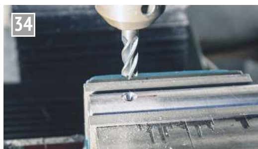
Creating a flat seating for the lever pin.
