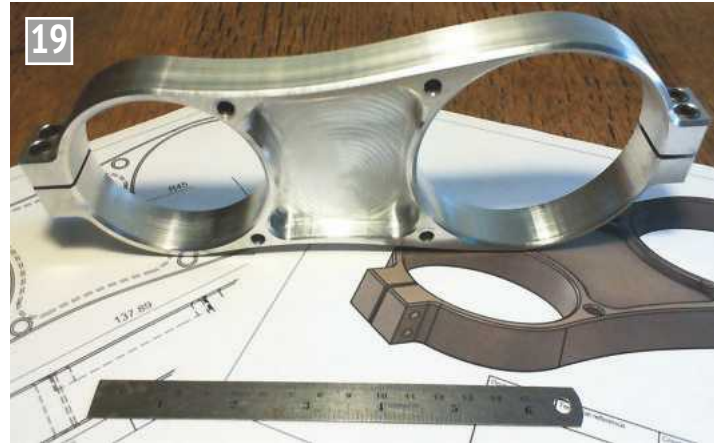
High speed spindle motor CNC machined yoke.
