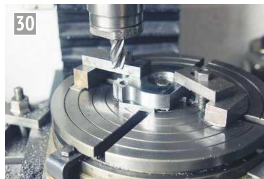
Machining the second stage of the outside of the flange.
