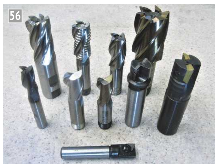
Milling cutters. Front row: Little Hogger single point carbide. Centre row, from left: three flute TiAlN coated, rounded edge, plain slot drill, 25mm diameter indexed. Indexed with TiN coating. Back row, from left: radius edge 25mm end mill, rougher standard 20mm end mill, plain end mill, 35mm end mill (£5 new on eBay!).
