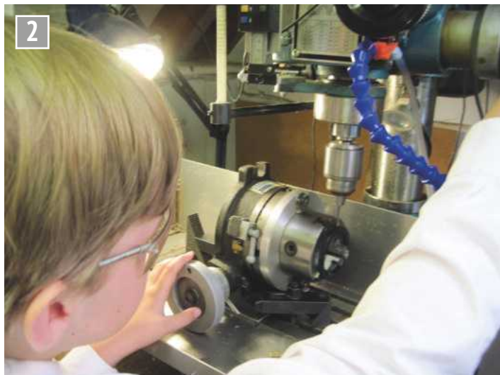
Rosie uses a dividing head to drill the holes for the spokes.
