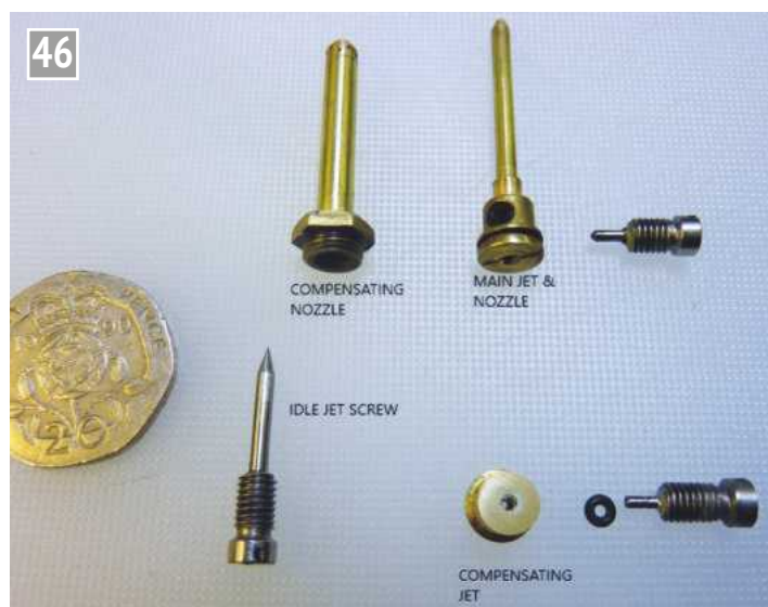
Nozzles, jets and screws. The 'cap' nozzle at the left fits over the main nozzle but both discharge through an array of tiny (0.3mm) holes to aid atomisation.
