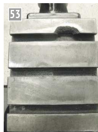
My distressed 'new' vertical slide showing why we need 'T' nuts!
