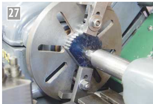
27 Plate located by the tailstock centre and clamped on to the faceplate.
