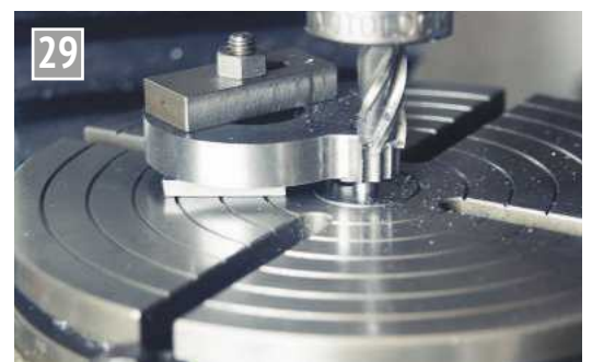
Machining the first section of the outside profile of the flange on the rotary table. The cutter is raised to allow photography.
