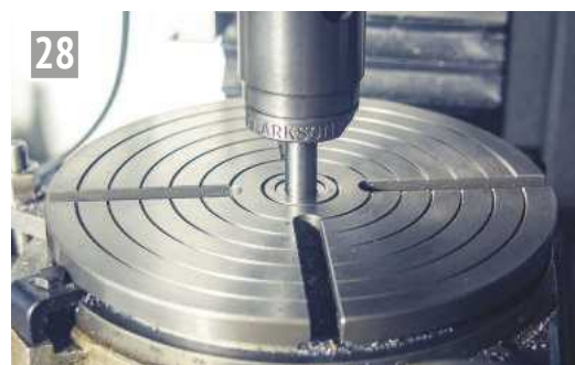
Using a plain silver steel probe in the autolock chuck to centralise the rotary table.
