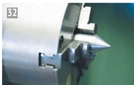
Turning a centre point on a stub of mild steel in the three-jaw chuck.
