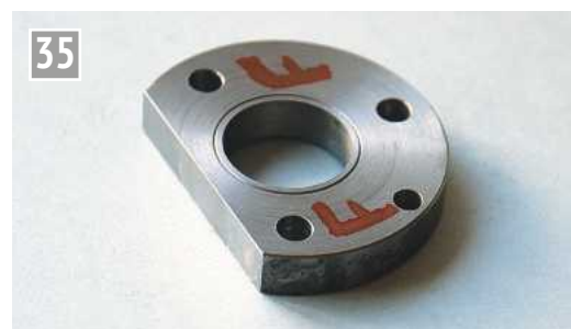
Transfer plate - made to transfer the fixing holes from the original shank to the new shank.
