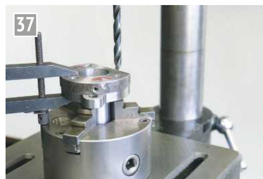
Jig drilling the new shank from the transfer plate. Note the 'F' (front) marks on top of the plate to give correct orientation.
