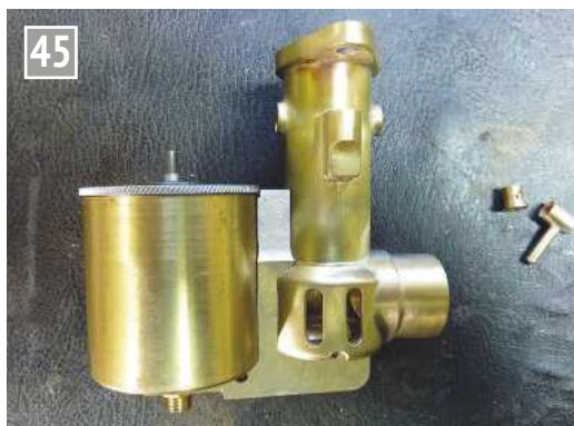
45 The carburettor assembled from the basic parts.
