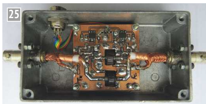
PCB (50mm x 50mm) complete with surface mount components.
