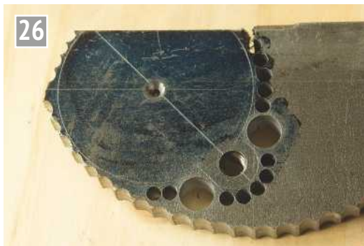
26 Plate for the flange, marked out and chain drilled on a piece of plate which had been chain drilled out of some other project.
