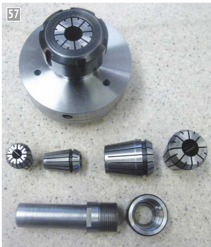
ER32 collet chuck for the lathe, home-made ER20 milling chuck in the front.
