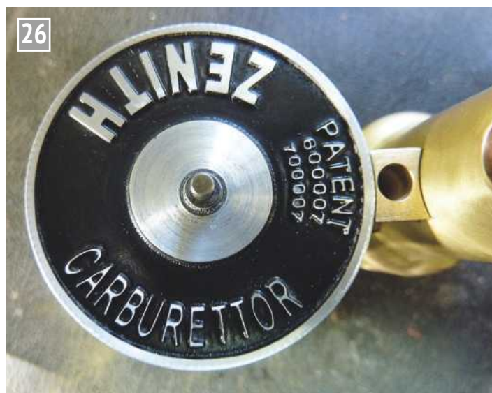
Reproduction half scale Zenith carburettor float chamber cover.
