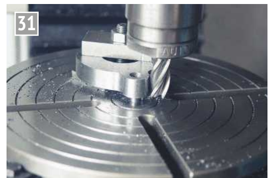
Work reset on a pin to locate in centre of the lug and exterior of lug machined.
