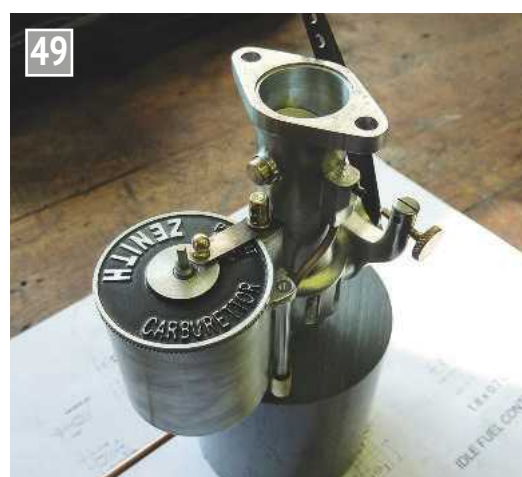
The bowl lid is secured by a leaf spring that can be slewed sideways.
