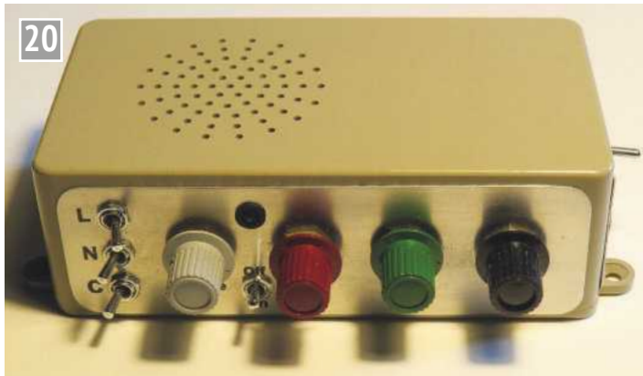
Morse tutor unit – case and front panel CNC drilled and engraved.
