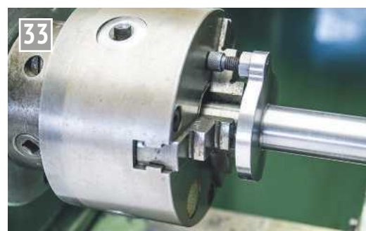
Cap head screw fitted into tapped hole in the plate being used as a driver whilst turning between centres.
