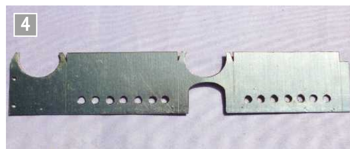
The case, drilled and ready for folding.
