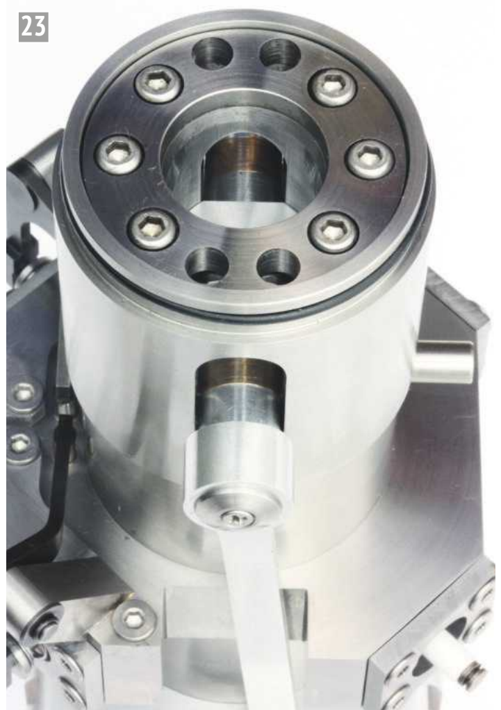
With the top cover plate removed the clamping arrangements become clear. The four bores are air passages which prevent the top cover being 'blown' off.
