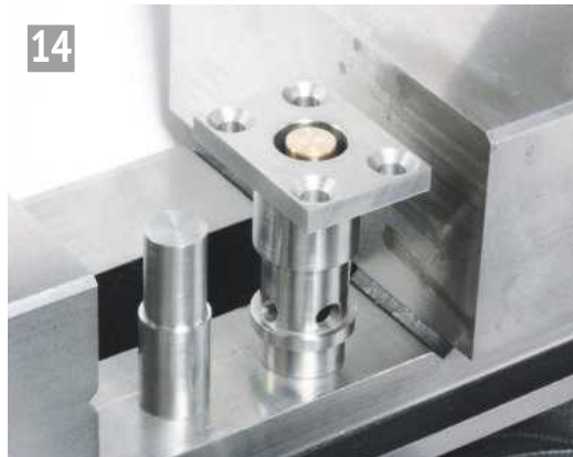
A bronze bush has been pressed into the valve inset from below but sufficient space remains in between to accommodate a valve spring.
