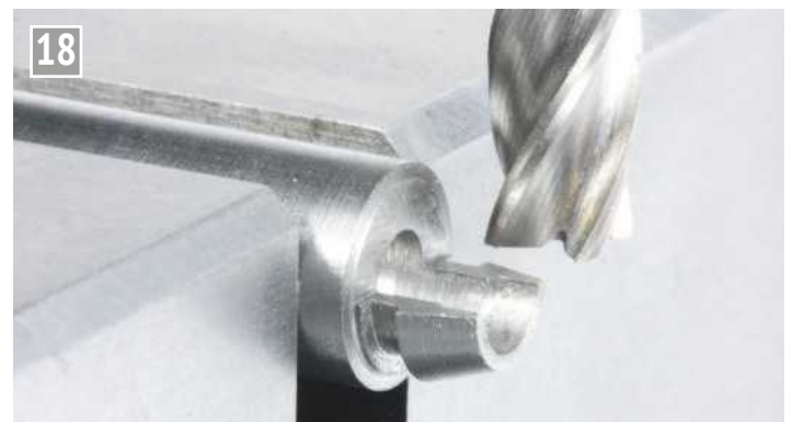
Four small wedges like this are required for the valve spring caps.
