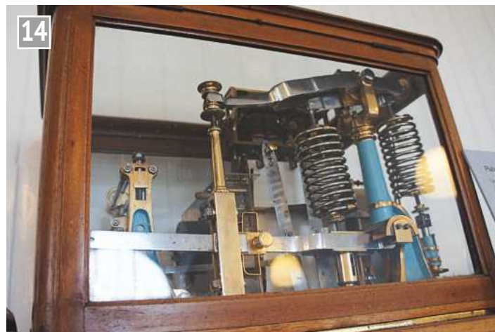
Pallograph measured vibrations. This came from John Brown's test tank when that closed in 1970.
