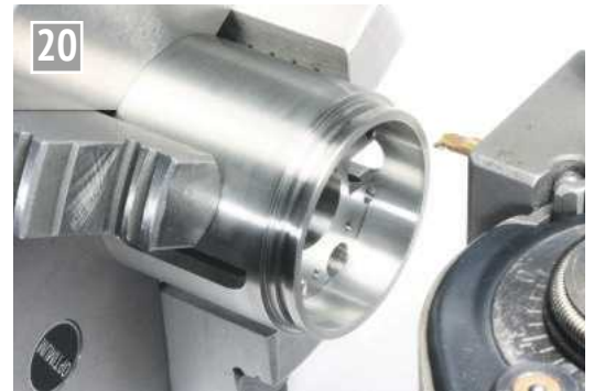
The rail case is still sufficiently solid to be chucked by three jaws.
