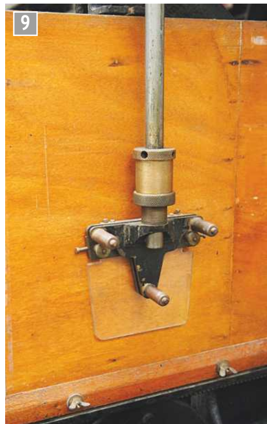
Tracer followed contour lines on plans so cutters would shape the model hull
