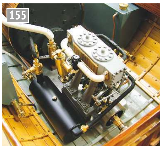
The finished installation. The exhaust lagging would later have a second layer of string applied - mainly for scale effect.
