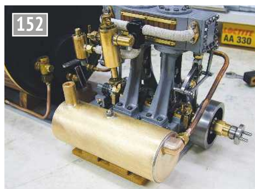
The oil separator tank worked well in use despite being horizontal as opposed to the usual vertical set up.
