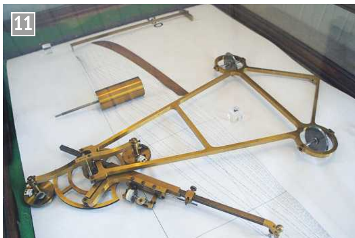
Integrator used to determine moments of area about a particular axis on a ship lines plan
