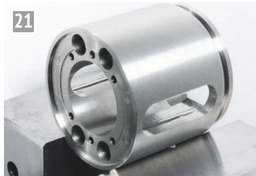
This is the finished sliding rail case with its four silver steel rails pushed in.
