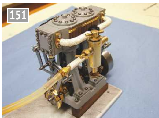
Ready to test - inlet side. The temporary copper wire to hold linkage pins was later replaced with split pins.
