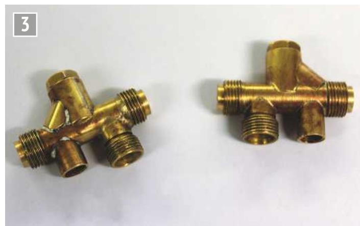
Finished injectors looking for a home.
