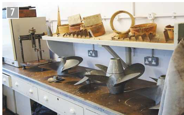
Denny's tested hundreds of propeller designs. Each took a skilled technician a week to make.
