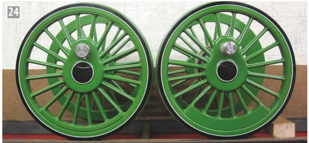
Completed wheel sets.
