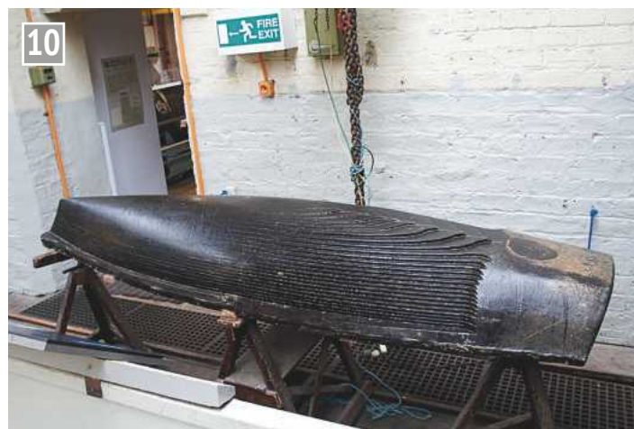
Contoured hull after cutting, partly smoothed off.
