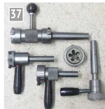
Four tailstock die holders; the three in the front are used most.
