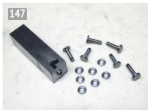
The simple drill jig for cross drilling the linkage pins.
