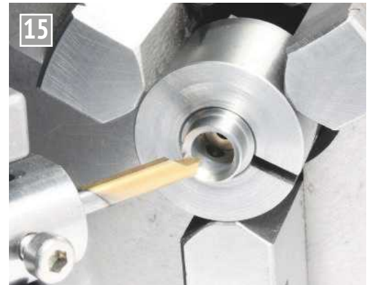
The valve guide bore is already reamed and the seat has just been turned.
