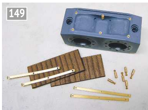
The lagging and method of fixing - much safer than tapping the casting directly.
