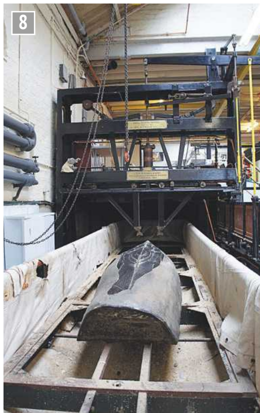
Machine to cut hull forms, designed for wood cutting it then cut wax models. Revolving cutters hang below.
