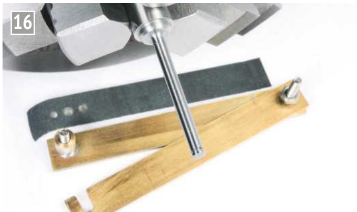
This is my lapping equipment: abrasive paper (up to 1000-grit) on one side, brass on the other side – and plenty of cutting oil.
