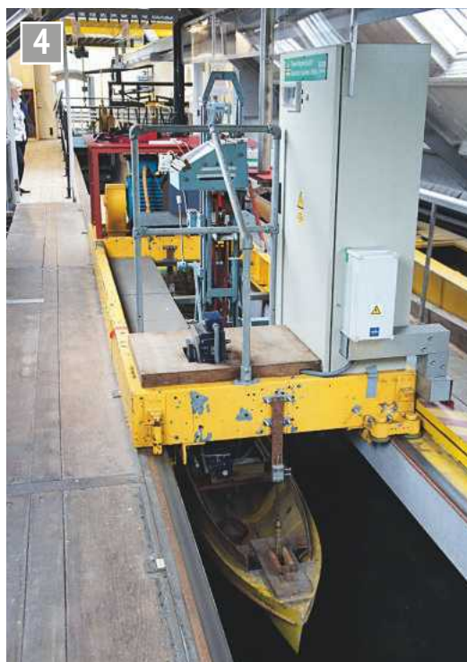
Instrumentation panel with hull model below (not normally accessible).
