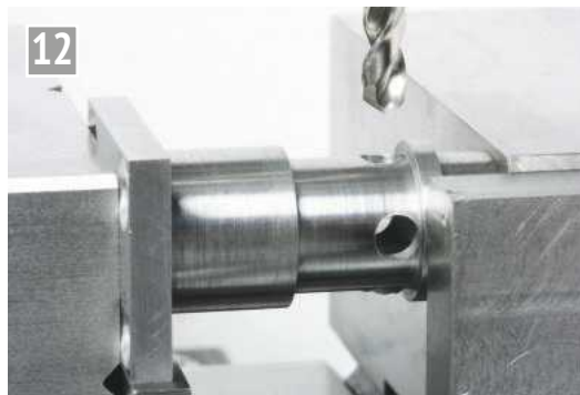
A valve inset has just been equipped with the inlet/outlet bores.
