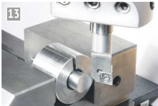
The high compression blind-plug fits the inner cylinder radius.
