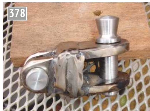
The towing eye and pins, after welding up.
