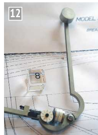
Planimeter used to determine areas enclosed by any shape.
