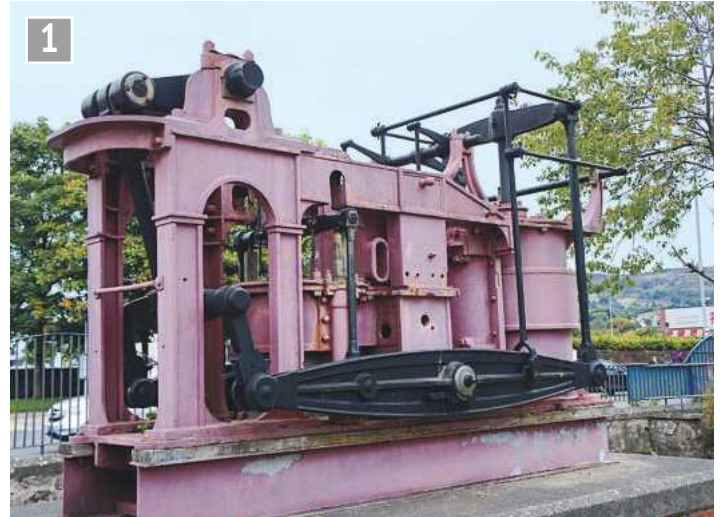
1 Believed to be the world's third oldest marine engine. Built by Robert Napier in 1824, his first marine steam engine, fitted in the paddle steamer Leven. Single cylinder side lever type of 30 horsepower.
