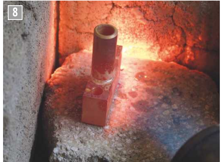
The solder after flowing.
