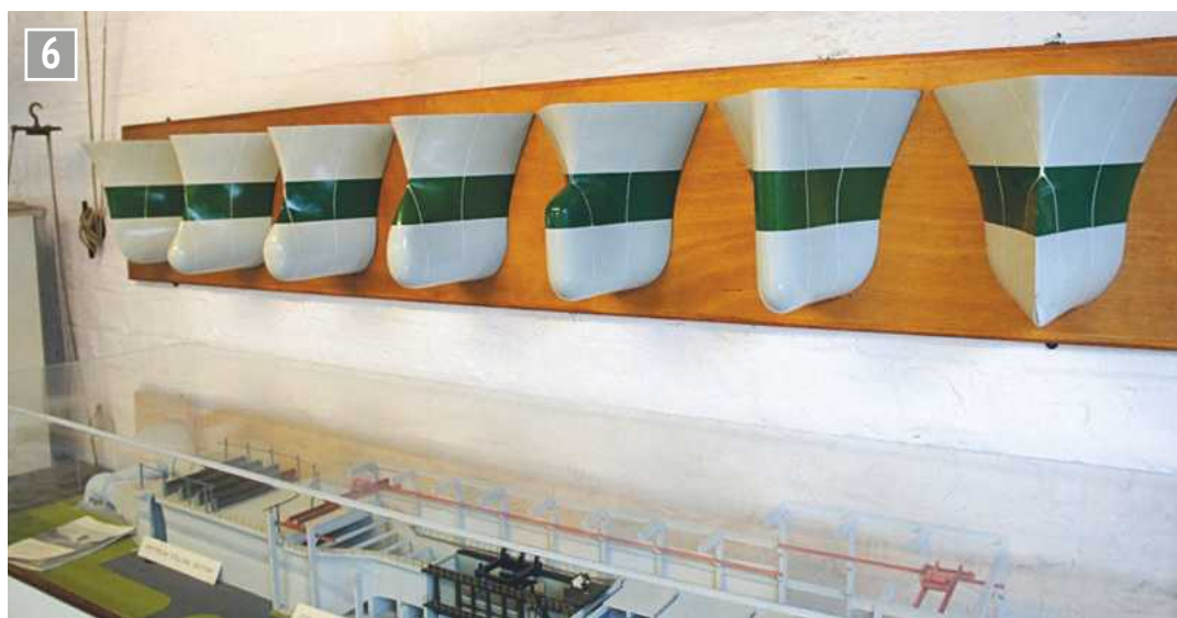
Bulbous bows developed through tank testing. Models show some types tested.
