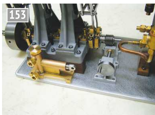
The small fabricated water pump and drive set up.
