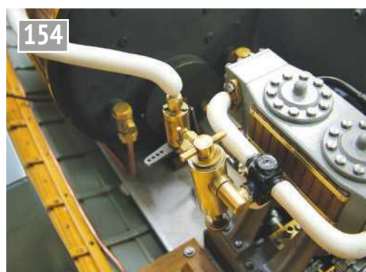
The epoxy covering on the lagging stood up well to the first steaming although exhibiting minor cracking in places.
