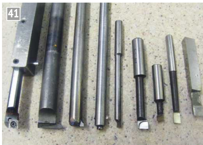
Boring tools, left to right: inserted bit in my tool holder, brazed small square bit for screw cutting, 10mm pocket cutting, 6mm through bar, silver steel 6mm shank, 3/8 inch carbide tipped (not now used), two small preformed bars, the one we will make.
