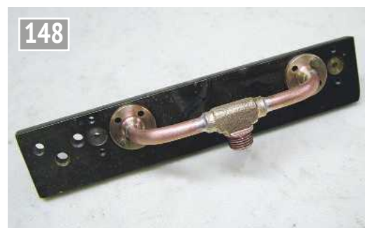
The jig for soldering the flanges in place. Holes to each side of the flanges are for the inlet. The other three holes are from a previous use.
