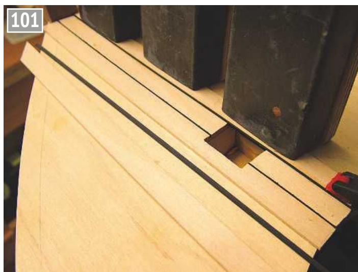
Showing the Bass wood planking and thick card 'caulking'.
