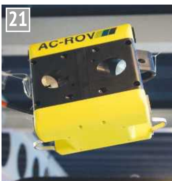
21 This mini ROV could be used for various applications including pipeline checking. Aberdeen companies lead the word in this type of technology.
