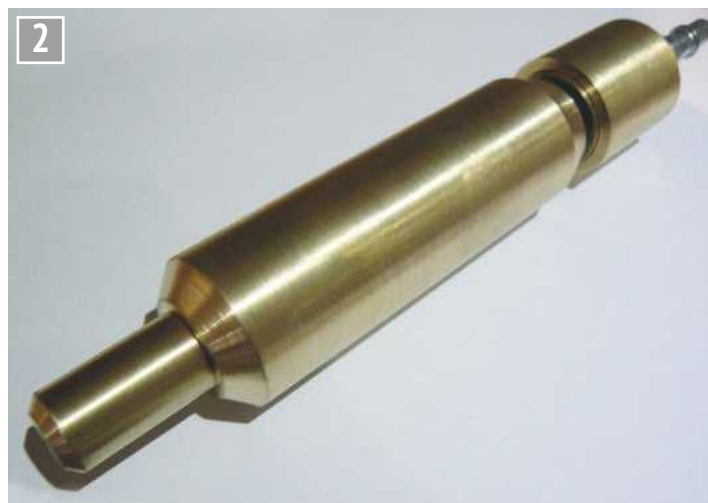
Completed steam whistle after testing on compressed air.
