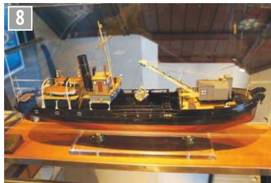
Grab dredger built for Aberdeen's harbour commissioners - it could work close to harbour walls.
