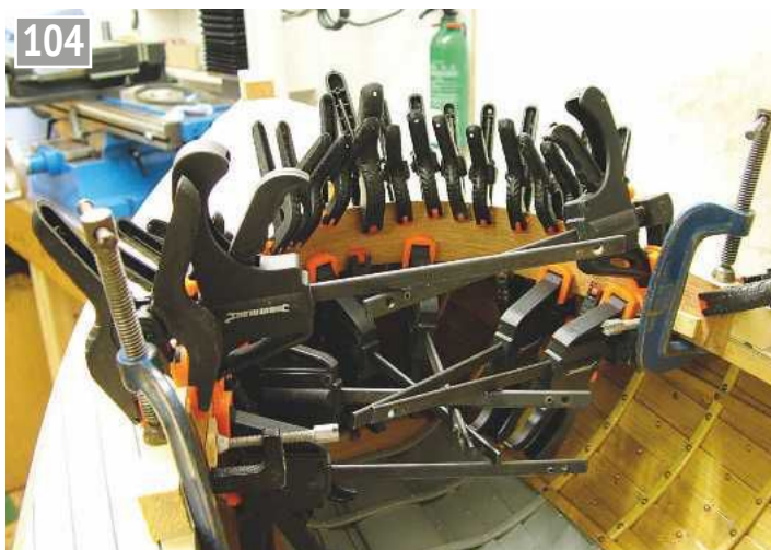
104 Laminating the forward coaming from three layers of mahogany sheet. As elsewhere there are never enough clamps at times.
