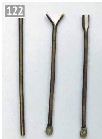
Forming the ends of the struts.
