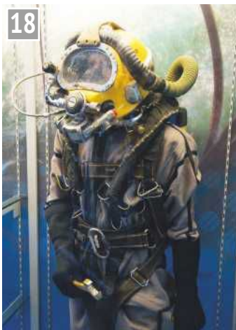
18 Sub-aqua diving suit as used in the North Sea; if working at any depth divers needed to decompress to avoid the 'bends'.
