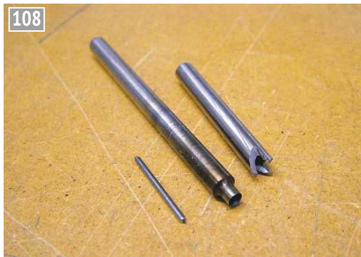
108 The simple cutters made to create small plugs – the plug cutter was left unhardened.
