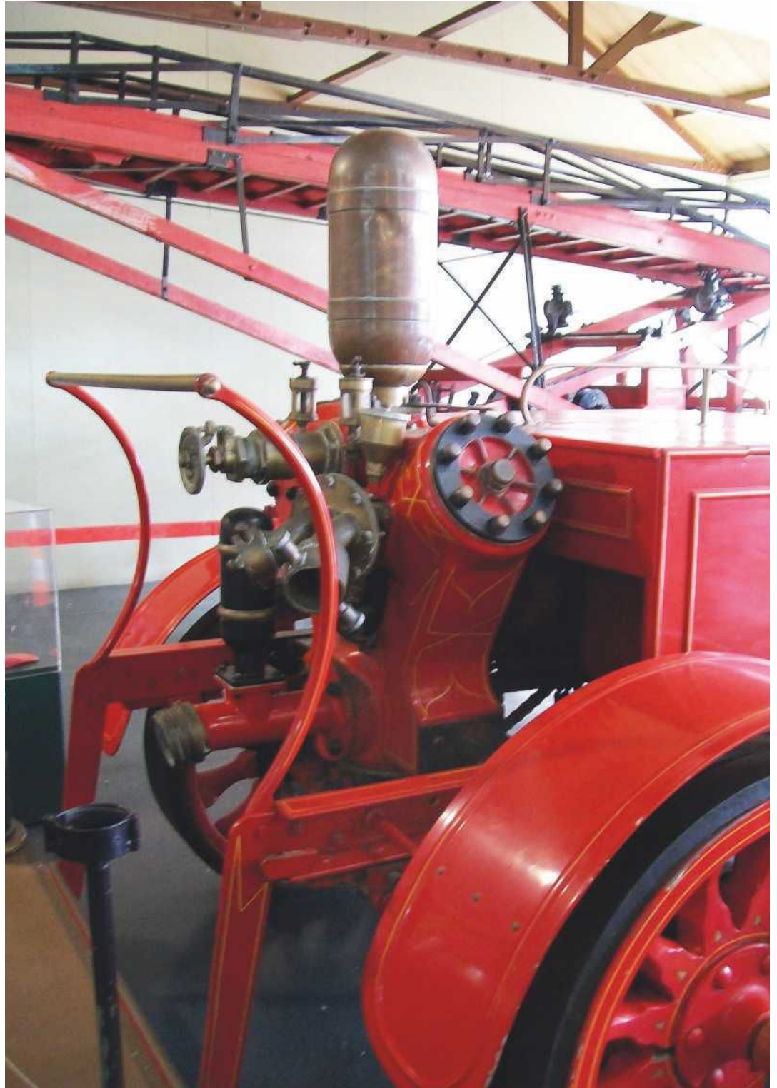
Hatfield pump on Merryweather fire engine of 1907-08 in the Museum of Technology and Transport, Auckland New Zealand. It could pump up to 250 gallons per minute. © Lisa Truttman 2012 and reproduced by permission.
