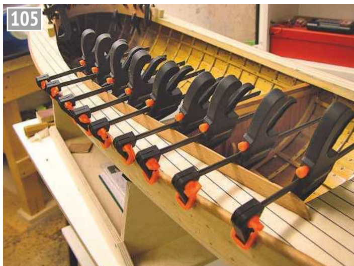
105 Laminating the side coaming from two layers – more clamps!
