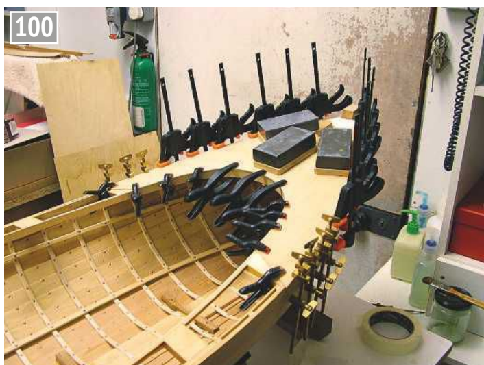
Attaching the 1.5mm ply sub fore-deck.
