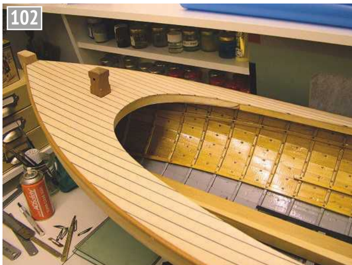
102 Finished planking after much sanding, scraping and more sanding!
