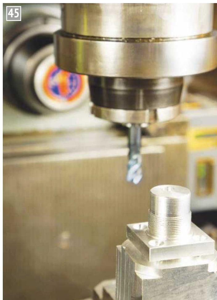
Milling and drilling the flange.
