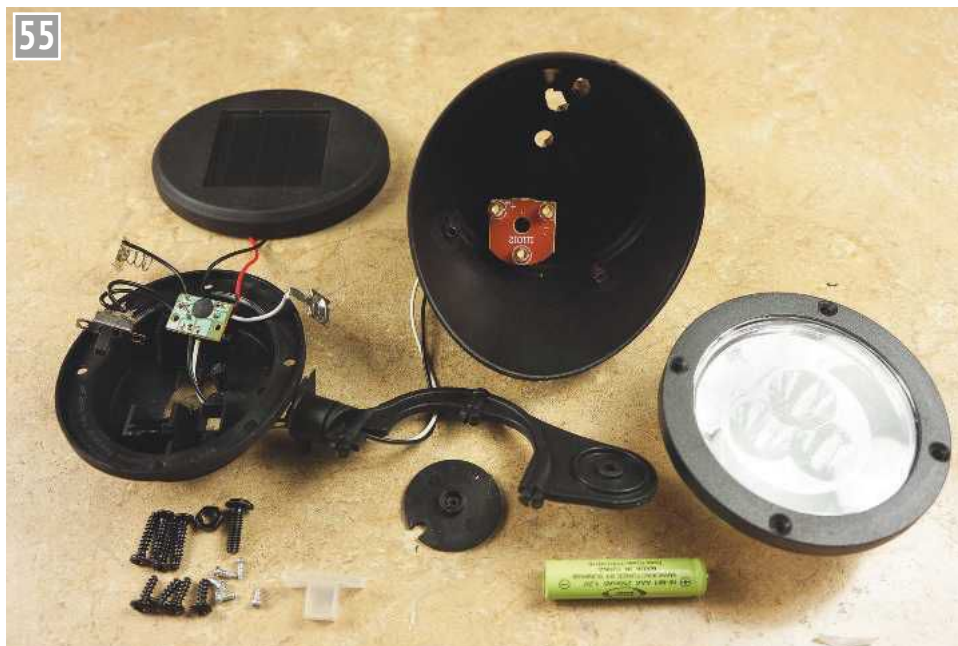
Dismantled solar light.
