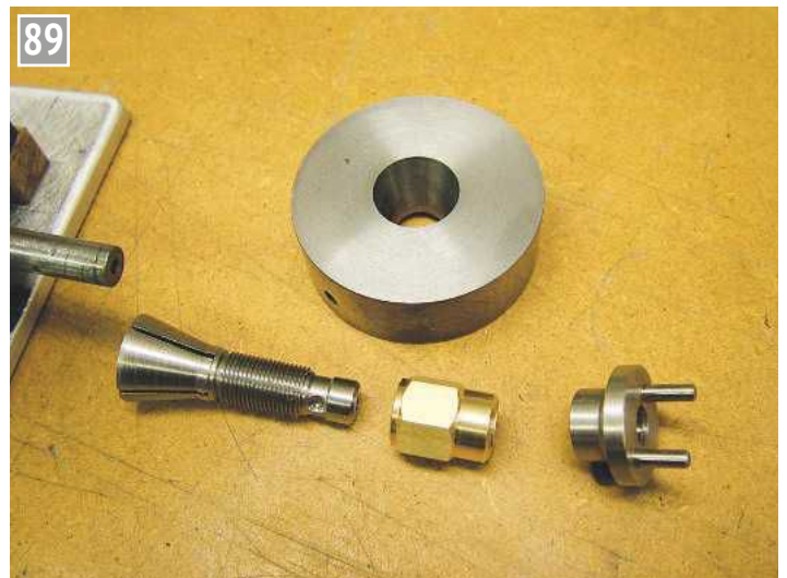
The parts for the collet type flywheel drive and coupling.
