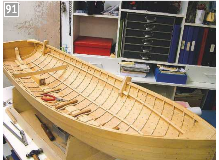
Fitting the stringers and the final riveting.
