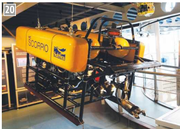
20 The Scorpio Remote Operated Vehicle (ROV) was for underwater inspection with an arm to manipulate items.
