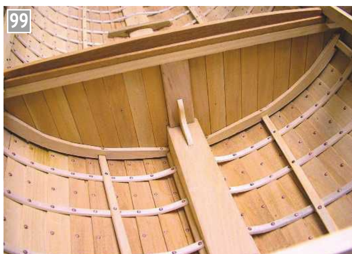
Aft bulkhead from the aft cockpit side showing the fixing ribs clear of the planking.
