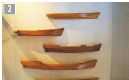
2 Half hull models used to design wooden ships. Designs were scaled up in the mould loft. Early shipwrights rarely used drawings.
