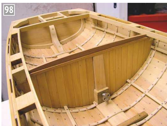
The aft bulkhead from the engine side.
