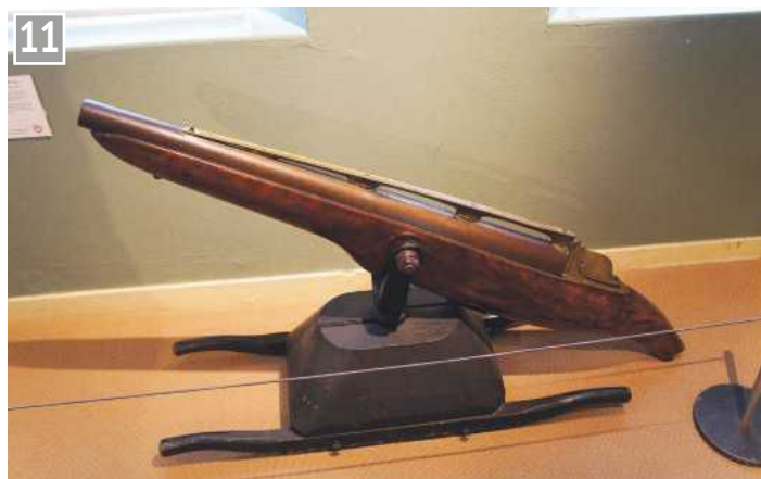
11 Harpoon gun used for lifesaving - it fired a line to a stricken ship.
