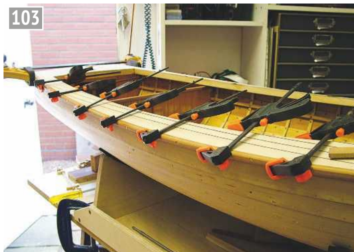
103 Fitting the mahogany rubbing strake, 10 BA countersunk brass screws were used for scale head effect.
