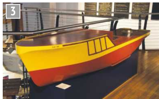
3 Model of the Lady Rosemary hull tested in the Denny Test Tank at Dumbarton. This was an oil supply vessel launched in 1973.
