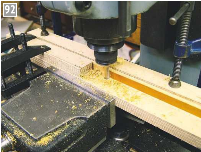
Home-made 'thicknesser' at work.
