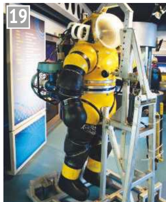
19 NEWT suit invented by Phil Nuyttens and also used in the North Sea. It is made of cast aluminium and the diver controlled it by propellers. This obviated the need for decompression.
