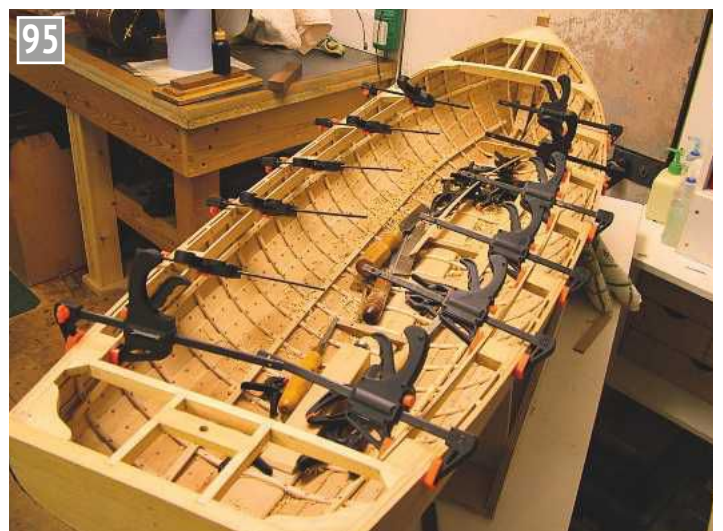
Fitting the inner coaming boards.
