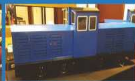
"Imp" £1650 4x motors 4x batteries 100A controller
