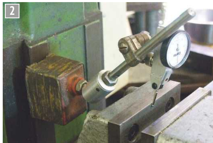
Setting the vice fixed jaw so it runs parallel to the X axis.
