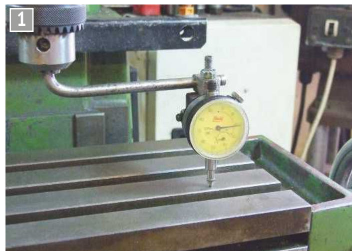
Checking the milling spindle is truly vertical to the table.
