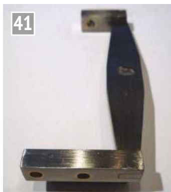
The valve actuator bar with levers attached.
