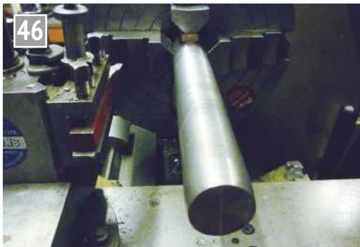
Offsetting the bar for the crankshaft.
