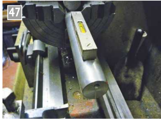
The centre for the main axis of the crankshaft.
