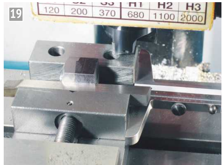
Cutting the head of the hammer using the milling machine.
