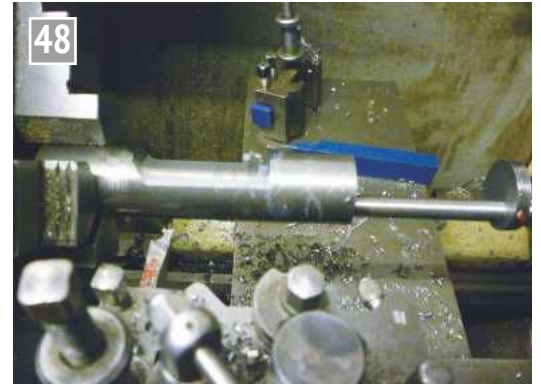
Turning the second half of the main axis.v
