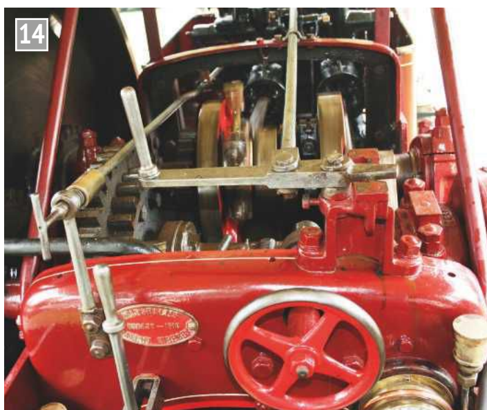
14 A three speed engine - the three speeds are accessed via the round hand wheel. Two of the three speeds may be seen in the left of the picture and the third is in shadow inside the flywheel rim.
