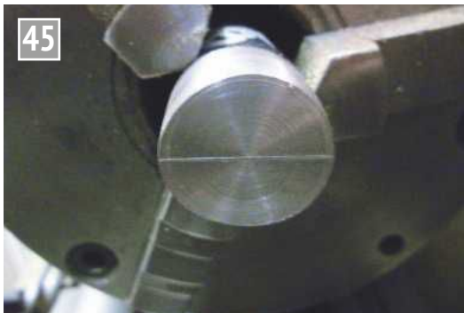
Marking the end of the bar for the alternative crankshaft.
