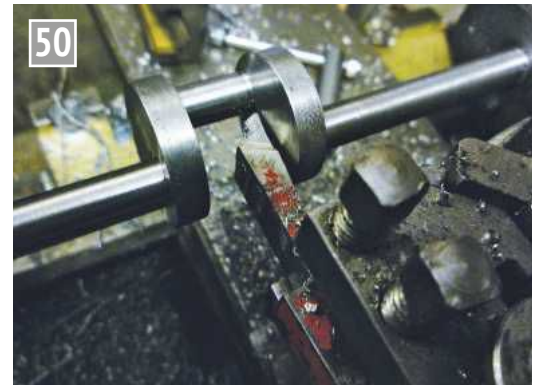
Turning the journal on the crankshaft.
