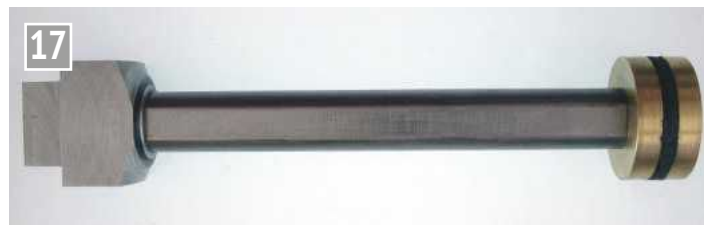
Hammer, rod and piston assembly. Note that the flat on the rod is parallel with the side of the hammer.
