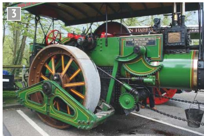
Detail of the Ratty scarifier - the tines are not fitted.
