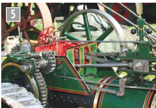
Note the model, like the full size, has split horn plates and a four-spline crankshaft.
