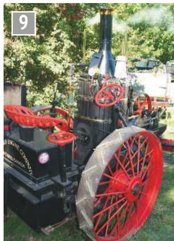
The prototype had a coal/wood box on the back but for practical reasons in model form a driver's seat has been substituted.
