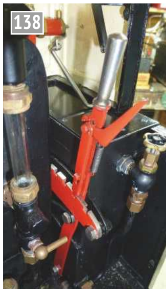
Cab view of reversing lever and quadrant.
