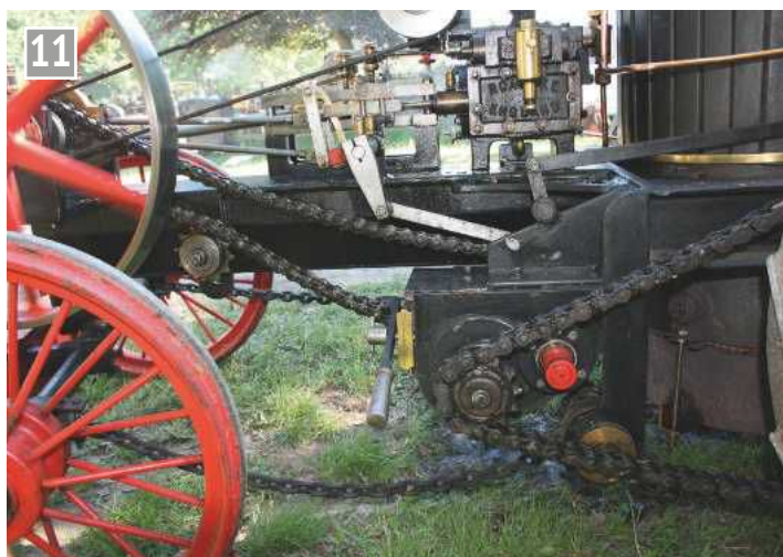
11 The drive train on the Fireproof Champion. The crank shaft, top left, drives by chain a two speed gearbox and thence by another chain the back wheels.
