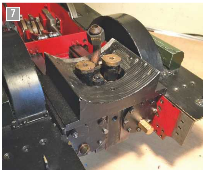
The two new blastpipe uprights shown in place.
