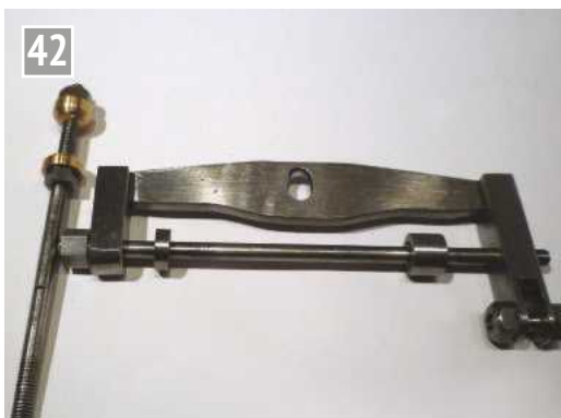
The support bar is now added to the actuator lever.
