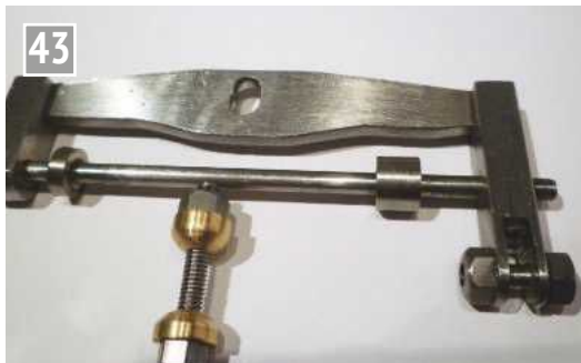
The valve bobbins mounted on the valve rod.
