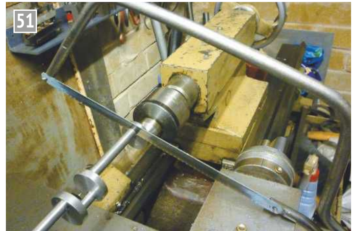
Parting the crankshaft from the unwanted stock.
