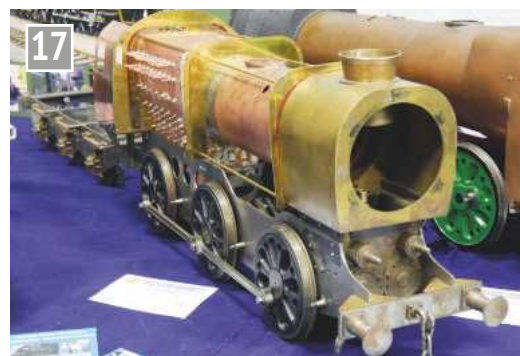
17 A part built 5 inch gauge Q1 class 0-6-0 goods locomotive built by the late Gerald Chandler and now owned by William Powell, who has set about completing the model.
