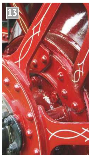
13 The wheel spokes are riveted to the both the hubs and rims, avoiding any risk of cast in spokes working loose.
