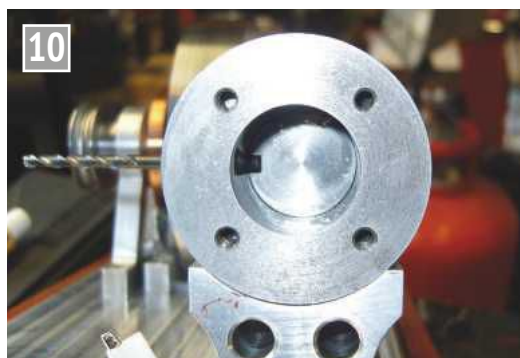
Using a drill to line up the ports with the cutouts.
