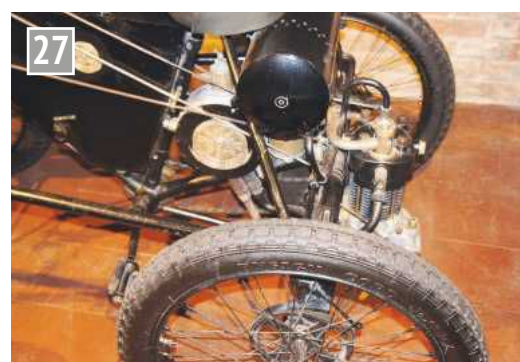
De Dion Quadricycle built 1899 detail of rear drive.
