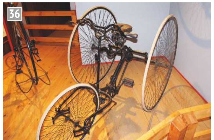
Quadrant tricycle made in Birmingham around 1885. It has a differential gear.
