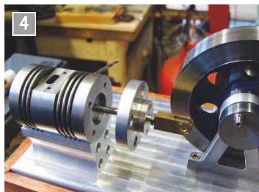
Cylinder bottom cover and piston rod seal.
