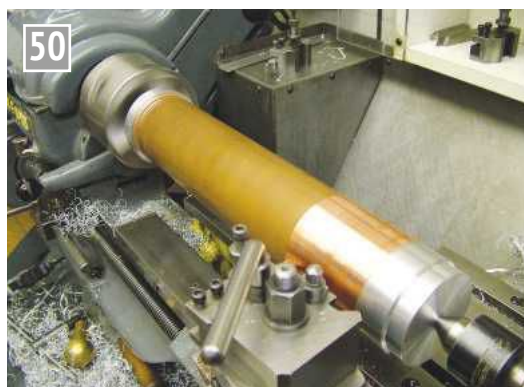
Reducing the 10swg tube to 12swg,
