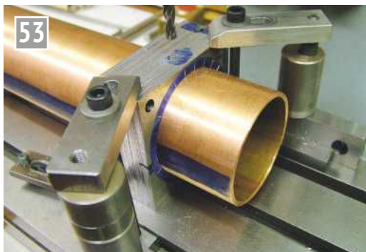
Drilling the first hole – the system worked better than anticipated.
