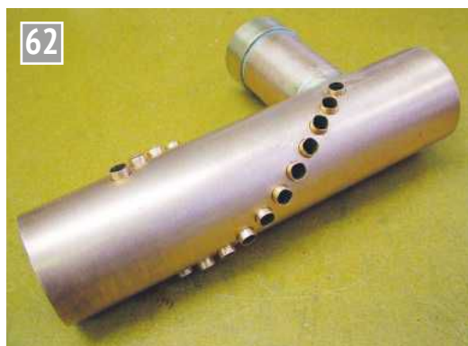
Second ends swaged and ready for soldering.
