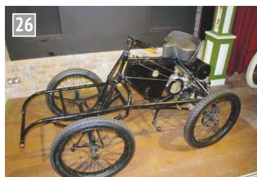
De Dion Quadricycle built 1899, derived from a motor tricycle. This now lacks a front seat.
