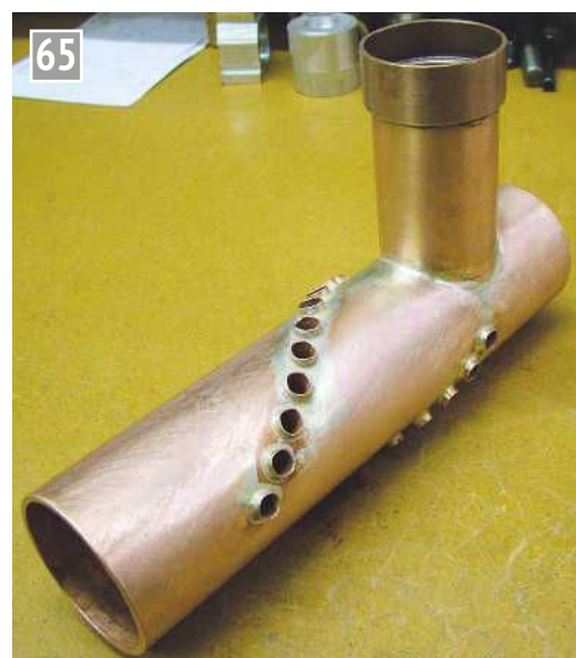
The finished flue, cleaned up and ready for inspection.
