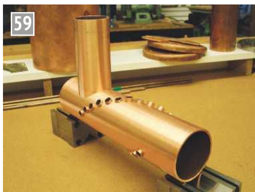
A dry run before final assembly for soldering.
