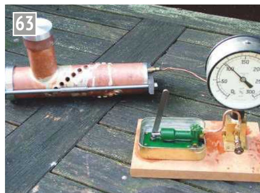
Pressure testing to check for leaking solder joints - none this time.
