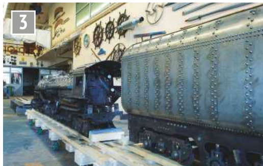
The original coal tender of the Big Boy locomotives were 14.4 metres long and weighed some 155 tonnes (342,200 lbs) when loaded.
