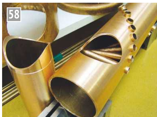
The end of the uptake was reduced to fit and to allow it to sit at the right depth.
