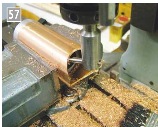
Using a boring head to shape the uptake tube – note the insert to prevent crushing.
