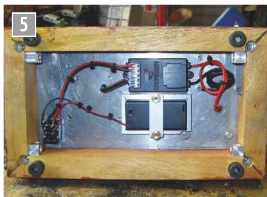
The electronic ignition system installed neatly under the baseplate.
