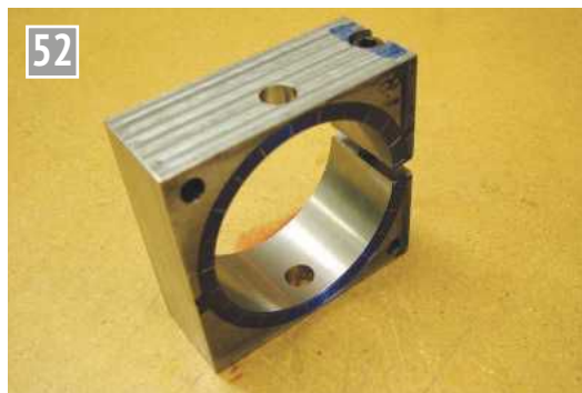
The clamping fixture/drilling jig. Doubling the number of divisions allowed the opposite scribed line to be used as the other 'disappeared' beneath.
