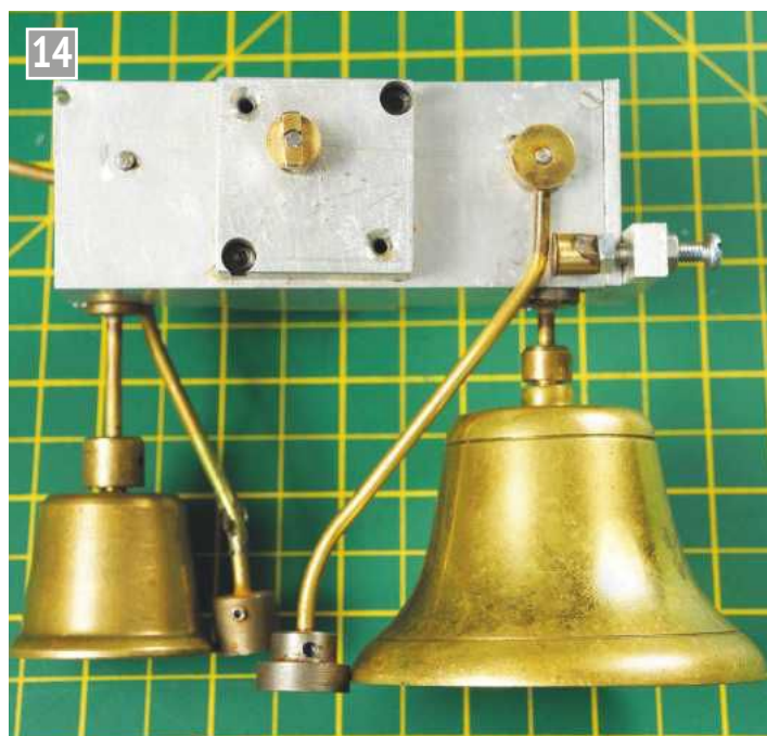
Modified bell-striking mechanism.
