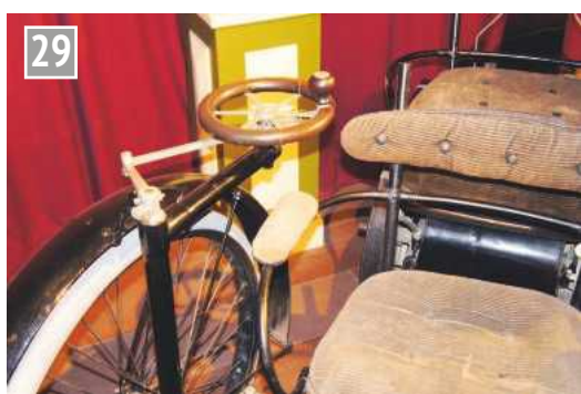
Coventry Motette detail - small hand wheel to steer.
