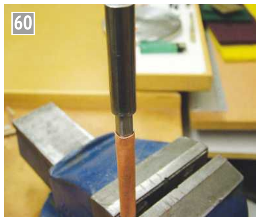
Swaging the first end of the water tubes. The tube sits over a steel mandrel that controls the depth of the swage.
