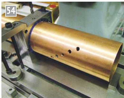
Showing the moveable 'fixed' stop – reset after each hole.
