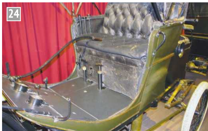
LEFT: White Stanhope steam car retained tiller steering. RIGHT: Cleveland battery-electric car built in the USA 1901. Electric cars did not need crank starting and were popular before the invention of self-starters. Electric cars even held the land speed record briefly.
