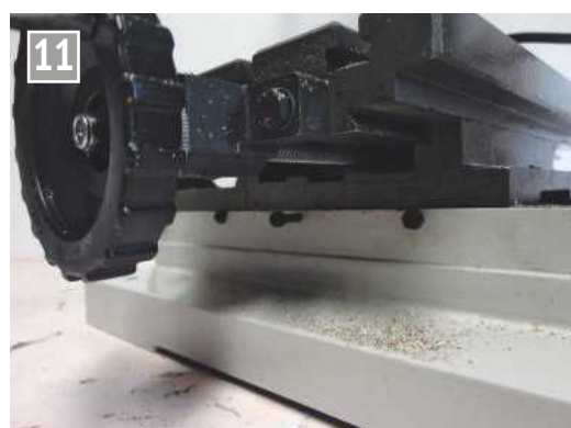
The slide clamps are simply M5 screws.
