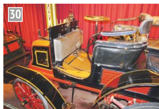
Panhard et Levassor car of 1899. Emile Levassor pioneered the engine in front plus clutch and gear box in line.
