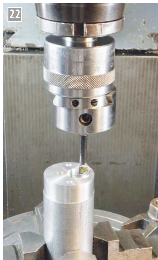
Boring the bearing location.
