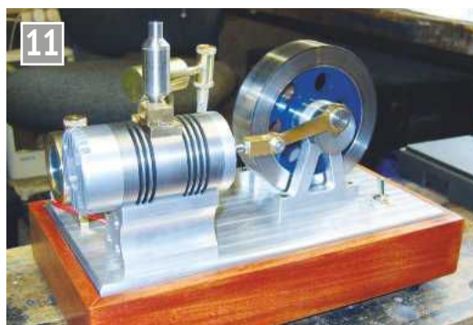
A view of the engine showing the new, finned cylinder head.
