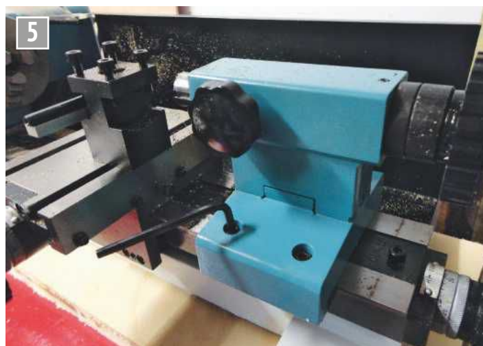
The tailstock is locked to the bed using two M5 screws.
