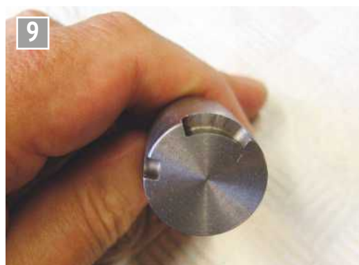
End-on view of the new piston, showing the inlet and exhaust cutouts.
