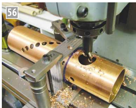
Boring out for the uptake tube.
