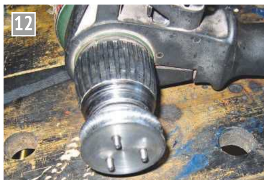
Three pins engage the engine pulley for starting.
