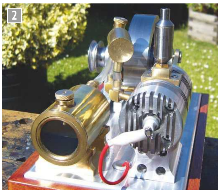
The view from the back end, showing the transparent fuel tank end and spark plug.
