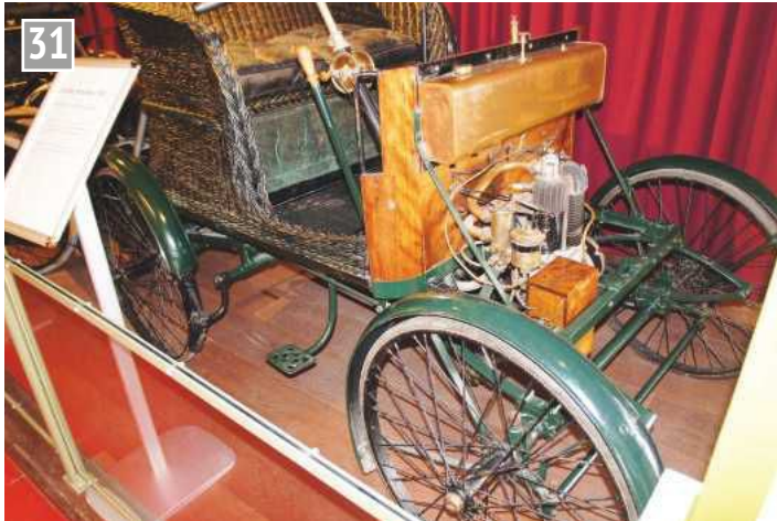
Unique Sturmev voiturette of 1900 with a De Dion engine. Built to test a prototype hub gear later used as the Sturmev-Archer bicycle hub gear.
