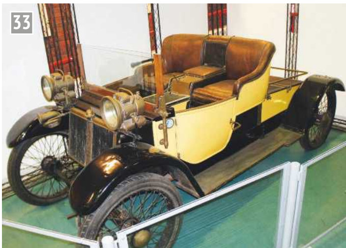
Lanchester open tourer of 1907-08 . Frederick Lanchester was ahead of his time as an automotive engineer. He pioneered the chassis and engine as one unit.
