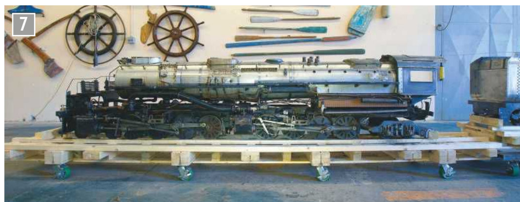
The 1:8 scale model measures 5,05 metres overall in length, 3.25 metres of which is the locomotive, 1.80 metres the tender.
