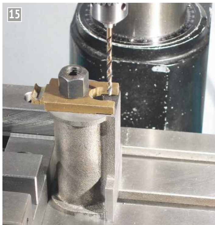
Drilling the steam passages.
