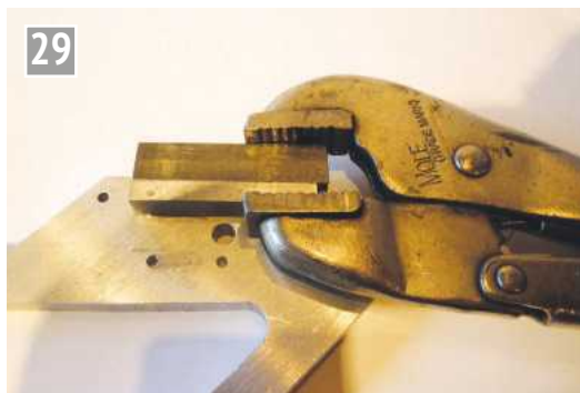
Clamping the upper slide bar into place for spotting through the holes.
