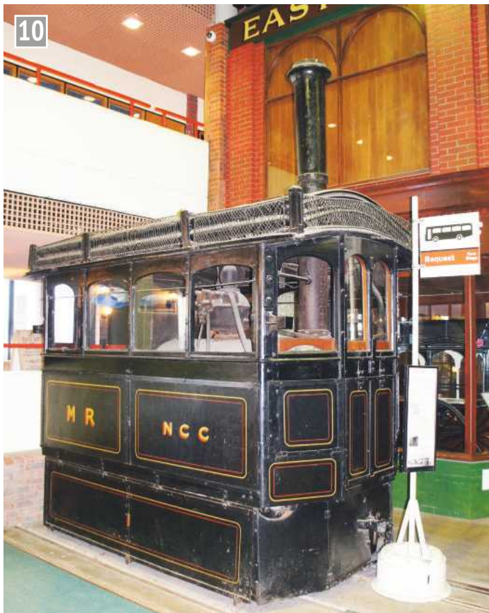
Kitson steam tram, Leeds, built in 1882 for the 3 foot gauge Portstewart Tramway in Northern Ireland. Later controlled by the Northern Counties Committee of the Midland Railway.
