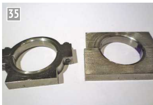
The eccentric strap is cut out and filed to shape.
