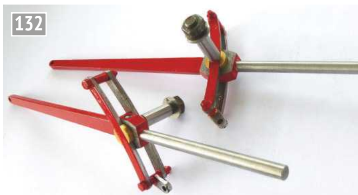
Expansion link and die block on the rebuild.
