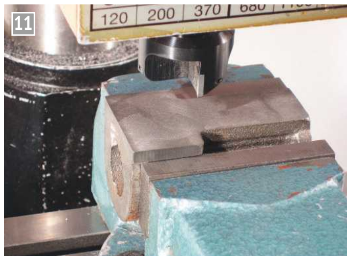
Milling the bolting face of the cylinder.
