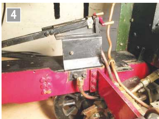
A new reversing screw is required to make use of the increased die block movement.
