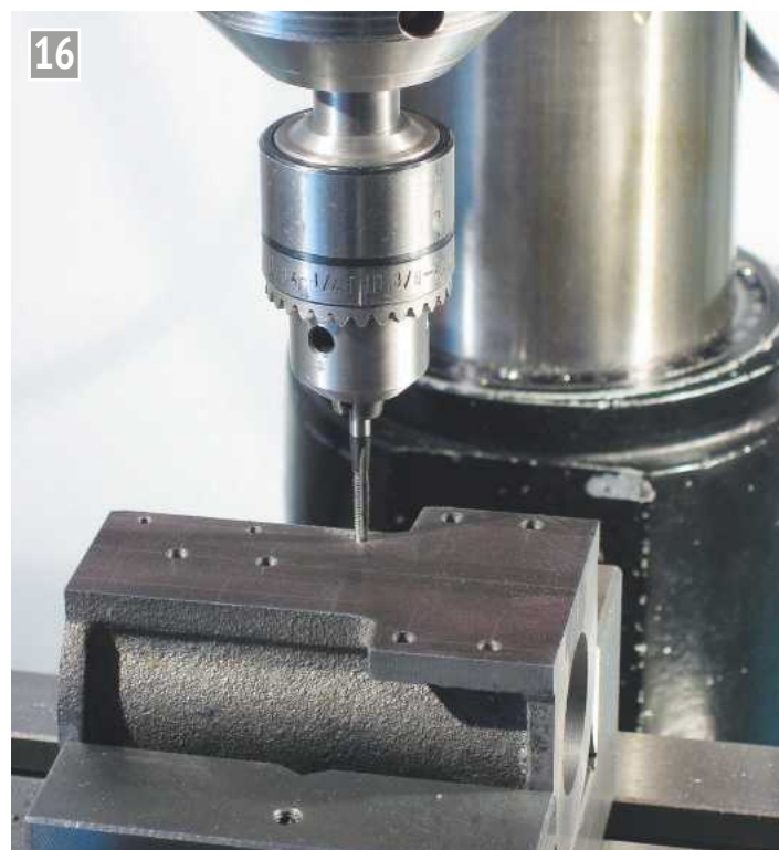
Tapping the screw holes in the bolting face.
