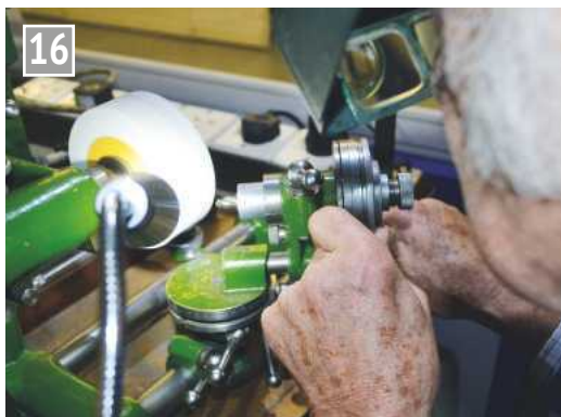
DAG Brown demonstrates precision drill sharpening on his Quorn tool grinder.
