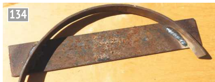
Expansion link guide plate forging jig.
