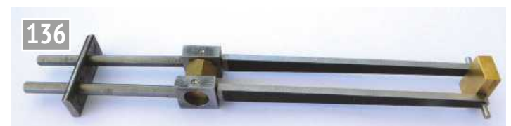
Set-up for silver soldering the radius rods.
