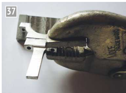
Spotting through onto the strap.
