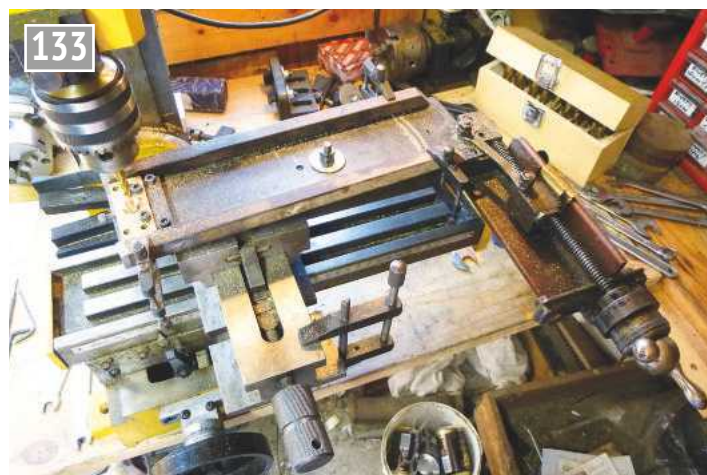
Milling the die blocks.
