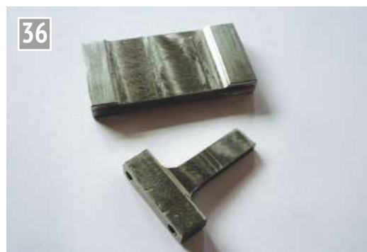
Forming the eccentric rod end.
