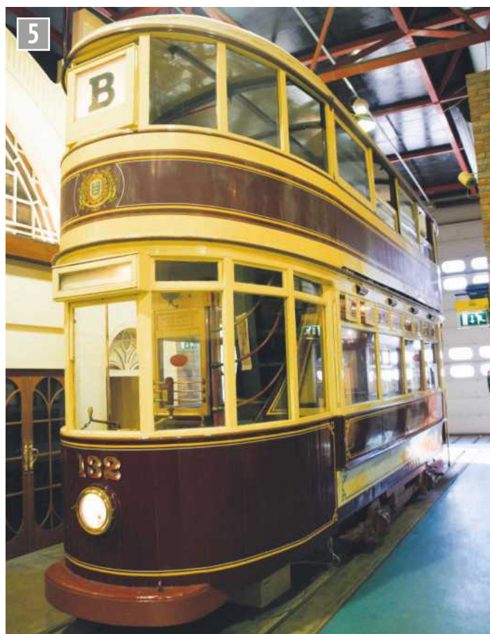
Later four-wheel tramcar of a type made in 1910 that operated until system closure in 1945. Some were then sold to Leeds.
