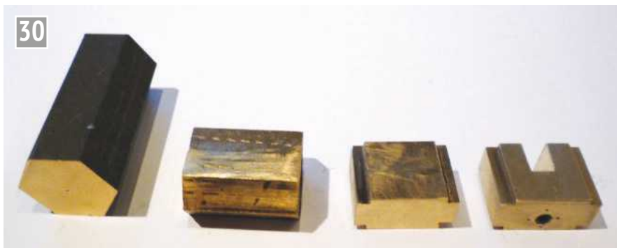
Stages in forming the crosshead.
