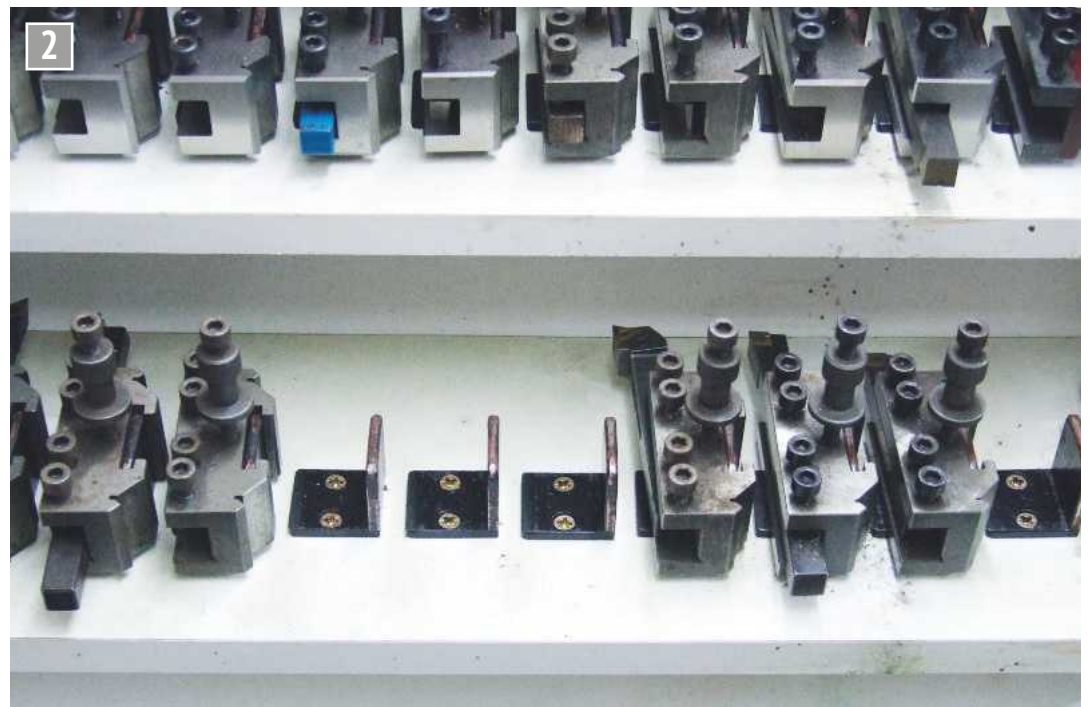
Four tools removed to show the tool support brackets.
