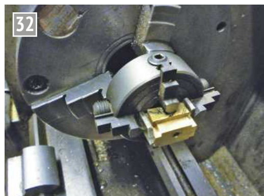
Crosshead held in a 'piggyback' chuck.
