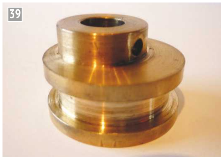
Finished eccentric sheave.
