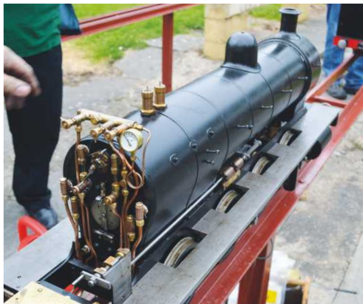
Ben's Netta has been loaded with plenty of weight so adhesion should never be a problem. These platforms are actually made of 12mm steel plate with the edge machined to look like a valance. They weigh in at 20lbs each, contributing to a total locomotive weight of about 200lb.
