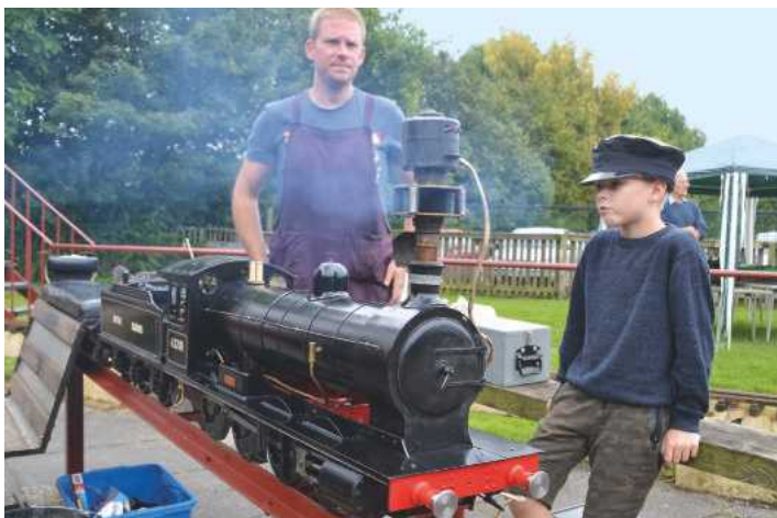
Another 5 inch gauge Netta was brought along by the Tompkins family; Dave, nephew Paul (official driver) and Paul's son Ollie (assistant driver). Like Ben's Netta, the Tompkins Netta has oversized cylinders, in this case 1½ inch diameter, machined from a block of Meehanite (a fine grade of cast iron). The tender is fabricated in aluminium sheet 'borrowed' from defunct printing machinery. The locomotive has two injectors but no hand pump or axle pump and is fitted with PTFE piston rings and two radiant superheaters. She was completed in 2003 and is a frequent runner at IMLEC.
