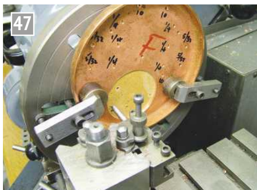
Boring one of the plates to take the flue tube.
