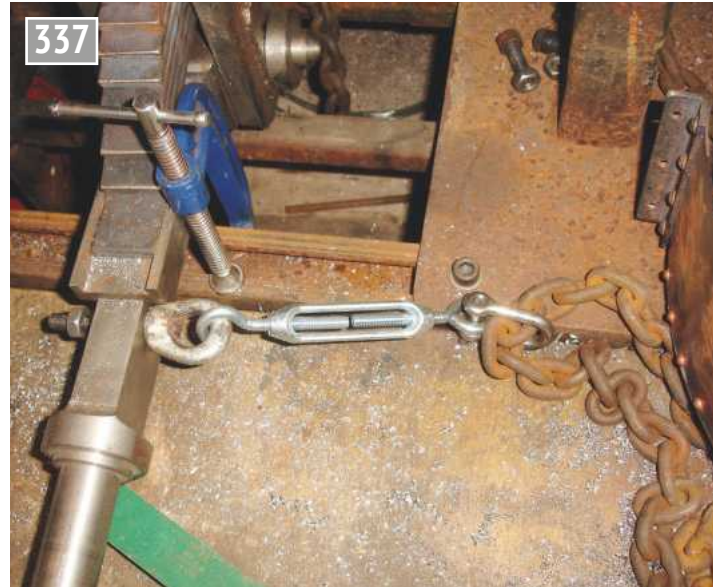
Left hand connection and turnbuckle.
