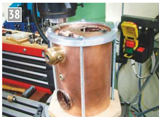
Cautious plunge milling took a while but was carried out without any hitches.
