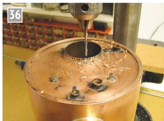
Chain drilling around to release the flue.
