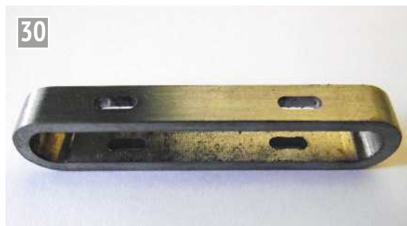
Connecting rod straps before separating into two.
