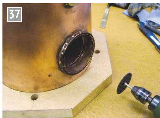
Cutting the flue inside the main shell.
