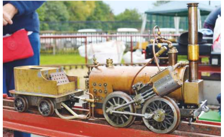
William also brought along his 3½ inch gauge Canterbury Lamb. Of note are the variegated wheels and the rosebud grate, which may be seen resting in the tender. The cylinders are comparatively big and I wondered whether the boiler would keep up with them. Evidently though, it does and the locomotive is, as the estate agents might say, deceptively strong. She was steamed up only at the end of the day for a brief run.
