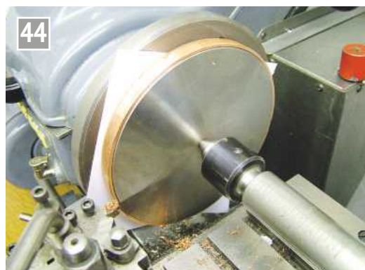
Turning the outer diameter to an easy fit in the barrel.
