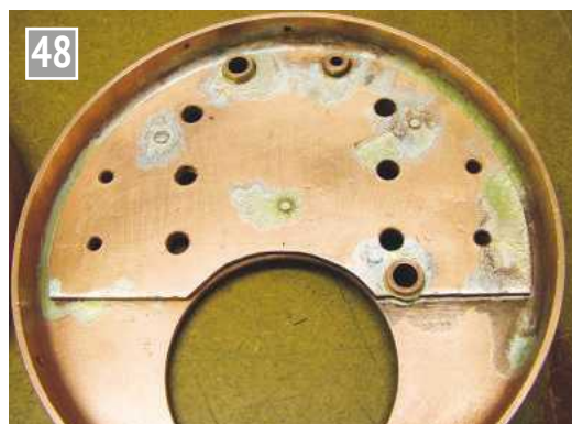
The inner strengthening plate note the deep chamfers for the solder to form good fillets.
