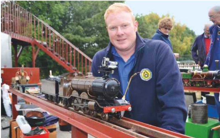
William Powell brought along two locomotives, including this version of Ayesha, named Freya, and finished in LBSC livery. This locomotive won the Curly Bowl competition last year. It was bought originally as a 'bag of bits', most of which had to be reworked, and is fitted with an 'Ayesha II' boiler.
