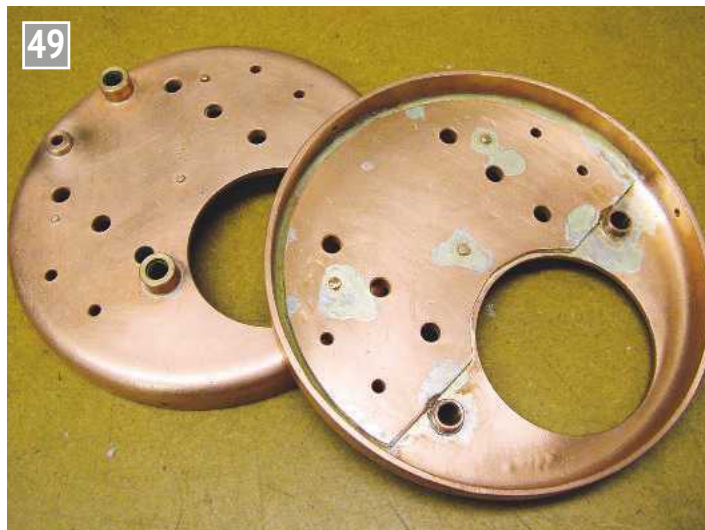
Finished end plates ready to fit note the three holes in the flange for the locating rivets.
