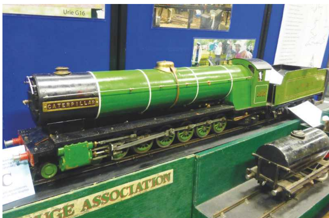
Another LBSC locomotive, Caterpillar, an unusual 2-12-2. This was reputedly based on a Union Pacific 9000 class and it was offered with three or four cylinders. It was published in English Mechanics in 1932.
