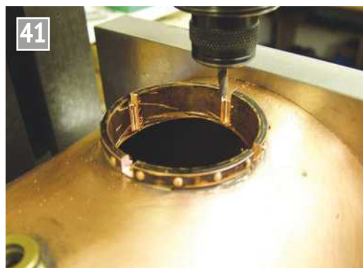
Plunge milling to cut away the flue outlet.
