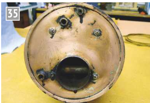
The manner of fitting the original end plates - 10swg copper with a reinforcing band.
