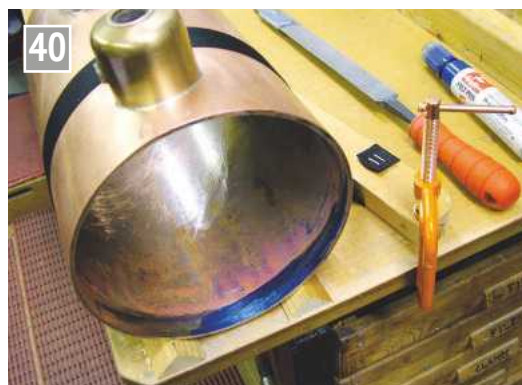
Filing the inner surface, note the protection on the file to prevent scuffing at the far end.
