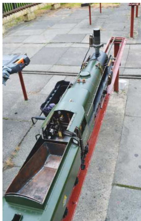
This is Andy Lawton's 3 1/2 inch gauge Britannia. She was bought as a chassis from Station Road Steam, about 75% complete, and finished over the period 2010-2012. The brass boiler cladding is actually older than the builder himself (and he is 72!) who finally found a use for the sheet he had acquired second-hand many years ago and hoarded carefully since then.
