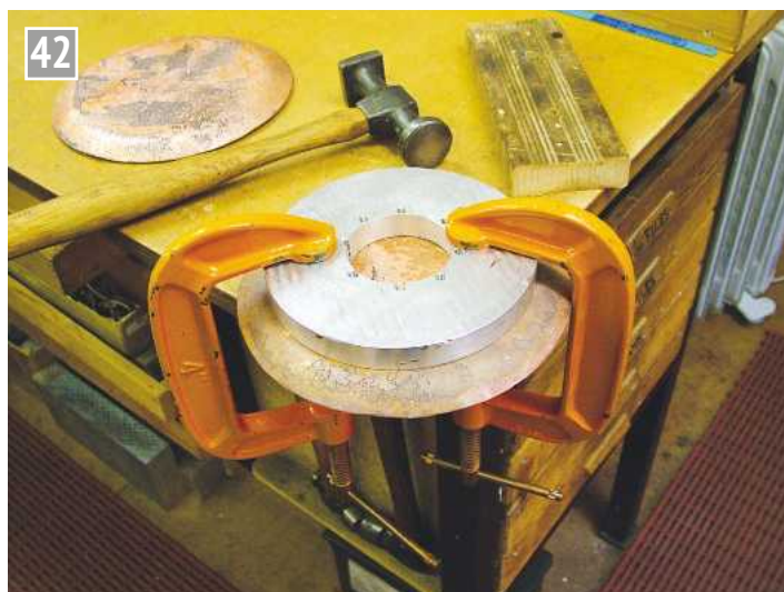
Initial forming of a flanged endplate.
