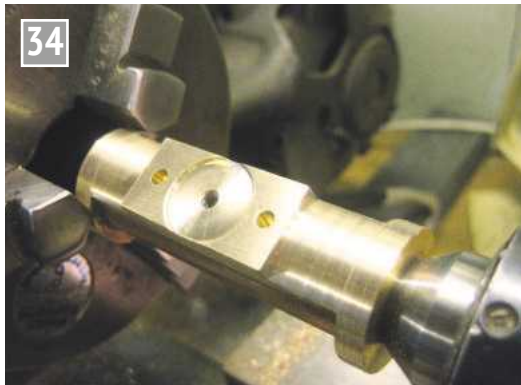
The cylinder assembly is drilled and machined.
