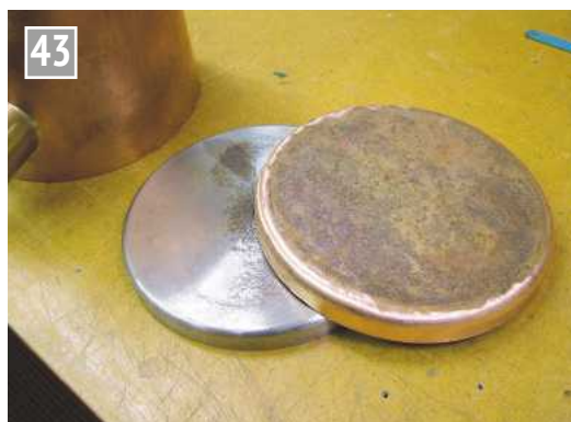
The steel former and the first end plate.
