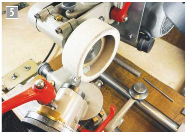
Grinding the side relief.
