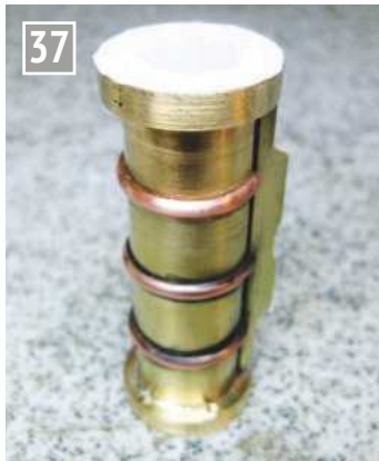
The cylinder had 'strengthening ribs' added.
