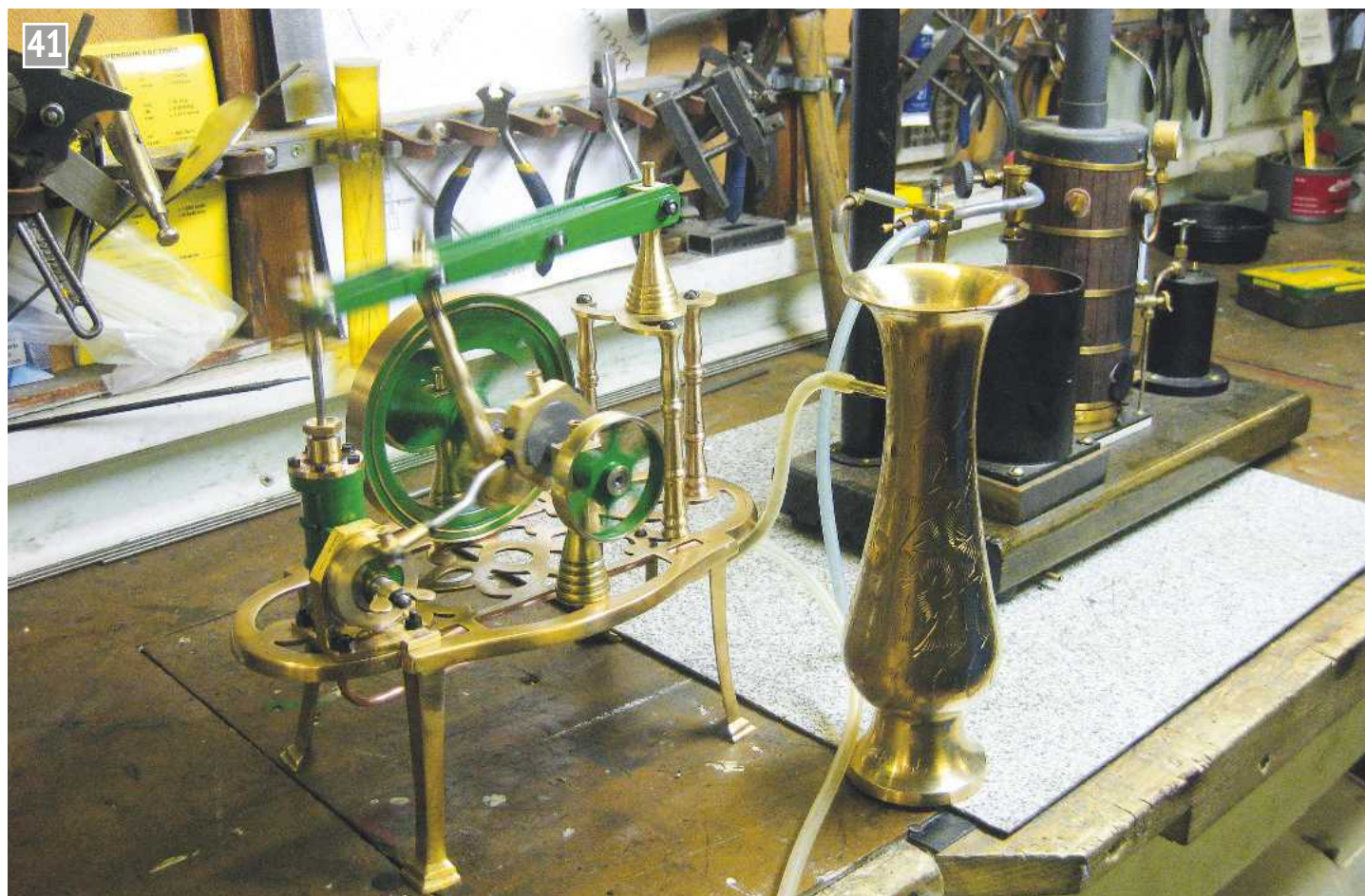
Under test with a rather fancy oil separator.
