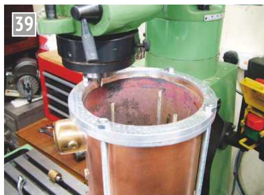
Cleaning the inner face as close as dared.
