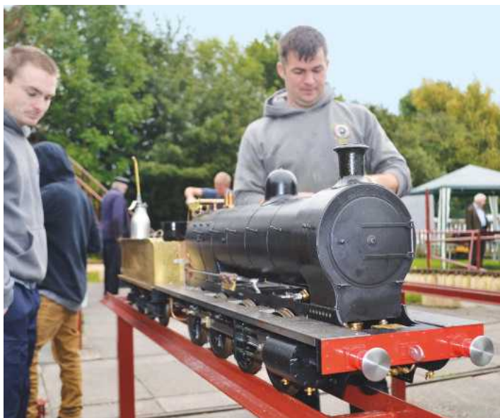
This is Ben Pavier's interpretation of a 5 inch gauge Netta, which was constructed over a period of 4½ years. The cylinders were machined from billets of cast iron rather than castings and are bored out to 1¼ inch diameter rather than the design size of 1½ inch. Cab, splashers and sandboxes are, I am assured, to follow shortly.
