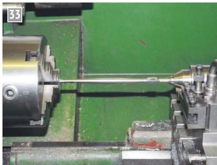
After some hand work, a handsome connecting rod emerges!
