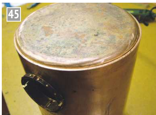
The endplates were held in position by three rivets to prevent moving while soldering.
