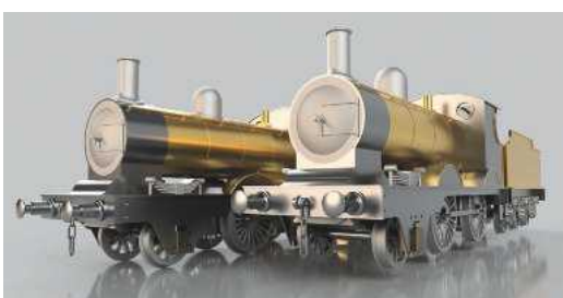
Rose had a single inside cylinder for absolute simplicity - yet it captured the North Eastern look.
