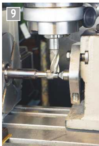
CNC milling helical grooves.
