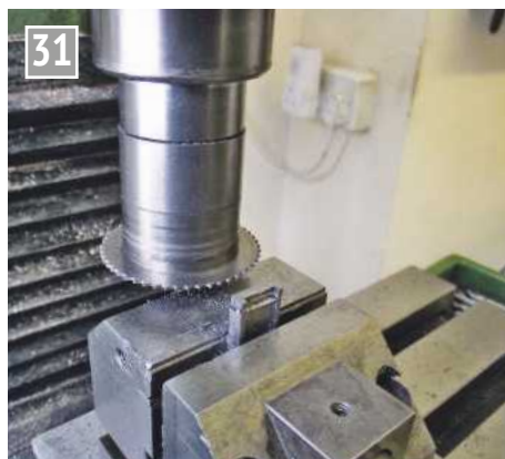
The set up for forming the 2mm thick gibs.
