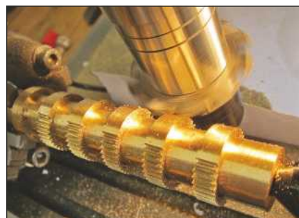
Making Meccano Gears – Chris Taylor goes into production mode!
