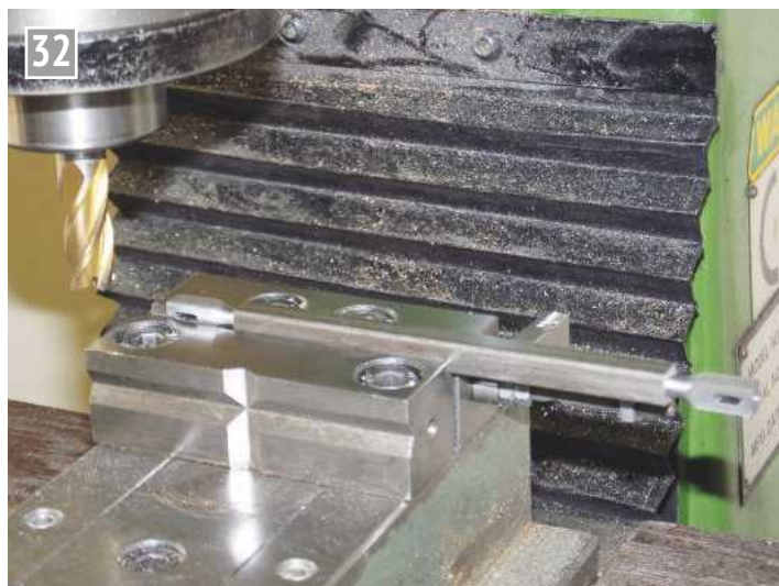
Reducing the square section to 6mm.
