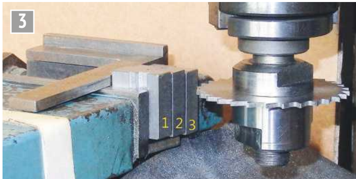
The set-up for machining all the teeth at one setting.
