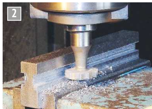
Using a Woodruff cutter to machine the guide groove.
