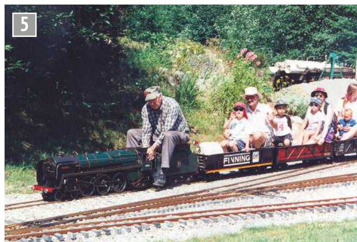
August 2001. Model of No. 70000 at work on the Burnaby track with Lindsay McDonnell on the regulator. The leading bogie vehicle contains the one propane cylinder the locomotive then ran with. (Photo, Mike Johns.)
