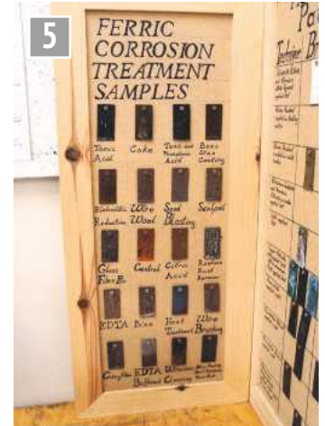
How to treat ferric corrosion - different methods shown by Stacey Hibberd.
