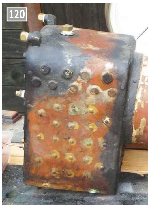
Boiler with copper rivet stays.
