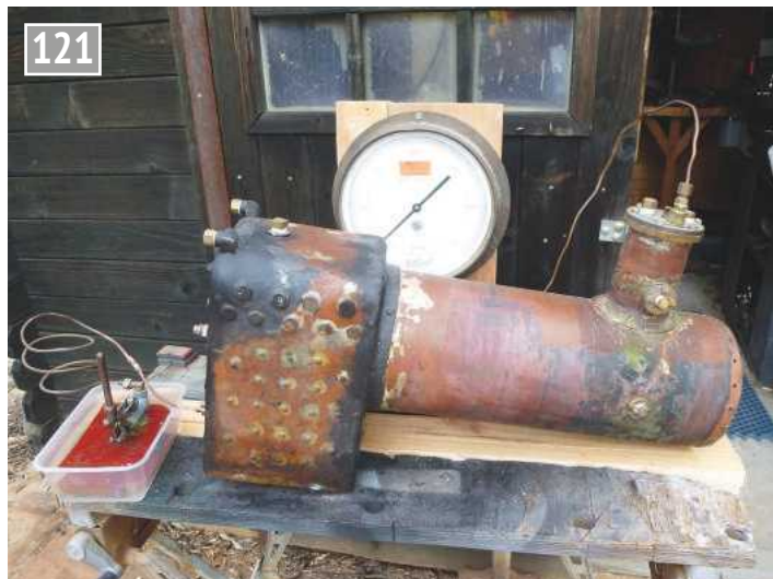
Boiler test in progress.
