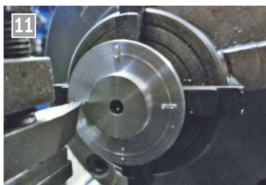
Marking the position of the holes on the cylinder cover plates.
