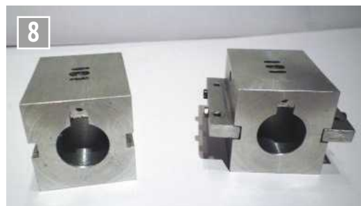
Cylinders bored and ports cut.
