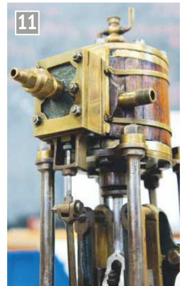
Hallett engine with screw holding strapping round cylinder that had worked loose. Now bulked up with PTFE tape.
