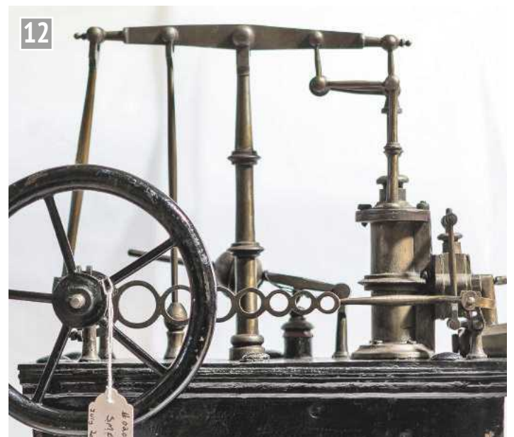
One of SMEE's oldest models made by John Littlewood Naylor in 1843. It had the condenser underneath and was known as the 'poker engine' using a red hot bar to heat water.
