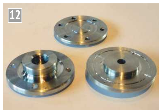
Cylinder end covers drilled and deburred.
