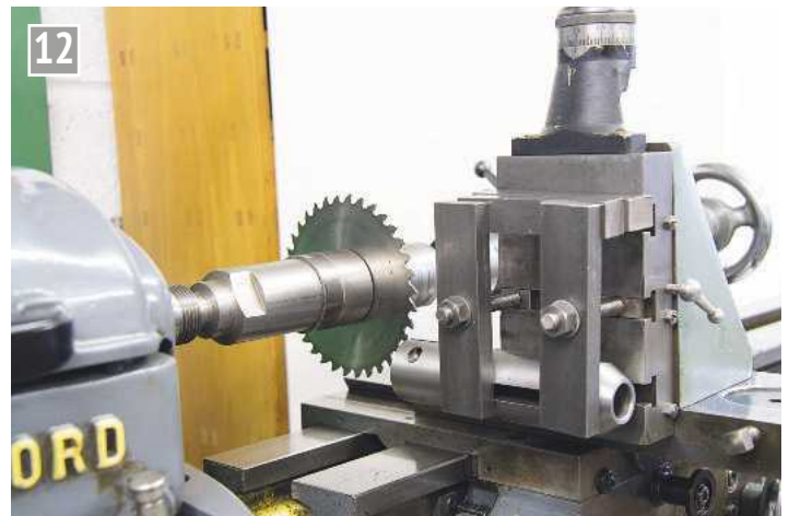
Use of a vertical slide for slitting the main body.
