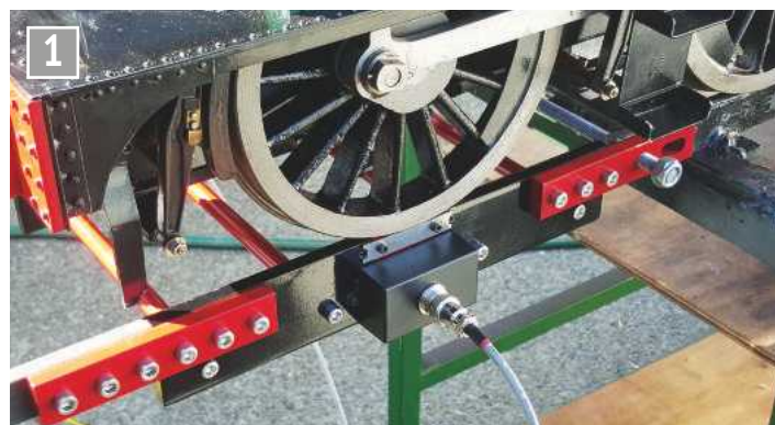
Peter Targett's axle weighing gauge, Hutt Valley & Maidstone Model Engineers' Society. (Photo courtesy of Peter Targett.)
