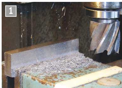
Machining a jaw blank to exact width.
