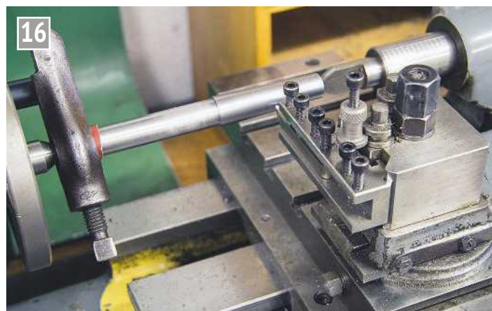
Turning the Morse taper between centres.
