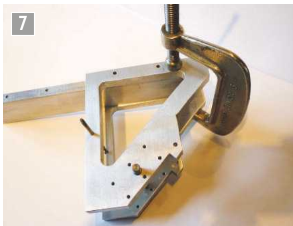
The frame clamped to the base spacer.
