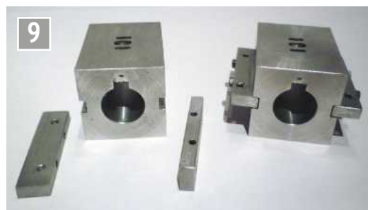
Cylinder support bars in the foreground.
