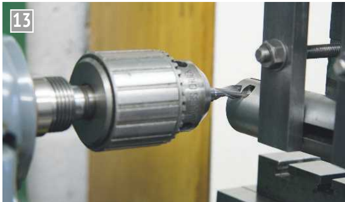
Producing a pocket with a slot drill to start the hole for the clamp screw.
