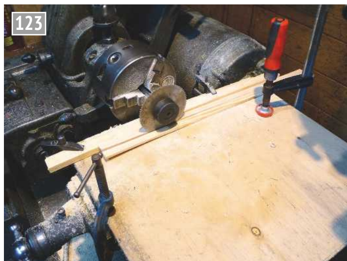
Jury-rigged slitting on the Myford.
