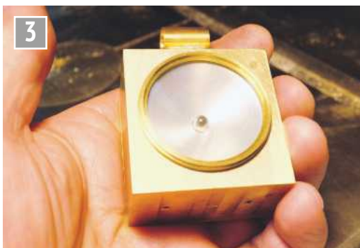
Reflector in the headlight casing. LED in the 5mm hole, round glass installed; the headlight is close to completion.
