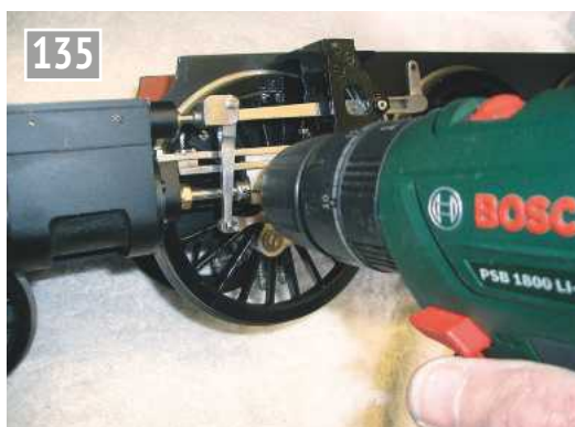
Drilling roll pin in cross head / piston rod.
