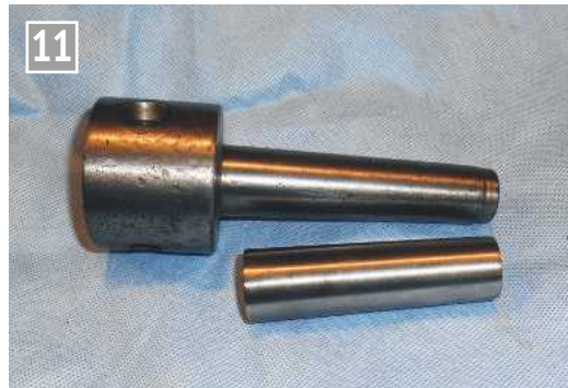
Finished adapter and original arbour.
