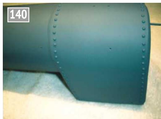
Back head riveted in position.
