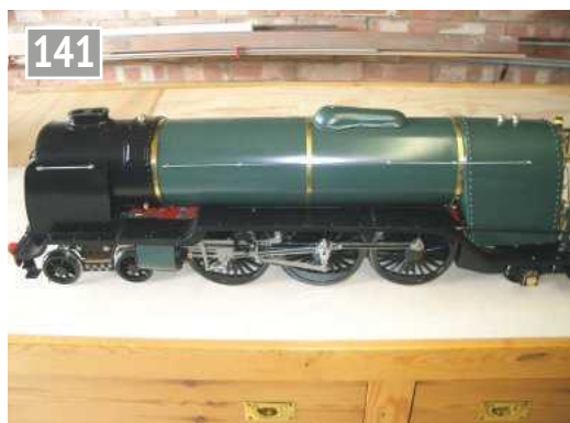
Boiler with brass bands assembled on the frames.
