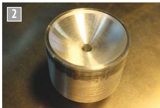
Reflector as machined but requires polishing. Outside diameter finish turned and chucking spigot removed.
