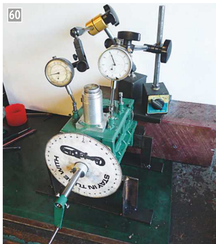
Setting and testing top dead centre.
