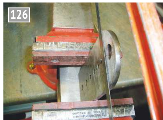
Sawing the bolt to length.
