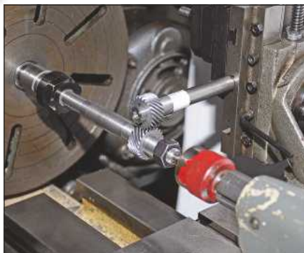
➤ Jeff Thyer adapts his Myford lathe for hobbing helical gears.
