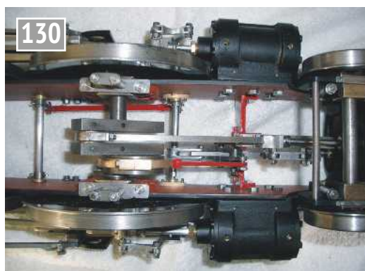
Centre crank, connecting rod and valve gear.
