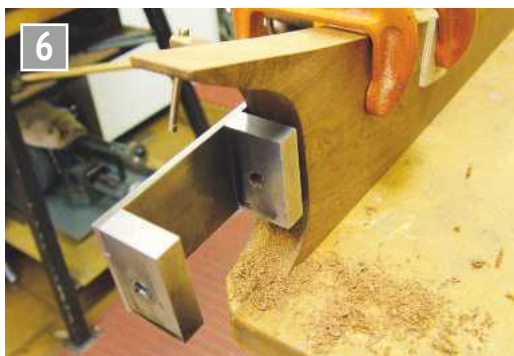
The mild steel jig for drilling the hole for the stern tube
