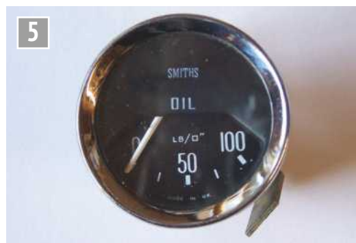
A typical 52mm diameter automotive instrument.
