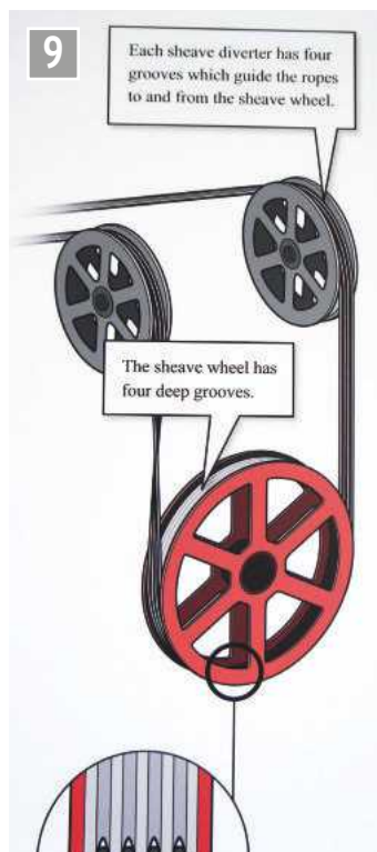
Diagram of the sheave and winding wheels displayed on a poster at the Tramway (Courtesy of Richard Gregory: www.richardpalmergraphics.com )
