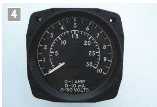
The 240 degree movement meter.
