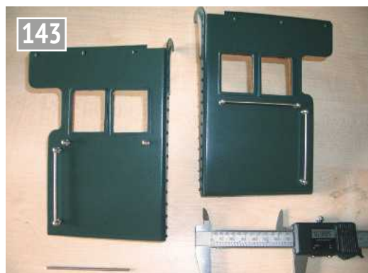
Hand rails fitted to cab sides.
