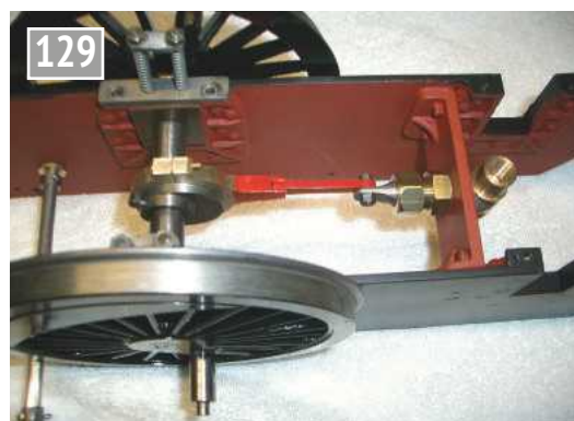
Feed pump in position.
