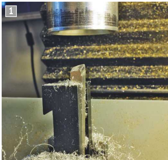
Aluminium stock mounted in the CNC mill spindle; the tool on the table; the headlight reflector surface is almost finished.
