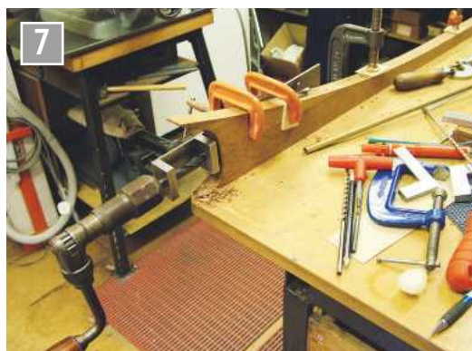
Drilling the hole using a long series drill in a carpenter's brace.
