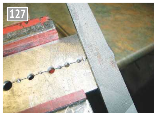
Finishing the bolt with a file.
