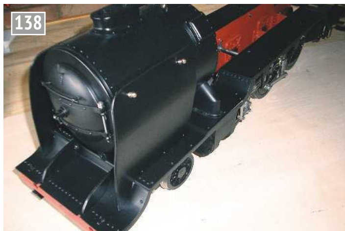
Smoke deflectors and running boards in position.
