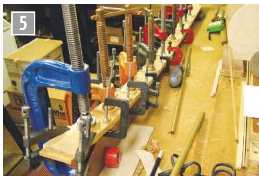
Laminating the Hog to the curvature of the keel.
