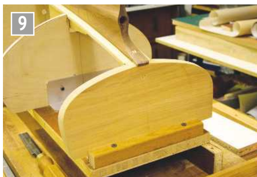
The transom was built from three pieces grooved and keyed together.
