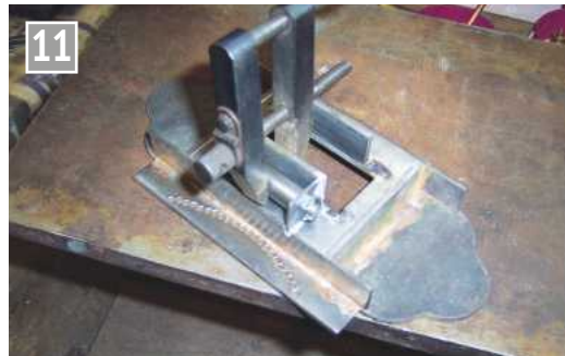
A simple jig supports a side control spring housing plate.
