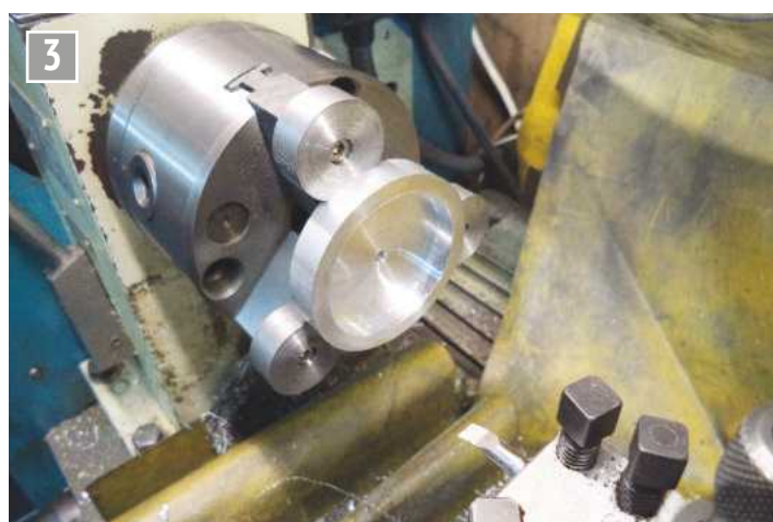
Boring out using soft jaw extensions.
