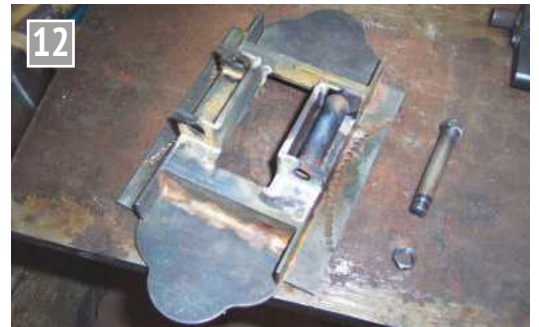
Spring housing plates brazed in position.
