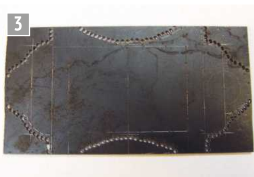
Marked out for chain drilling.
