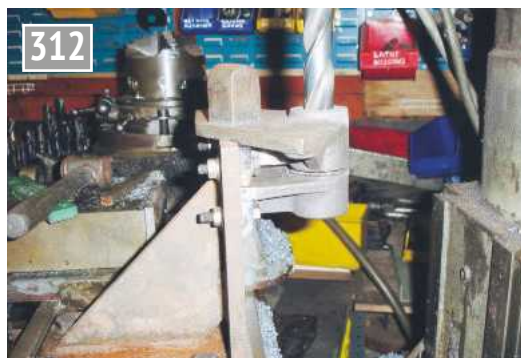
Drilling steering brackets.
