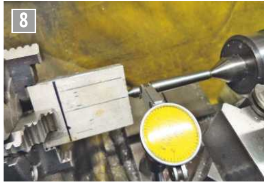
Clock the valve body true in the four jaw chuck.
