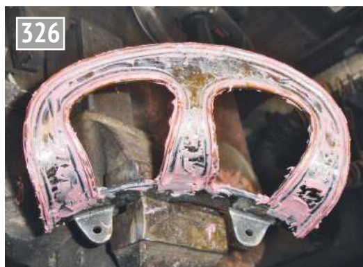
Filler applied to hose carrier.
