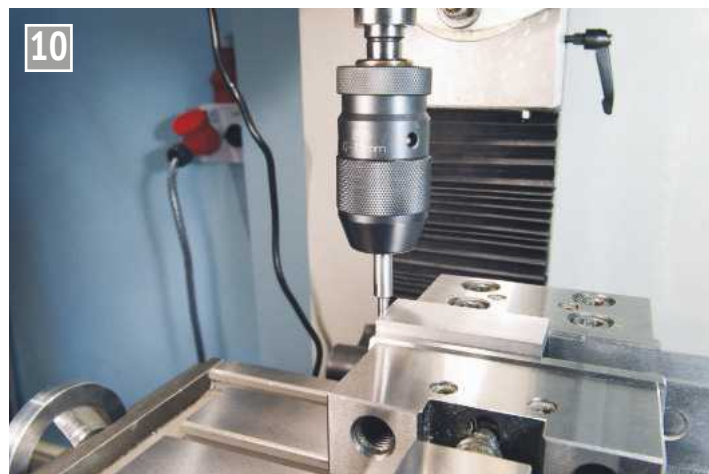
X- and Y-axis handwheels were set to zero.
