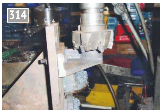
Milling the lower steering bracket.
