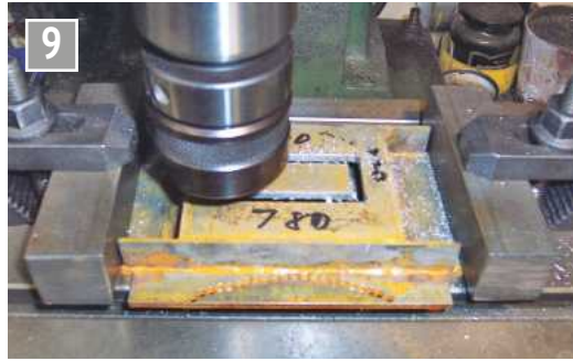
A two flute cutter removes the centre section.
