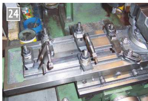
The set-up for machining the four longitudinal bars.
