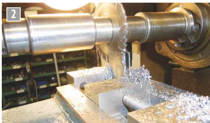
Slotting the lifting arms of the crucible.
