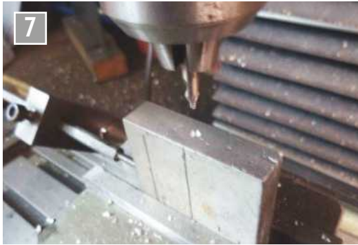
Centre drilling the valve body.
