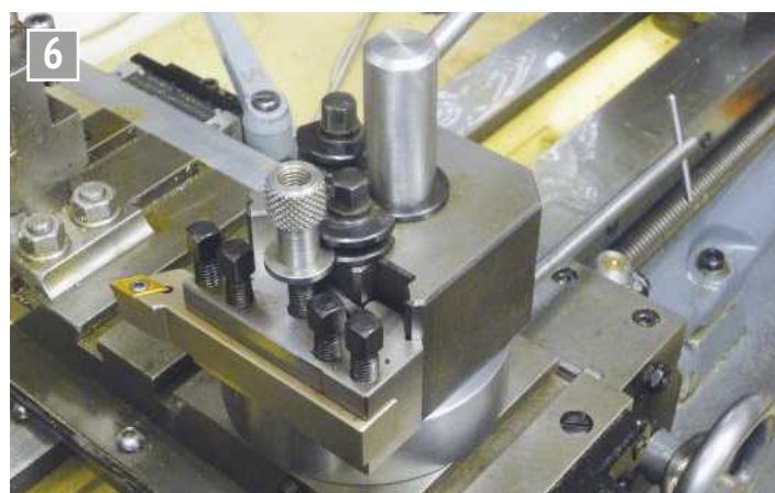
Top view with a 16mm tool holder in use.
