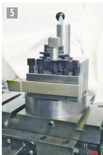
Mounted on the Super 7 with 16mm tool.
