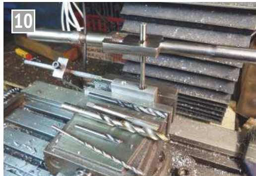
Drilling the oil ways.
