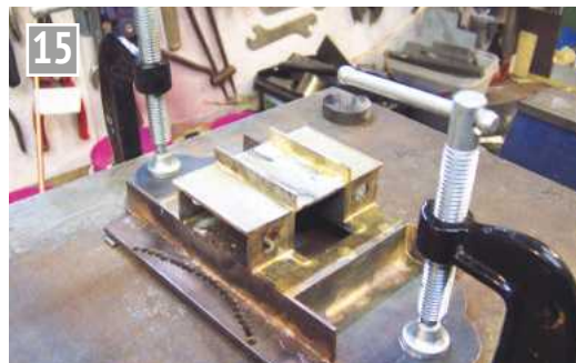
Correcting a slight misalignment with G-clamps.
