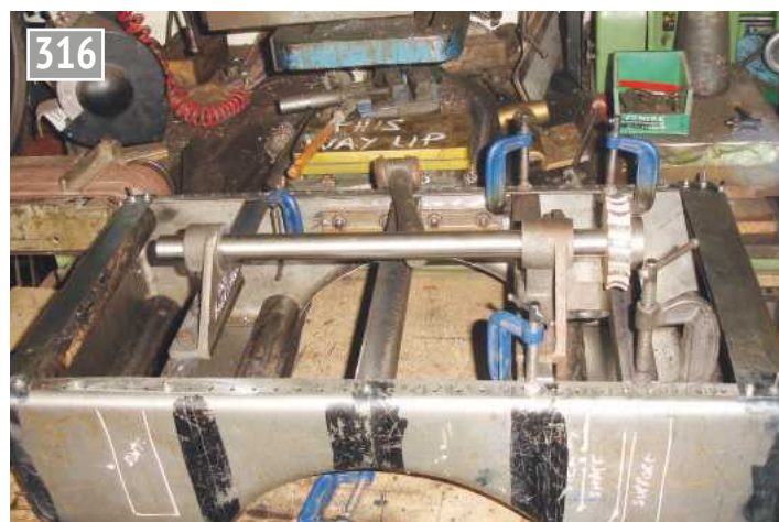
Steering shaft in position on the belly tank.
