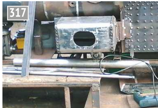
Belly tank refitted.
