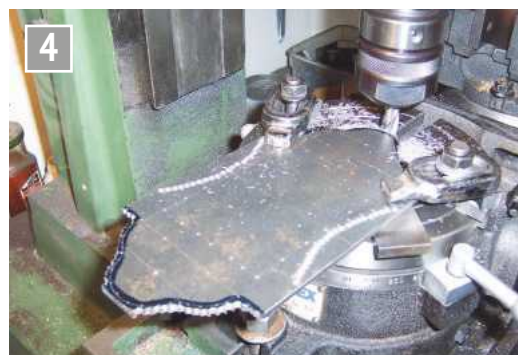
Profiling the 3/4 inch radius.
