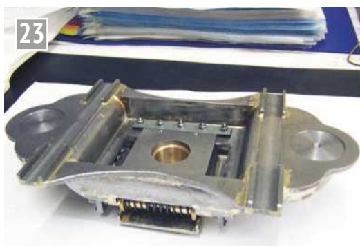
The complete pivot bearing unit inside the bolster.
