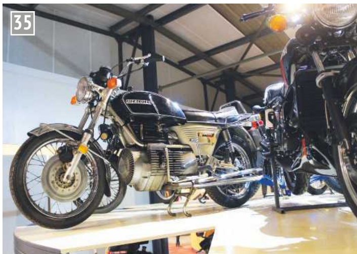
The DKW Hercules built in 1979 had an unusual rotary engine, but did not sell well.
