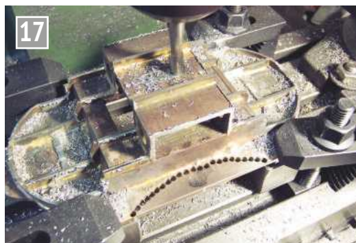
Machining the bogie pivot slot.
