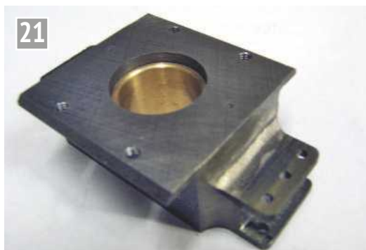
Gunmetal pivot bearing within the machined block.
