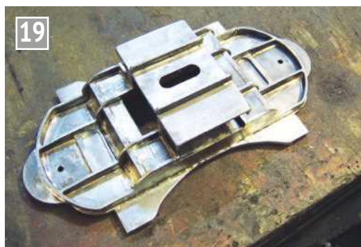
Underside view of the bolster.
