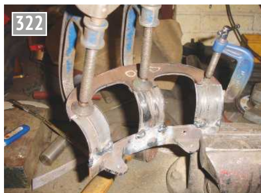
Fabricating a water hose carrier.
