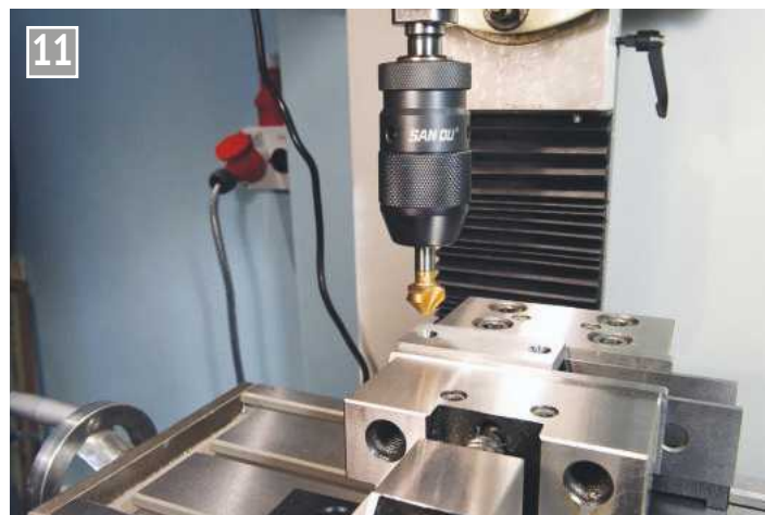
Countersinking at low speed.
