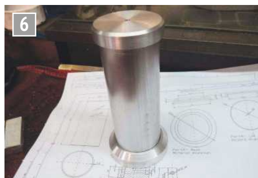
Trial assembly of body, base and lid.
