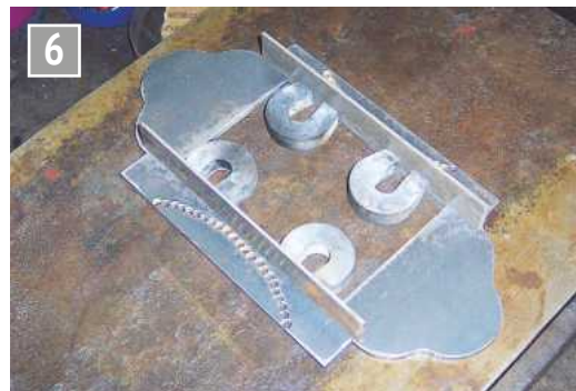
Using magnets to hold the 1/16 inch plates for soldering.
