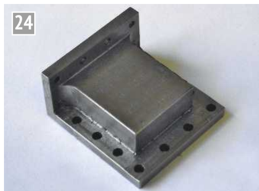
The completed steam chest.
