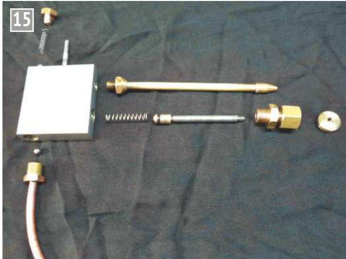
Pump parts ready for assembly.
