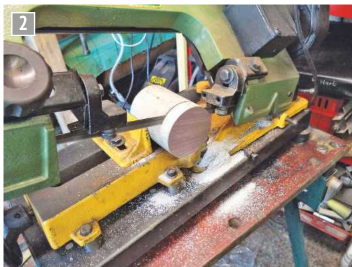
Cutting the bar into slices for the lid and base.
