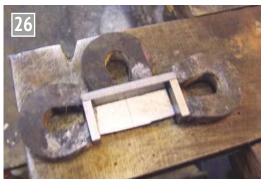
Components of the horns ready for soldering. Magnets in use again!
