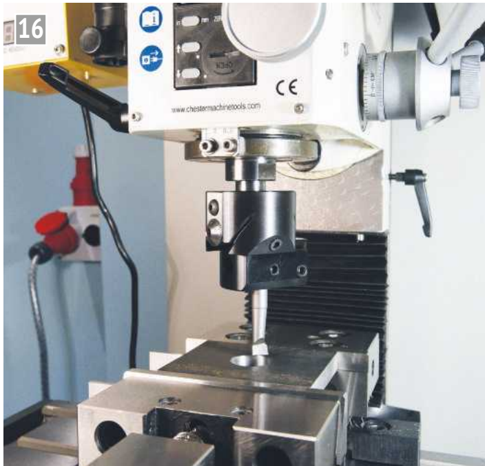
Boring up to 1 inch diameter.
