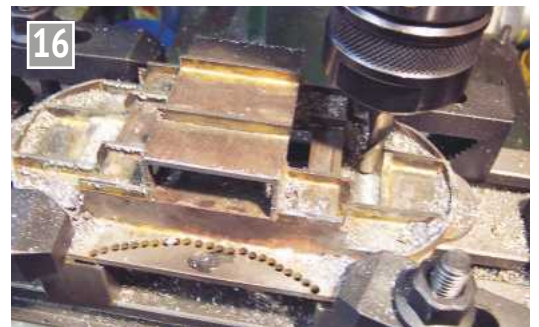
Forming the spring pad recess - an underside view.
