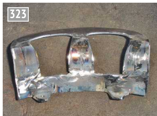
Hose carrier welded and partially cleaned up.
