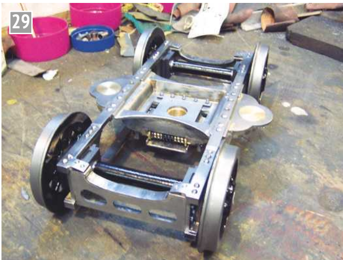
Now with the stretchers, wheels and axleboxes in place.
