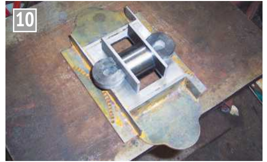
Magnets in use again to assist with the silver-soldering.
