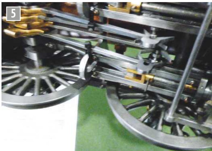
Lion's 'gab' valve gear on the OLCO stand at Doncaster.
