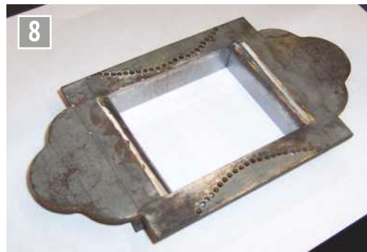
The shoulder plates in position.
