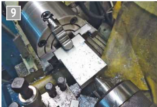
Turn the valve body to a tight fit in the tube.
