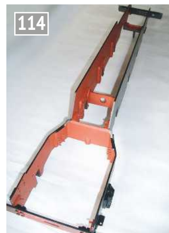
Main frames painted.
