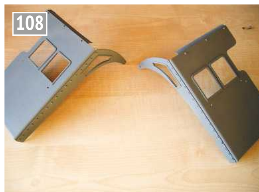
Riveted cab with window frames attached.
