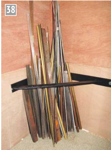
Corner space utilised to store small diameter stock.
