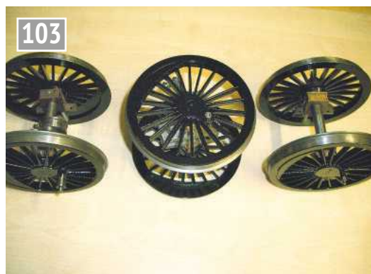
Main drive wheels painted.
