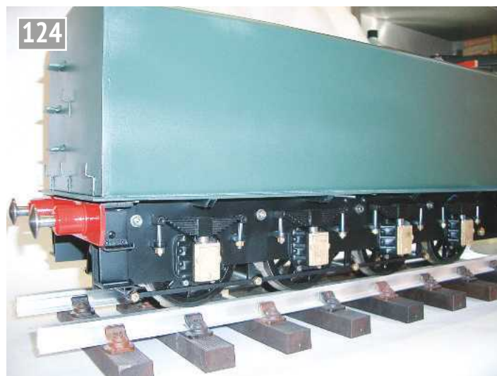
Tender assembly rear view.
