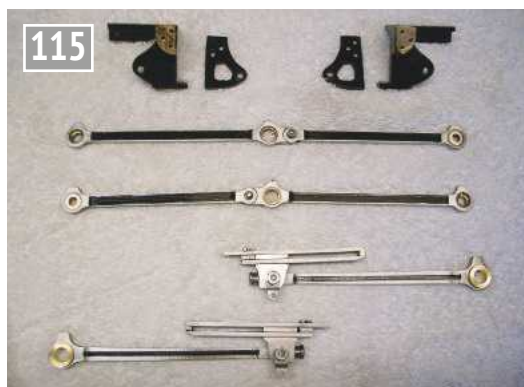
Motion brackets, coupling and connecting rods painted.
