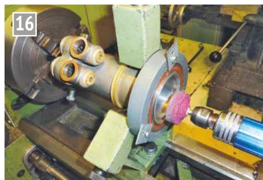
16 Set-up for internal grinding. Note the ball race fitted to the steady. This was set accurately to the lathe axis and dowed to the steady so it could be removed and replaced as necessary during operations.
