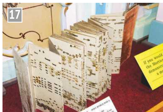
Music is controlled via a Jacquard punched card system.
