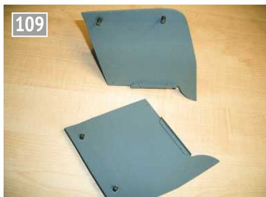
Smoke deflectors with spacers and fixing angle.
