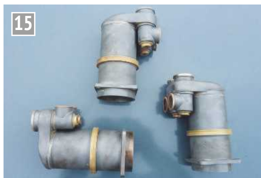
15 Finished cylinders. Note the valve housings set at 3 degrees to the main axis. The weld is almost invisible. The copper jackets will bond to the brass flanges.
