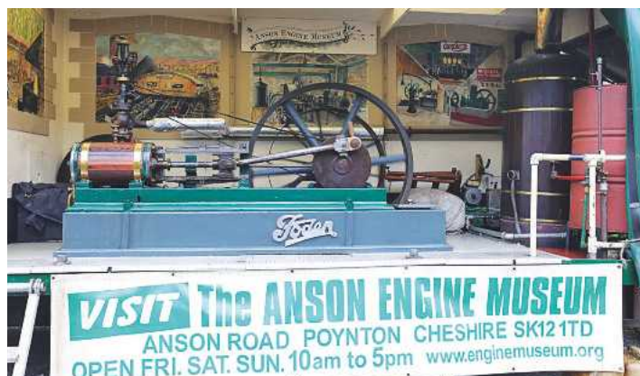
From the Anson Engine Museum, Poynton, this horizontal mill engine complete with vertical boiler is regularly displayed at Lancashire and Cheshire rallies by Geoff Baker.
