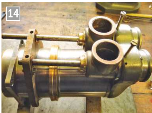
14 Cylinder head and two valve housings being lined up with the transfer plate. Various pins and screws hold everything in place during brazing.
