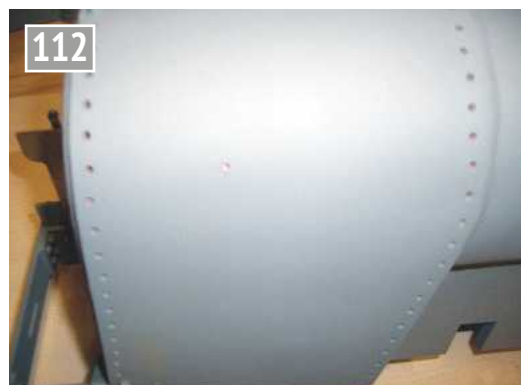
Rivet holes in fire box and back plate.
