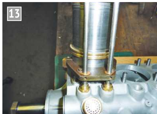
13 Transfer plate clamped around the lower part of the cylinder. Adjustable bushes register the exact position of the two rods that represent tappet axes.
