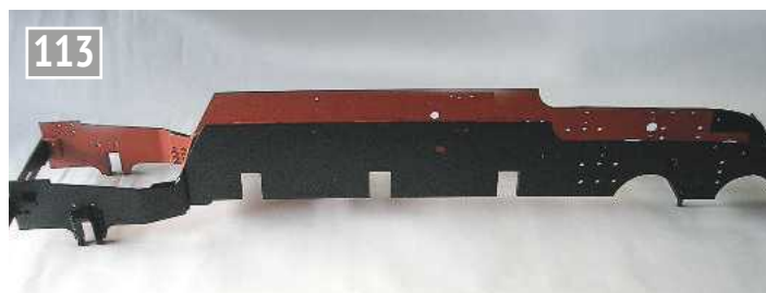
Main frames painted.
