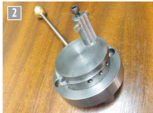
A flat is machined on the left side of the post to provide clearance next to the job.
