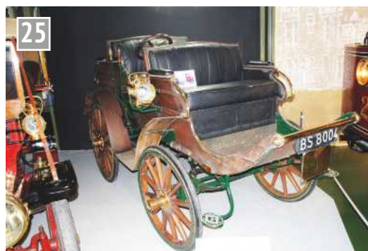
Scottish made Arrol-Johnston dog cart of 1902 with an opposed piston, two cylinder engine. Dog carts remained popular in Scotland longer than elsewhere.
