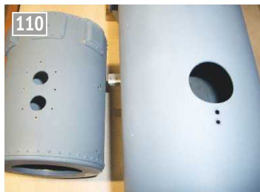
Chimney and regulator fixing holes in boiler and smokebox.
