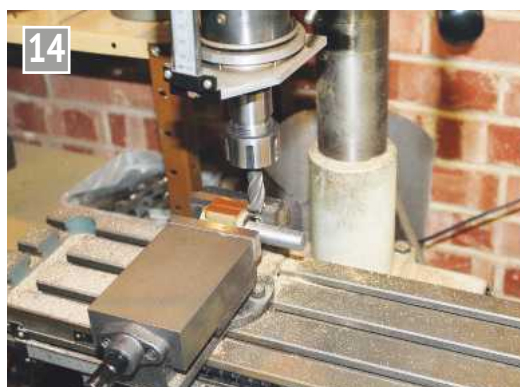
Milling the port face.
