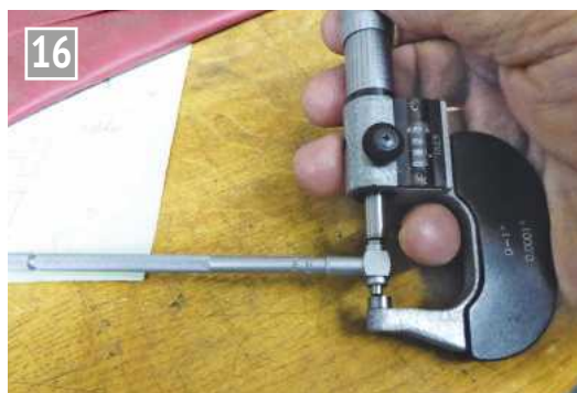
... and a micrometer is used to finally check the bore size.
