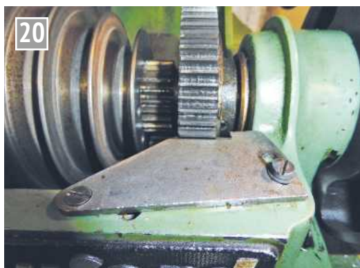
It is cut from 1/8 inch BMS plate and the part that enters the bull wheel, is shaped to fit the wheel's tooth.
