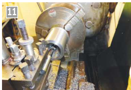
Now, with a change of boring tool, the central hole is bored to size.
