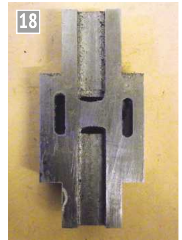
Showing the various slots and steam passages.
