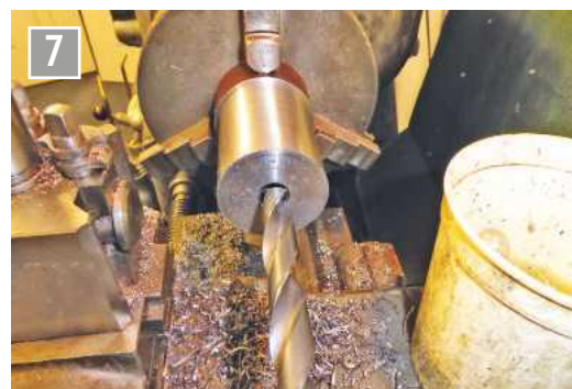
... until the hole is opened out just below finished size, which will be obtained by boring.
