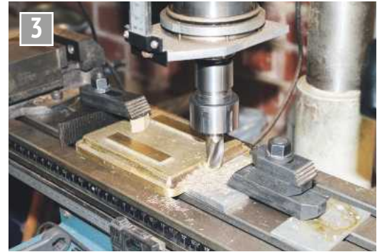
Milling the edges of the base.
