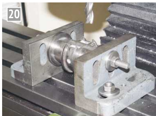
Set-up for machining the valve seat.
