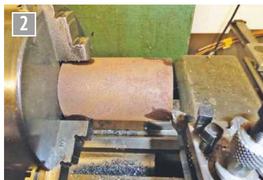
This rusty lump provided material for the main 'master' die holder, as well as for the drilling jig.
