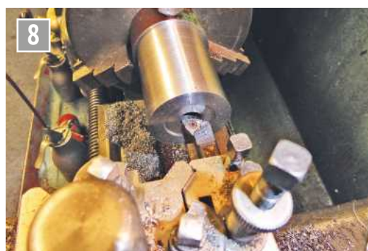
First, start to bore down to match the die holder thickness, towards the finished depth ...
