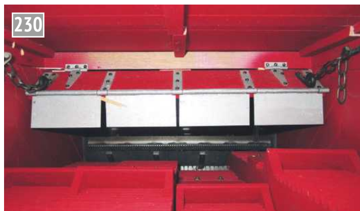
Check plates viewed from the front.
