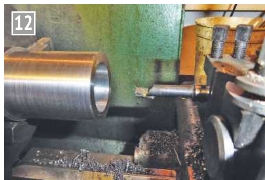
This tool is sturdy and the overhang is kept as short as possible.
