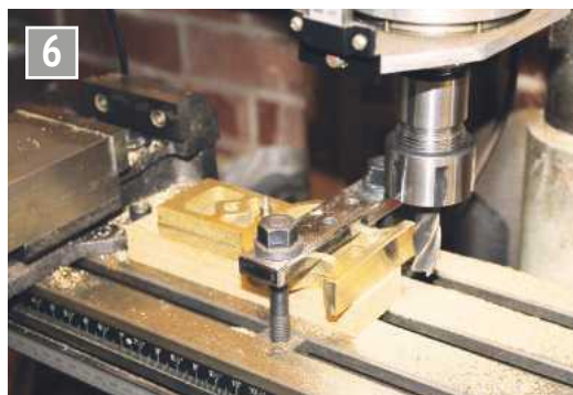
Milling the side frame feet.
