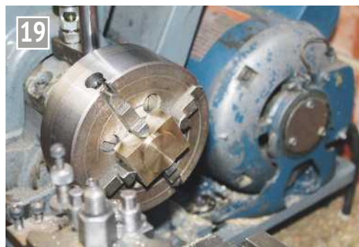
The bosses are turned in the four jaw.
