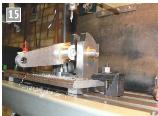
Drilling and reaming the dowel holes.
