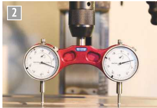
Setting the head using an EDGE Technology Pro Tram.
