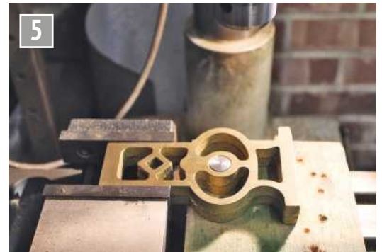
Holding the frames in the mill vice.
