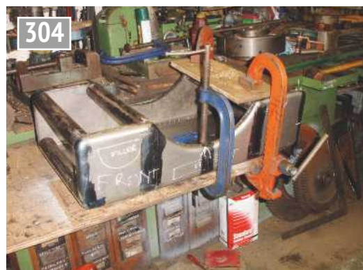
The end/top piece clamped.
