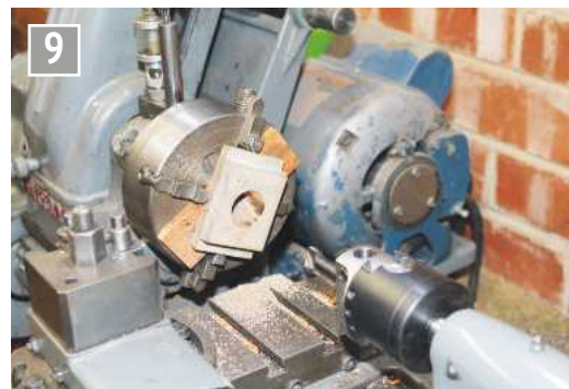
Set-up to bore the table.
