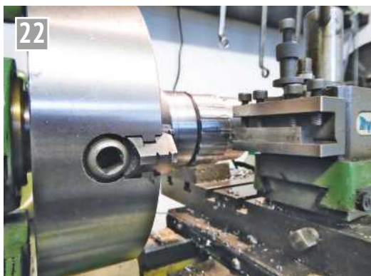
By keeping indexing round, an easy to hold grip is produced.
