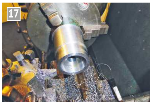
Now, I have taken a cut across the outside to reduce the length of the grip that I produce with the next operation.
