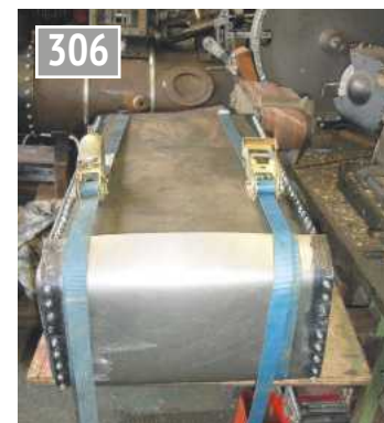
Ratchet straps used again as 'pullers'.
