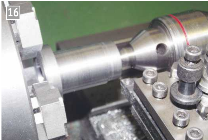
A method using tailstock support.
