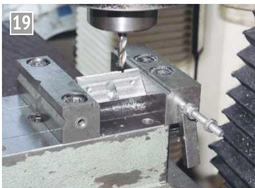
Machining the angled hole with an end mill.
