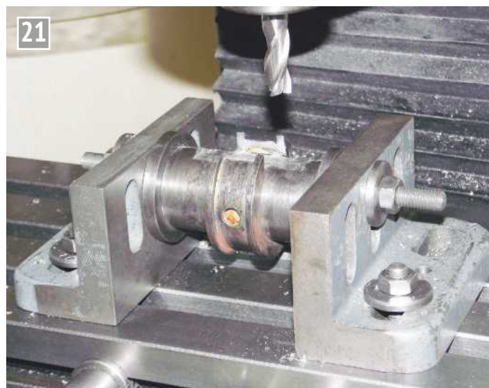
Machining the second seat.
