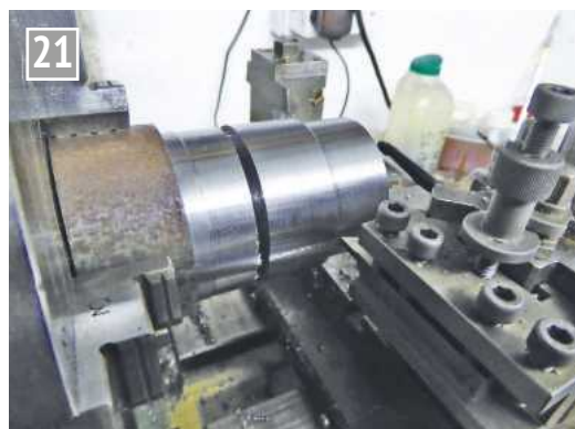
With a round nosed tool set at centre height, on its side and advanced about 2 thousands of an inch per cut, a groove is produced as a grip.
