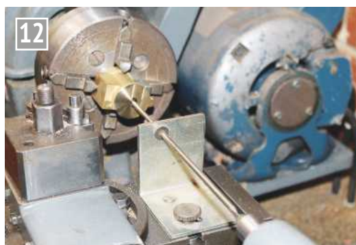
The cylinder being centred in the four jaw with the help of a home-made wiggler.
