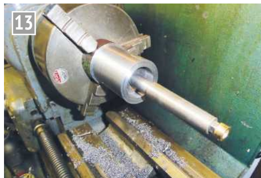
A test piece, in my case the taper slider from the original set, was used to check the finished bore size.
