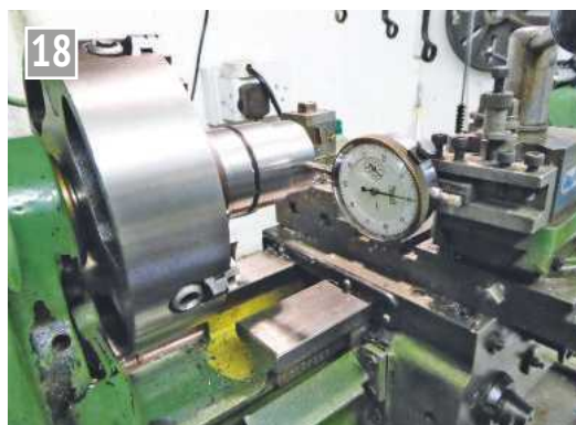
The work is transferred to the smaller lathe which has dividing facilities; here it is being centred in the four jaw chuck, which I chose to use to better hold the long overhangs.
