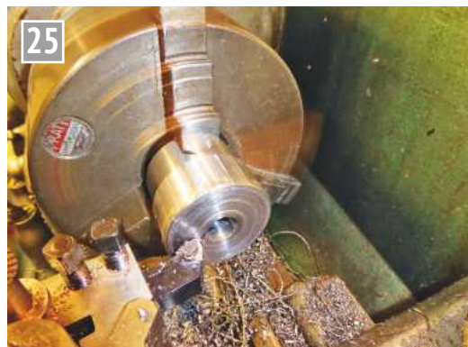
With the job reversed in the three jaw chuck, the parted off face was cleaned up.
