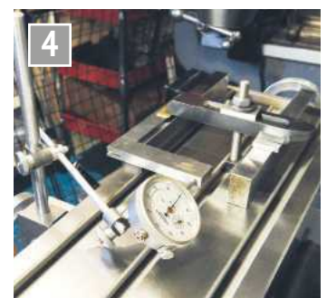
Checking the X and Y axes are square.
