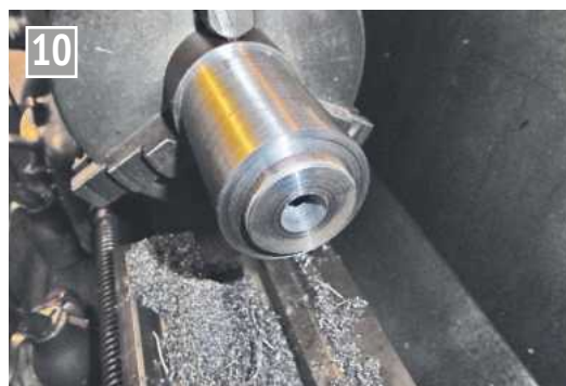
The bore should fit the die holder blank easily, but without slop.
