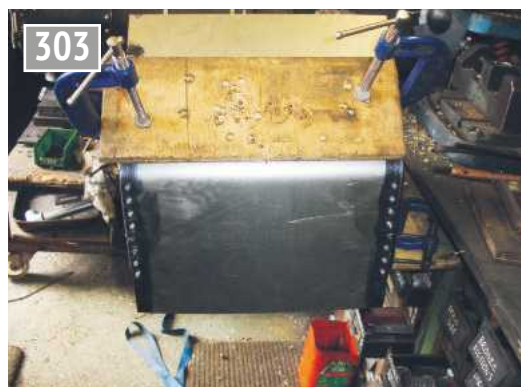
Wrapping the end piece around the stay tube.
