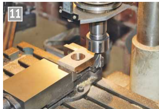
The table sides being milled.
