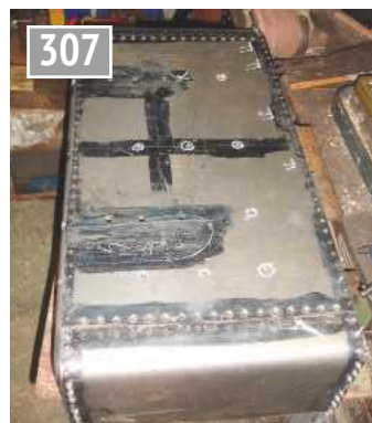
The completed belly tank base.
