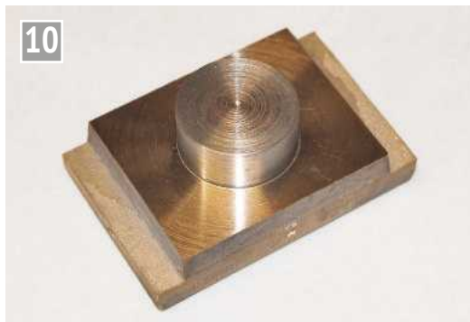
The table top with its plug, ready for milling and drilling.
