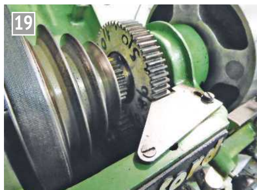
This simple device, with the painted 60 tooth Bull Wheel, allows simple dividing, in this case 20 positions per revolution.
