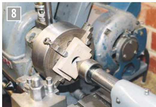
Ready to machine the table top.
