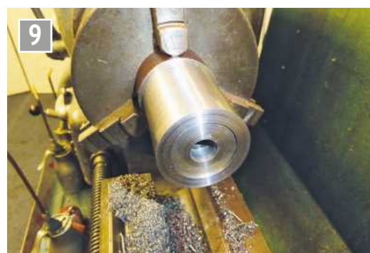
... opening the hole up to final size after reaching finished depth.
