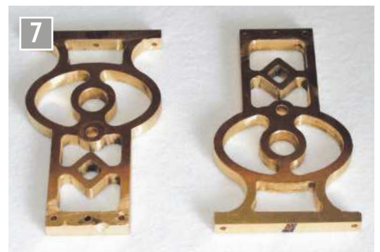
Starting to polish the frames (note the damage!)
