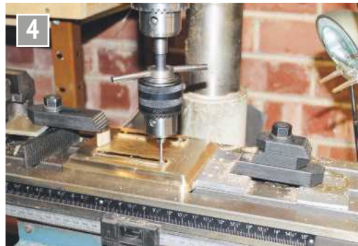
Tapping the mounting holes.
