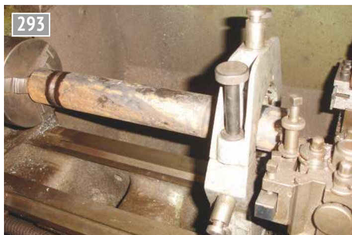
Turning the belly tank stays.
