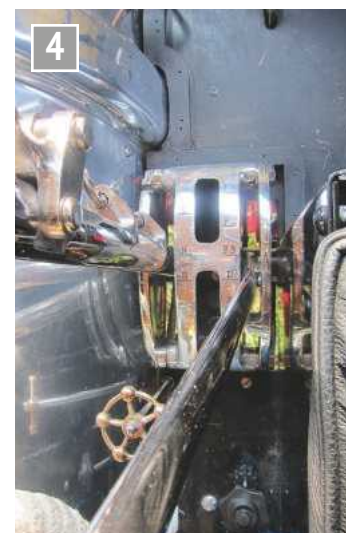
The driver's controls; high and low gear on the left and 'cut-off' on the right.
