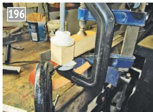
Clamping after applying adhesive.
