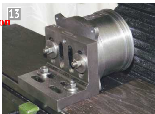
The set-up for machining the base casting's cylinder flange seating.
