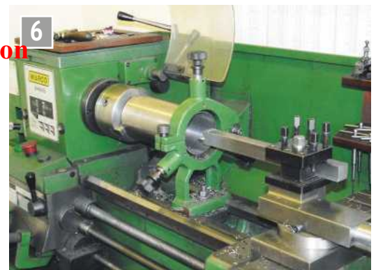
6 The overhang of the boring bar made machining the taper in one go impractical.
