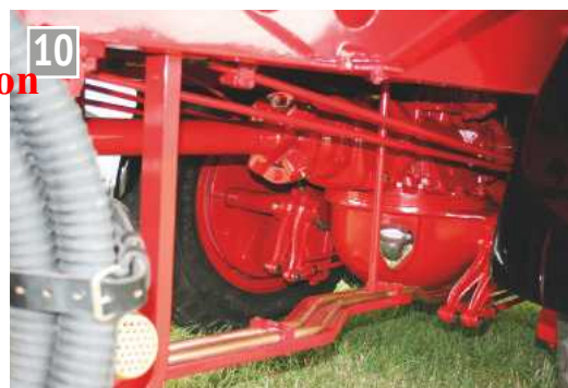
The Speed 12 showing the forward of the pair of worm and wheel differential units on the back axles.
