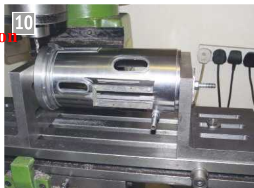
Using the angle plate set-up once again, the slot for the flywheel is cut.
