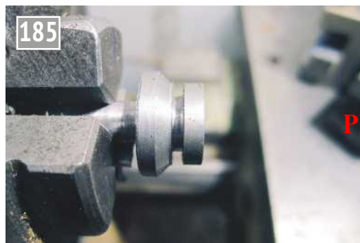
Turning the form of the cutter. This will be the tongue.
