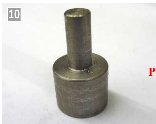
A stub for the alignment of the chuck/ rotary table.
