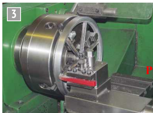
The flywheel casting mounted in a four jaw independent chuck.
