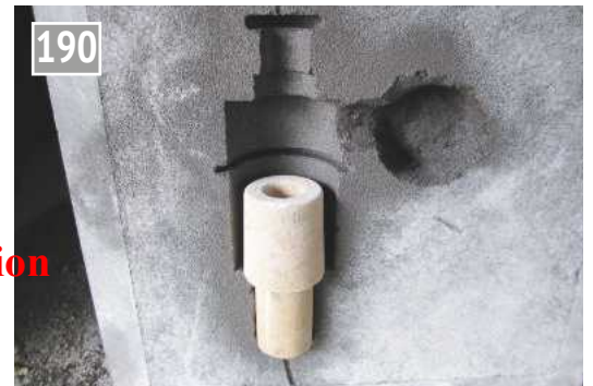
The mold rammed up and the core in place.
