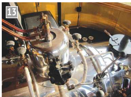
Diver's view of the top of the boiler.
