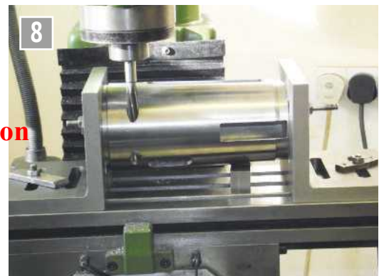
8 The set-up using angle plates. A three flute 6mm end mill with an extended cutting edge cut without deflection.
