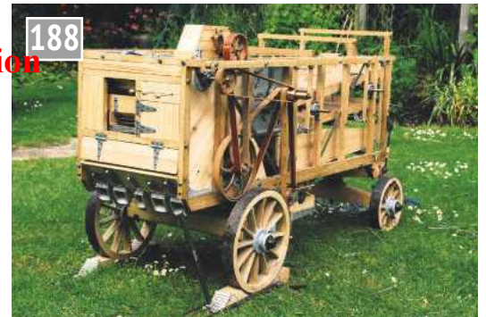
The partly clad threshing box.
