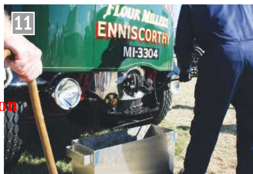
The fire hole door at the front is used for lighting up and raking the fire. When being driven, coal may be added from the cab via a top chute.
