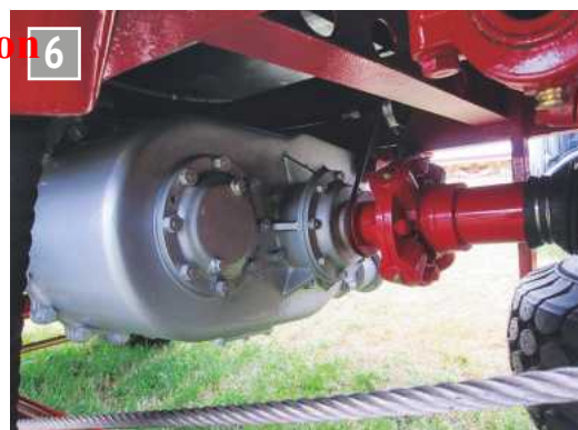
Aluminium castings were used where possible.
