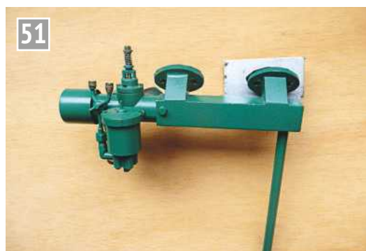
Manifold after painting.
