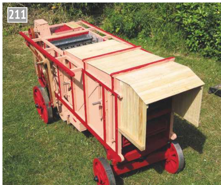
The wind hood under construction.
