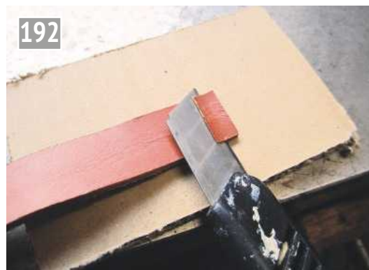
Starting to make a scarf joint.
