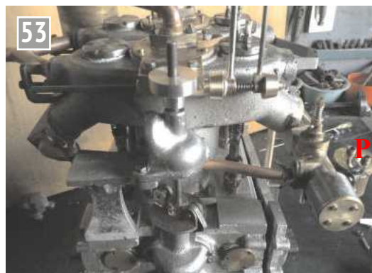
Under construction; showing the machined castings in place.
