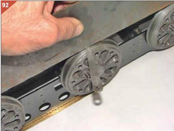
92 Checking that the wheels are dead level.
