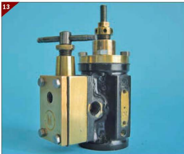
Cylinder showing the inlet, exhaust and governor bracket.
