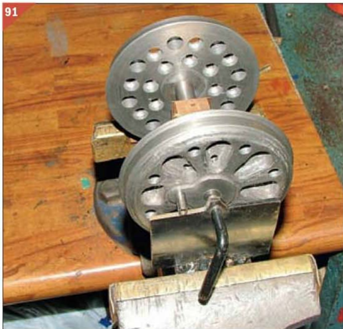
The other side of the quartering jig.
