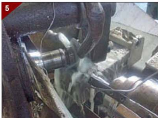
5 Forming the flutes with a profiled milling cutter.
