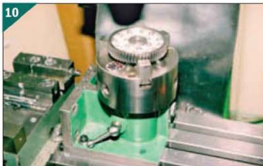
Drilling holes prior to milling the spokes.
