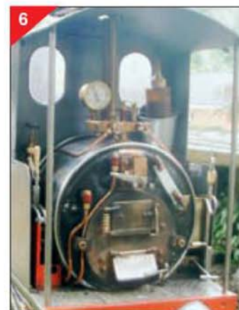
A view of No. 5 showing the marine type boiler.
