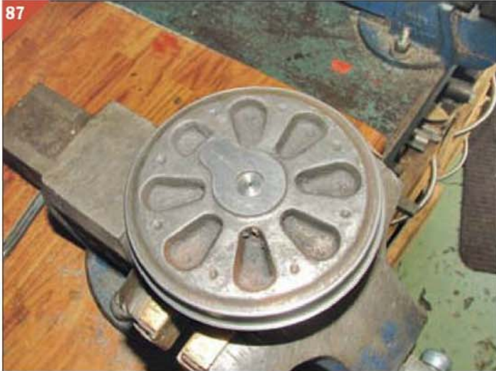
87 Marking the radial line for the crankpin.
