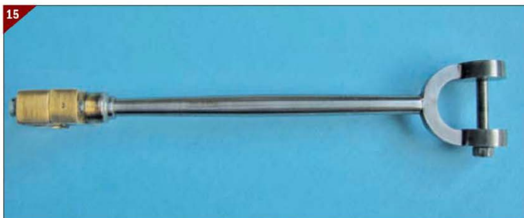
Connecting rod showing the fork.
