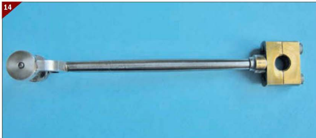
Connecting rod showing the big end.
