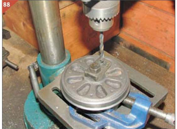
88 Drilling for the crankpin.
