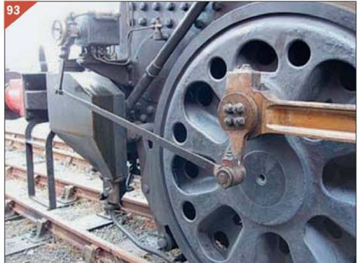
93 Return crank and mechanical lubricator drive on C1.
