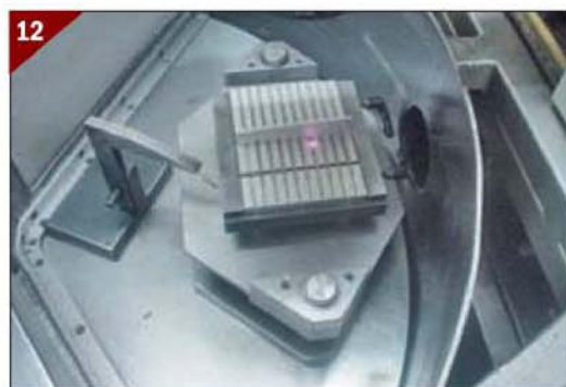
Laser marking 2mm dia. hand reamers.
