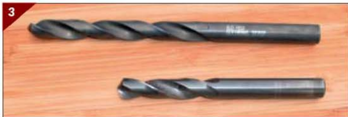
3 A stub drill compared to a standard drill of the same size.
