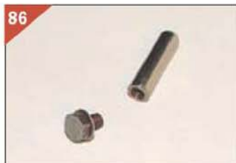
86 The simple plain crankpin, no shoulder, just press in to required depth.
