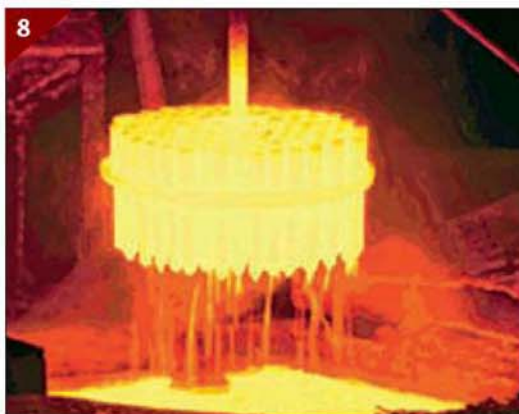
8 Tools as they leave the heat treatment bath.
