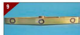
Top view of beam, the circles indicate pins used for assembly.
