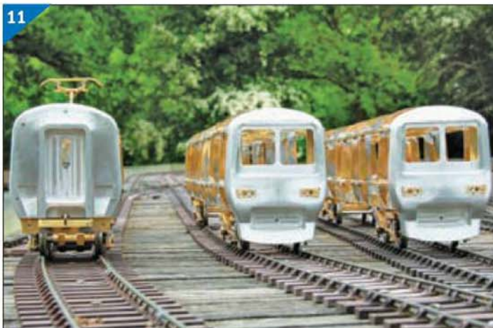
Different ends from solid aluminium.
