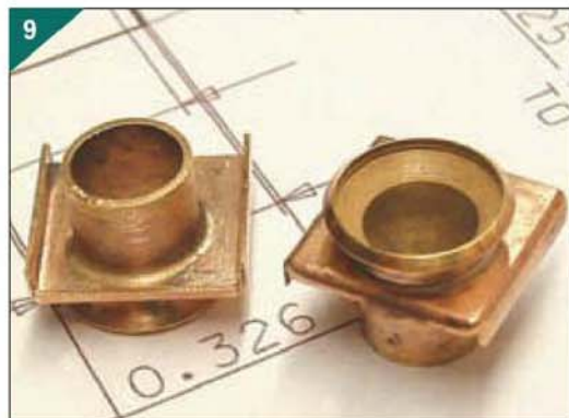
The bezel soldered to the front plate.
