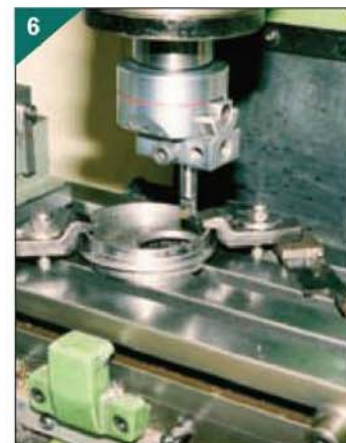
Boring the boiler ends.
