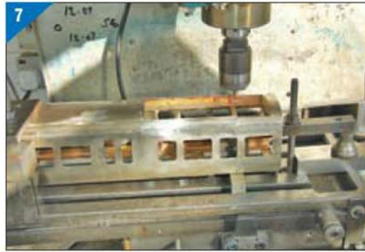
Milling the roof to take the pantograph.
