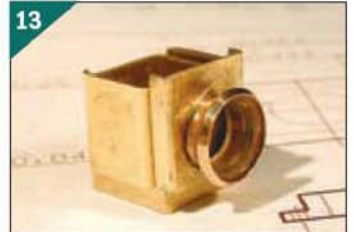
Front panel and bezel assembly fitted to body.
