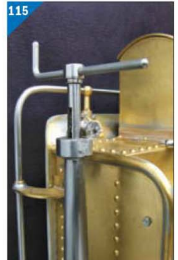
Water scoop operating column.
