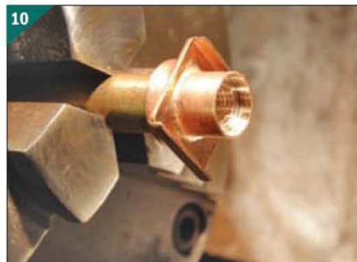
The bezel mounted on a mandrel.
