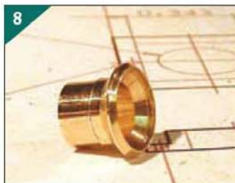
The lens bezel with extended spigot.
