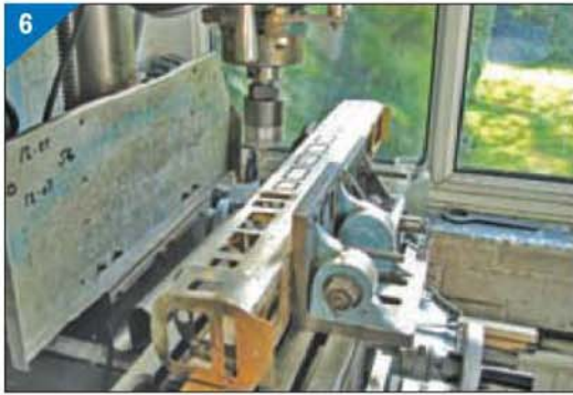
Milling the windows.
