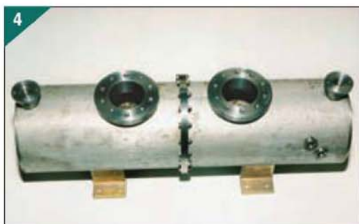
The boiler showing the supports underneath.
