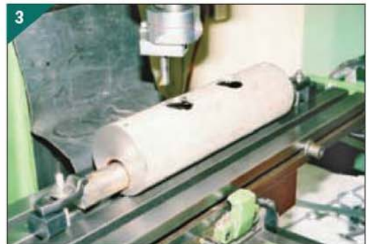
Boring the holes in the boiler.
