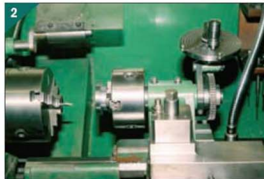
Drilling the cylinder mounting stud holes.
