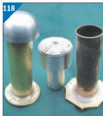
Making the tank ventilators.
