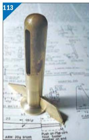
Making the water level indicator.
