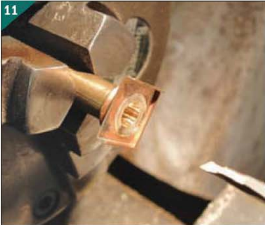
Removal of excess spigot.
