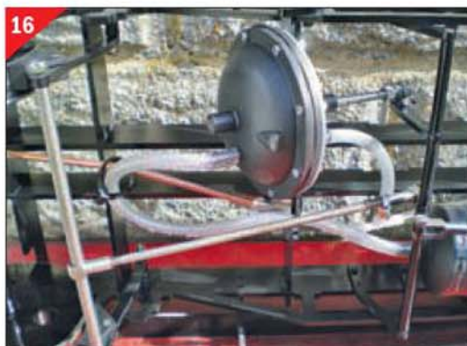
16 The vacuum system piped up with reinforced plastic tube.
