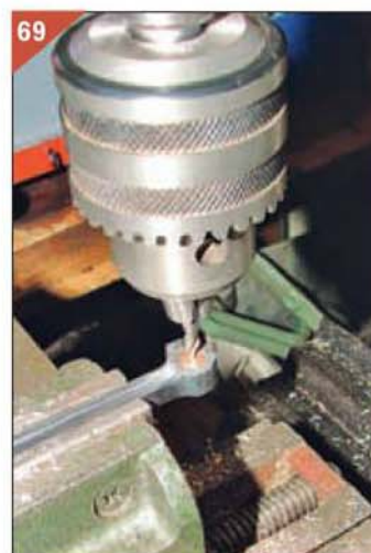
Centre drilling the bushes.
