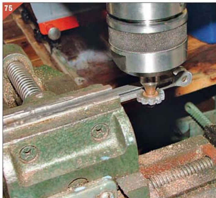
75 Care is needed at the ends of the fluting.
