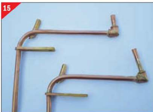
15 The two swan neck brake connections. The stub on the left closes the open end of the brake pipe when not in use.
