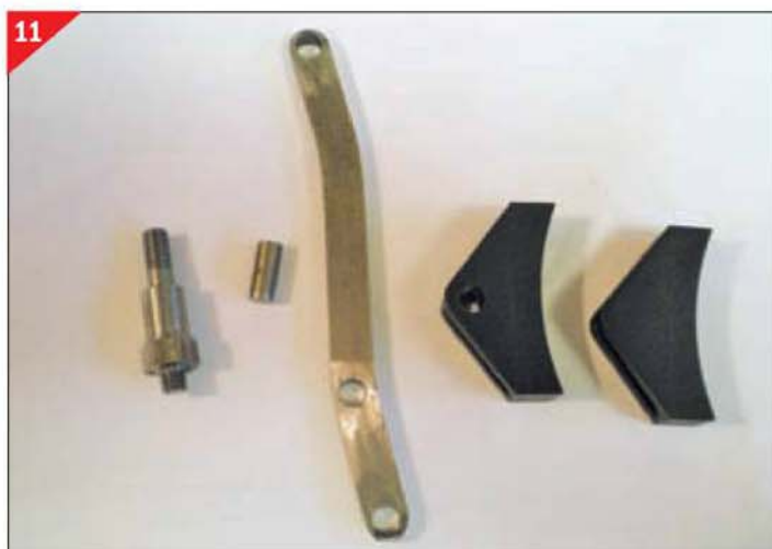
11 The components that make up one brake shoe assembly together with an undrilled shoe.
