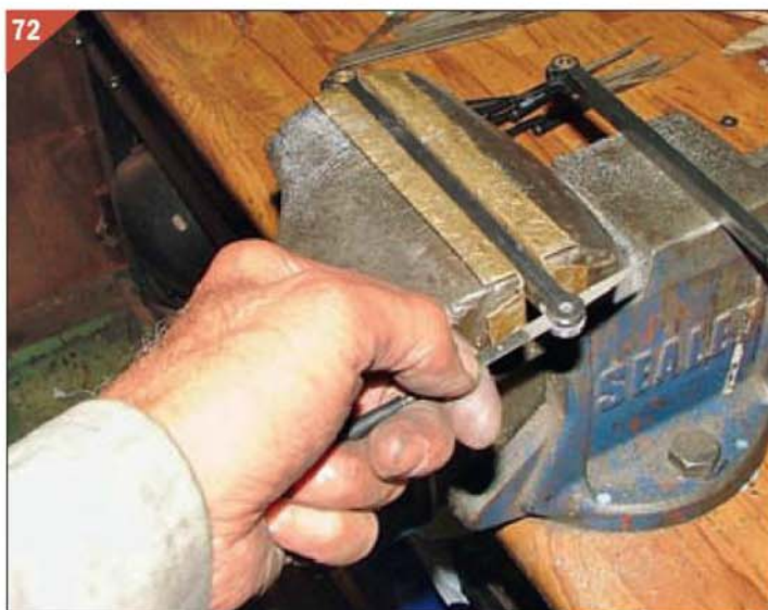
Files are used to tidy up the rough slot.
