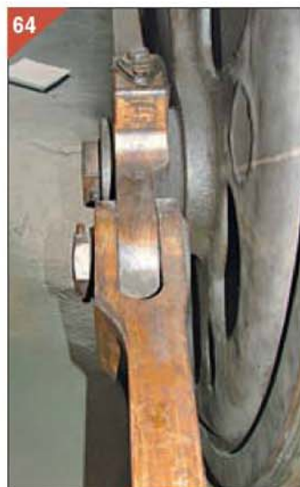
The left centre crankpin at York seen from the rear.
