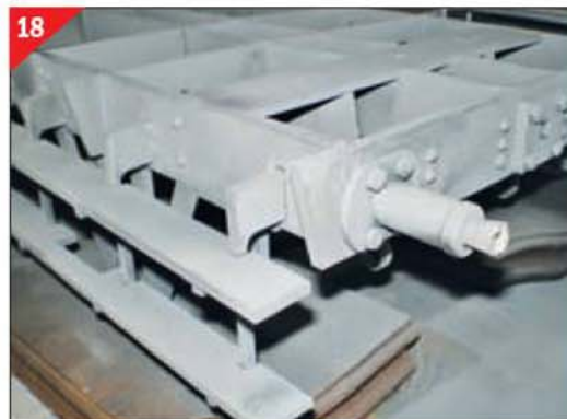
18 The chassis after the second primer coat had been applied.
