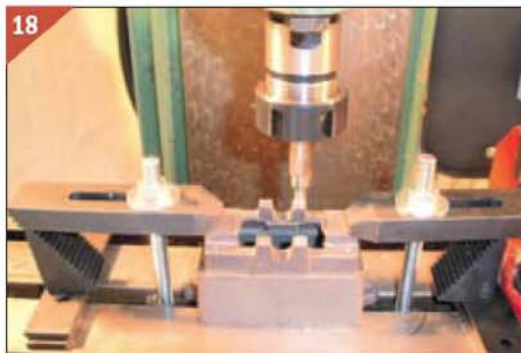
Wobbling up the back of the casting.
