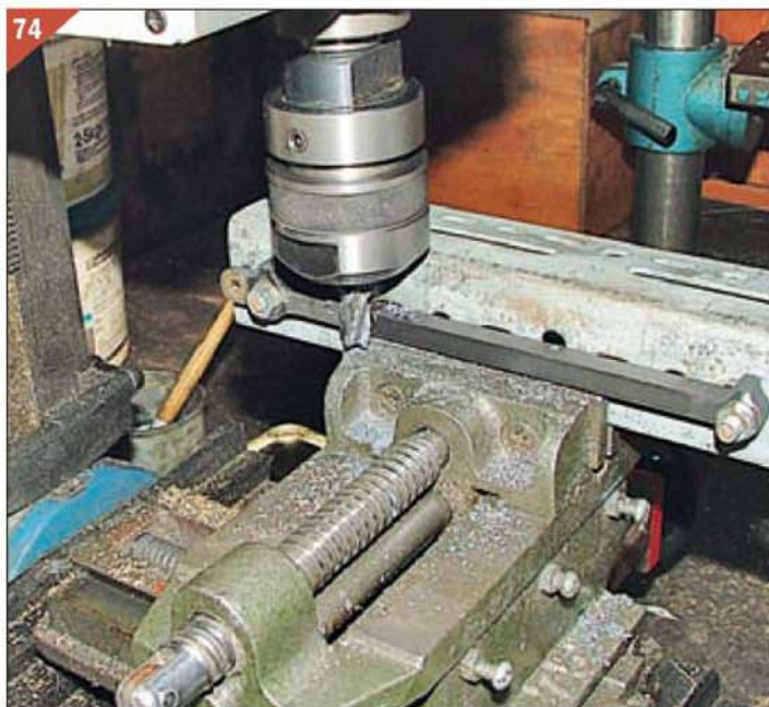
74 Heavy duty Dexion was adequate to hold the rods.
