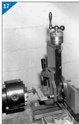
Milling the spoke profile.
