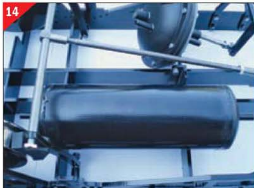
14 The push rod eye, through which is passed the brake cross beams.
