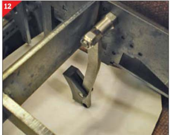
The complete hanger assembly in place, secured with a 6mm Nyloc nut.
