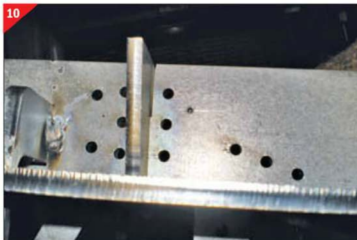
10 This centre punch mark locates the 6mm tapped hole in the frames into which is screwed the brake hanger bracket.
