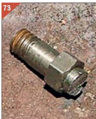
The knuckle joint bolt before silver-soldering.
