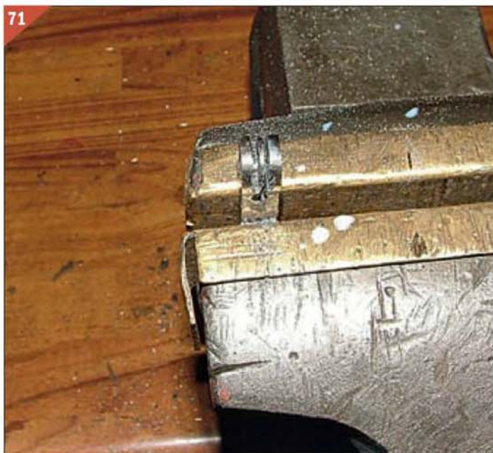
Cutting out the forked end of the rear rods.
