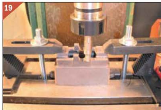
Wobbling the front of the casting.
