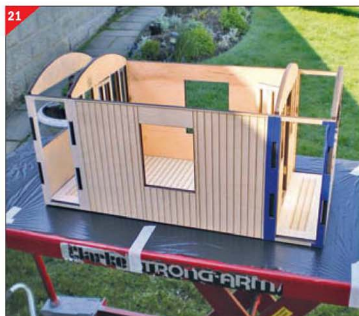
21 The van body assembled for a dry run standing on polythene to catch epoxy drips.
