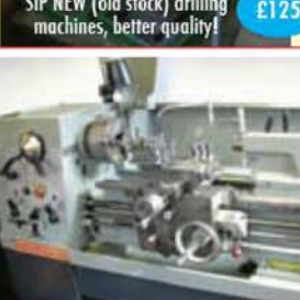
Colchester Student 1800; 6" x 24" + gap bed, 3 & 4 jaw chucks + 240 volts!
