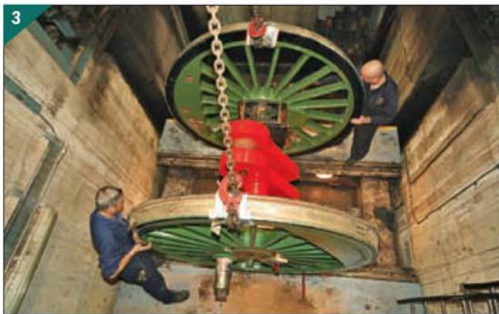
Flying Scotsman's centre driving set is examined in the NRM's wheel drop pit. (Photo: NRM)
