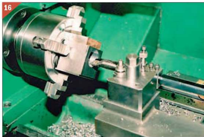
Boring the column top block.
