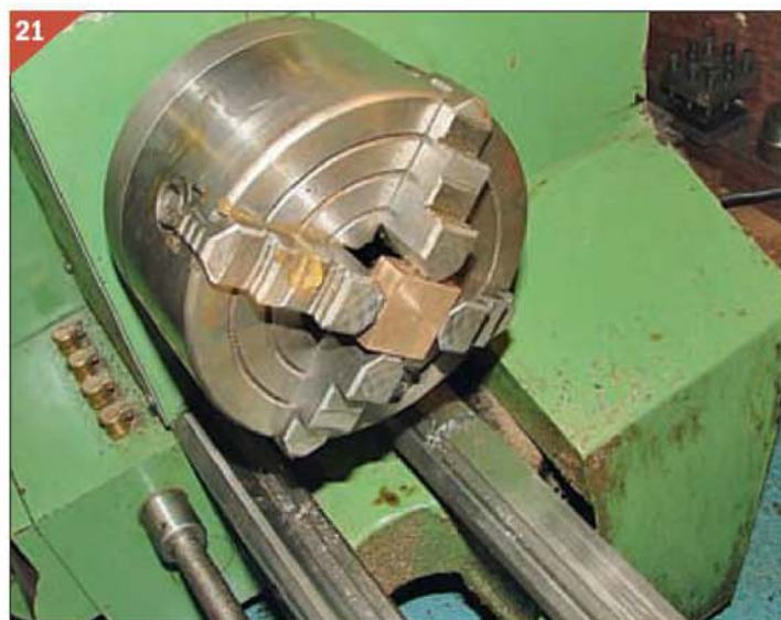
The axlebox material is set up in the 4-jaw with the punch mark central.
