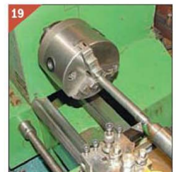
An axle is set up in the 3-jaw and machined at the tailstock end. A dead centre is used or live centre if you have one.
