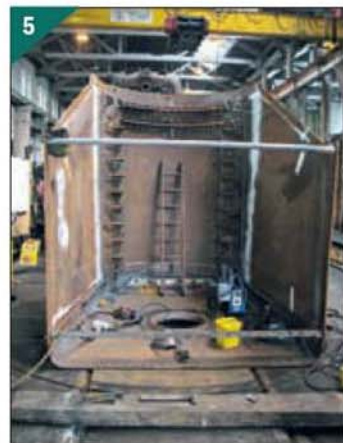
The backhead and sides of the outer firebox during a break in work at Riley & Son's works at Buckley Wells, Bury. (Photo: K. Williams)
