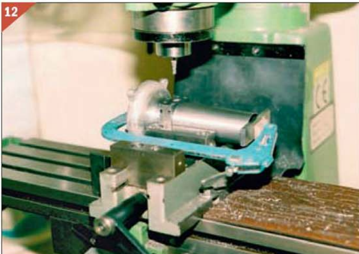
Milling the slot.
