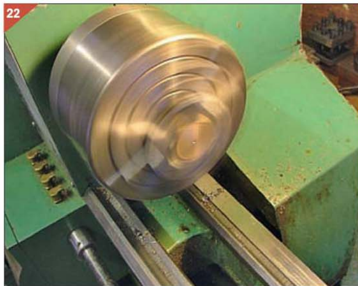
With the lathe running the punch mark must be static.
