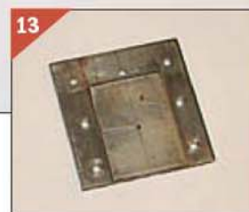
This is the centre finder and drilling jig. Remember not to drill the top row of holes for the rear axleboxes. See photo 18.
