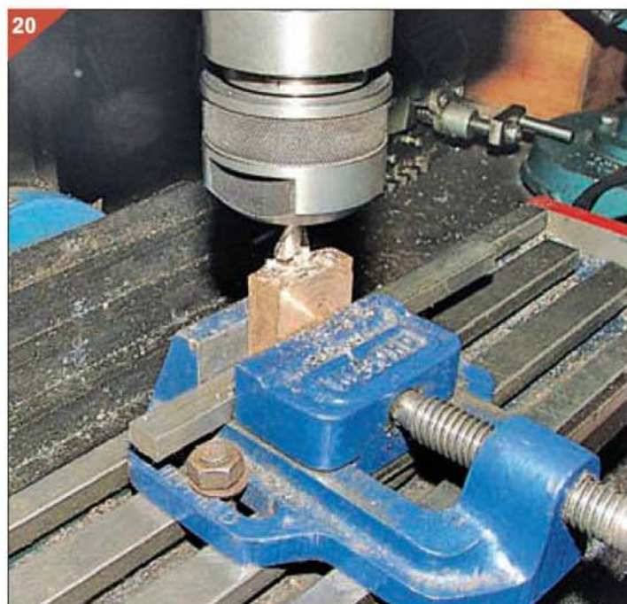
The sawn pieces of bronze for the axles are milled to size in a machine vice bolted to the mill table.
