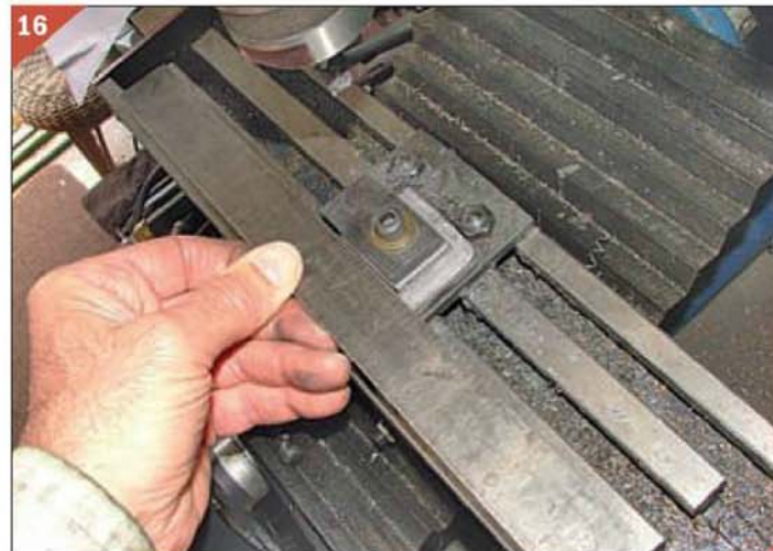
A cast iron horn is set up in the jig on the milling table, ensuring that it is lined up with the axis of the machine. File down the back of the horn to remove any roughness from the casting.
