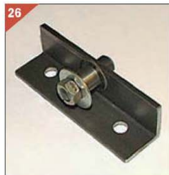
The axlebox jig is a simple assembly used to hold the items at a fixed height on the milling table.
