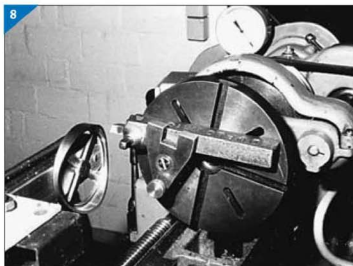
Flycutting the radius on the turntable mounting.
