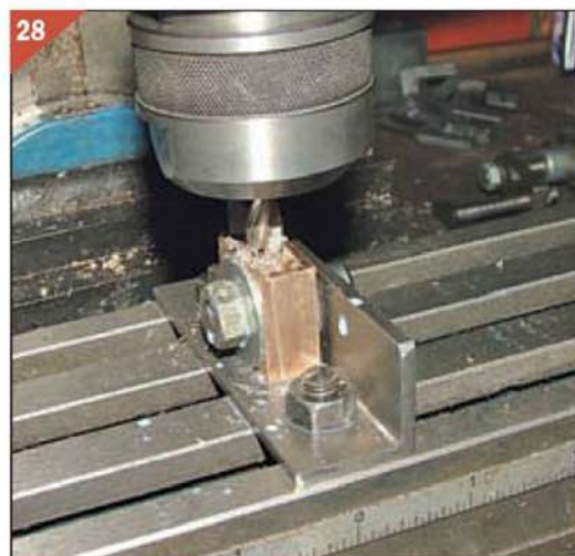
Milling the slot in the axlebox.
