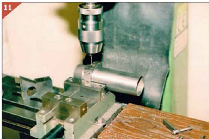
Drilling the bolt holes.
