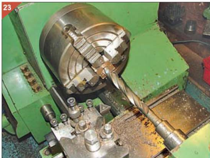
After centre drilling the hole position a large drill can be used in the tailstock. A very small amount of run out is permissible, as the milling jig should correct small errors here, assuming we have made the axlebox slightly oversize.
