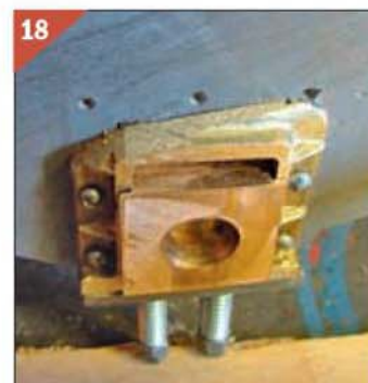
The rear horns need a considerable amount removed to clear the base of the firebox. Note the row of holes drilled by mistake. Another rivet was added later to the reduced top section of flange.
