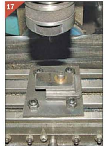
The jig is easily made from 6mm steel plate. The top plate used to clamp the horn in place is made the same width as the frame slot and can be used as a visual guide for the cutter.
