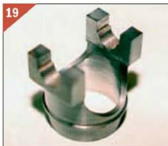
The machined column top.
