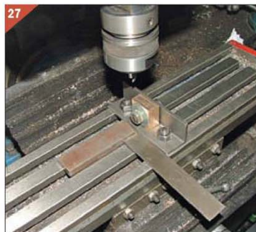
The milling jig is set up on the mill table to ensure it is square.
