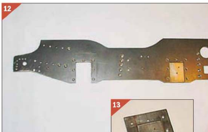
The left frame with the centre finder in position. I have marked out the centre line of the cylinders and from this the fixing holes can be positioned.
