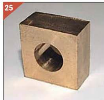
A finished reamed axlebox blank.
