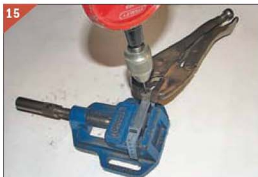
Drill and tap one set of holes in the motion plate and then bolt and clamp the trunnion brackets in position. Use a hand brace or battery drill to spot drill the position of the second holes using a clearance drill. This will stop the tapping drill wandering on the hard surface of the laser cut plate.
