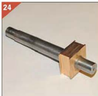
The axlebox has now been reamed to a close fit on the axle.
