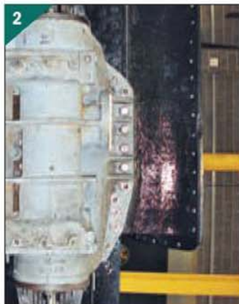
The replacement right-hand cylinder from A3 No. 60041 Salmon Trout after re-drilling and fitting to No. 4472. (Photo: Gary Boyd-Hope/SR)
