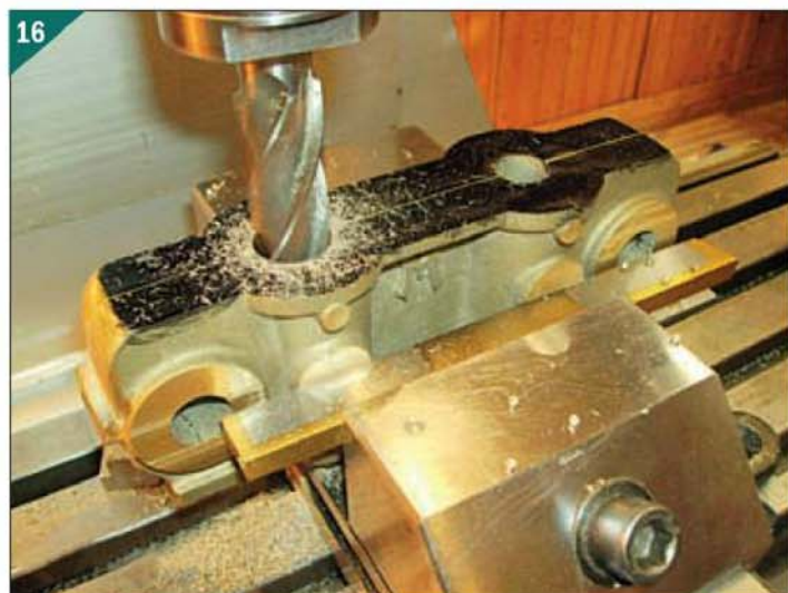
Opening out the cylinder bores.
