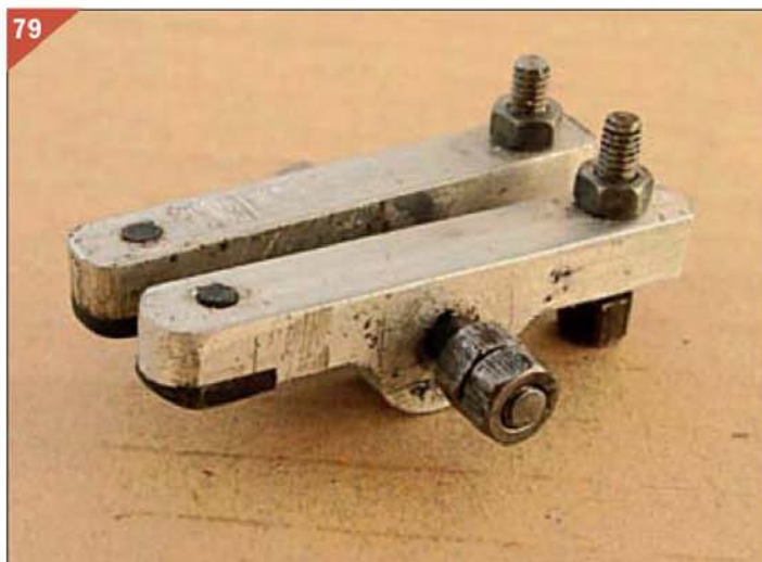
Two rocker arms fitted to shaft.
