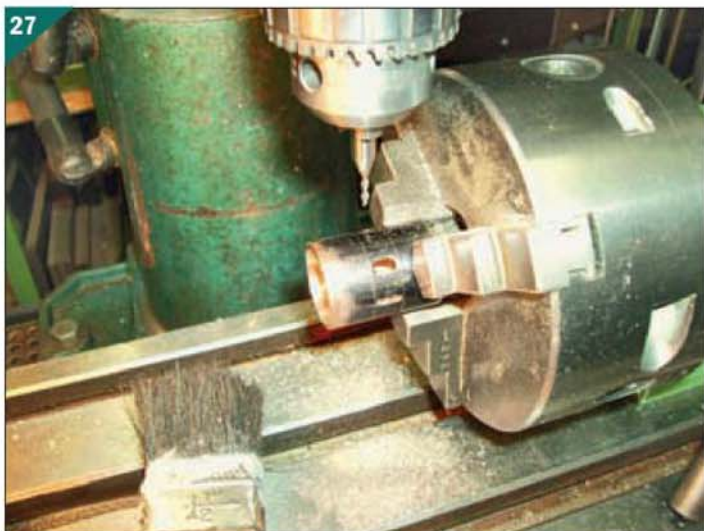
27 Drilling the valve bushings.
