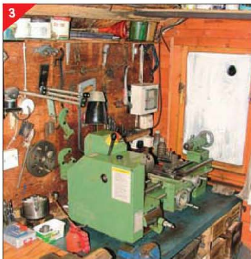
The Warco 918 lathe is mounted on a steel engineer's bench. When the removal men tried to move this bench they thought it was still bolted to the floor as it's so heavy! More racking or shelving for lathe tools would be an advantage.
