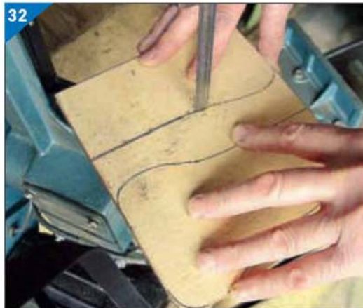
Cutting the firebox templates.
