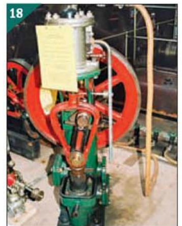
Joseph Evans vertical ram pump of 1951 with reversing eccentric.
