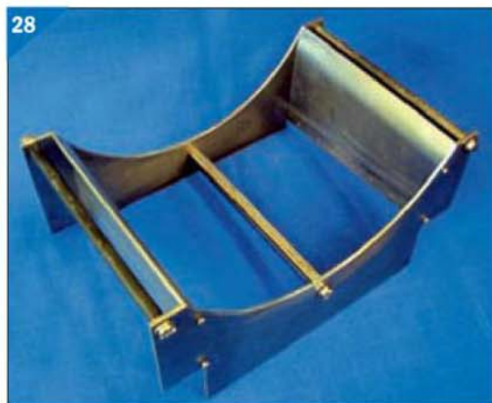
Fabricating the smokebox saddle.
