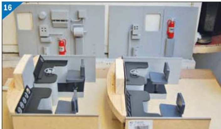
The cab interior parts ready to be fitted to the model. Dolls house fittings used for seating and fire extinguishers.
