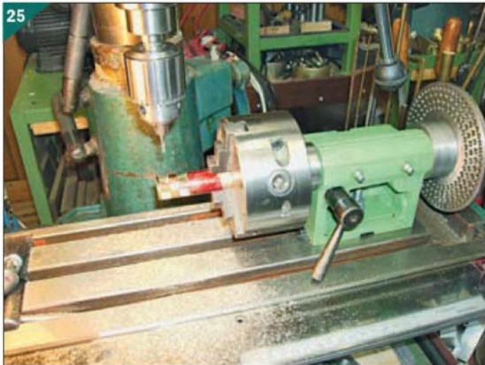
25 Making the rotary spool valves.
