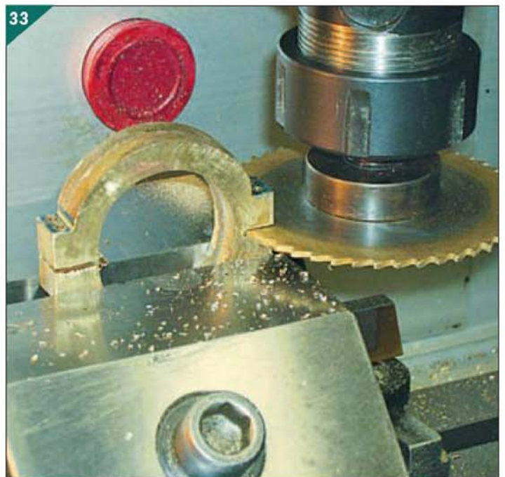
Cutting the eccentric straps in half.
