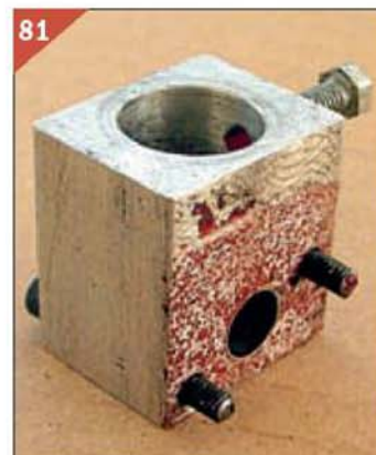
The inlet elbow, even mottling of Hermetite confirms flatness of mating faces.
