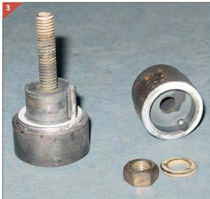
A small gapping jig.
