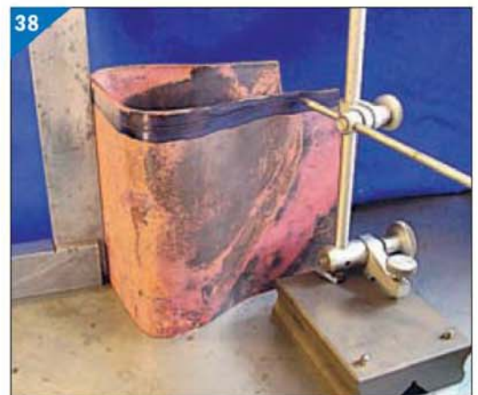
Marking out the firebox.
