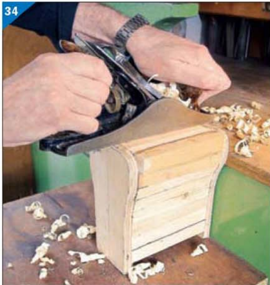
Shaping the top firebox former profile.
