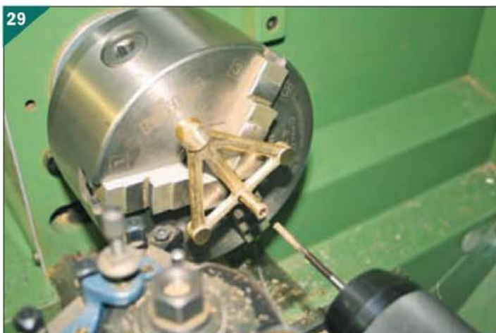
29 The triangle is turned and faced then drilled ready for reaming.
