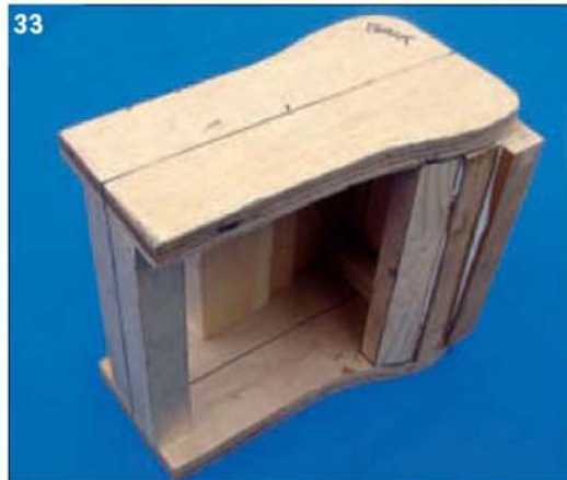
Making the firebox former.
