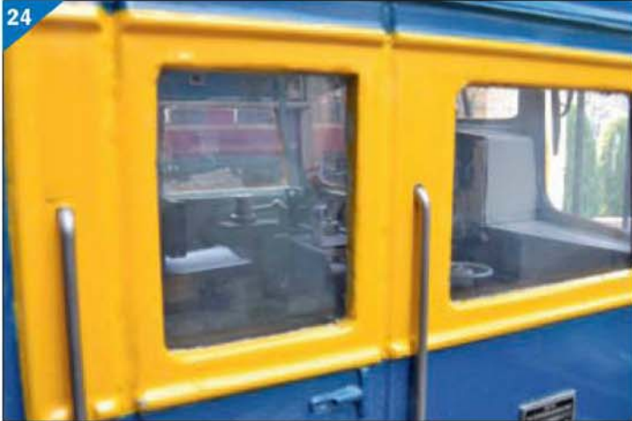
The view of the cab with windows fitted. The final aluminium upper dash panels can be clearly seen.
