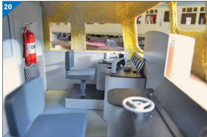
20 All dashboard units in place and only the front aluminium panels are required to complete the cab.
