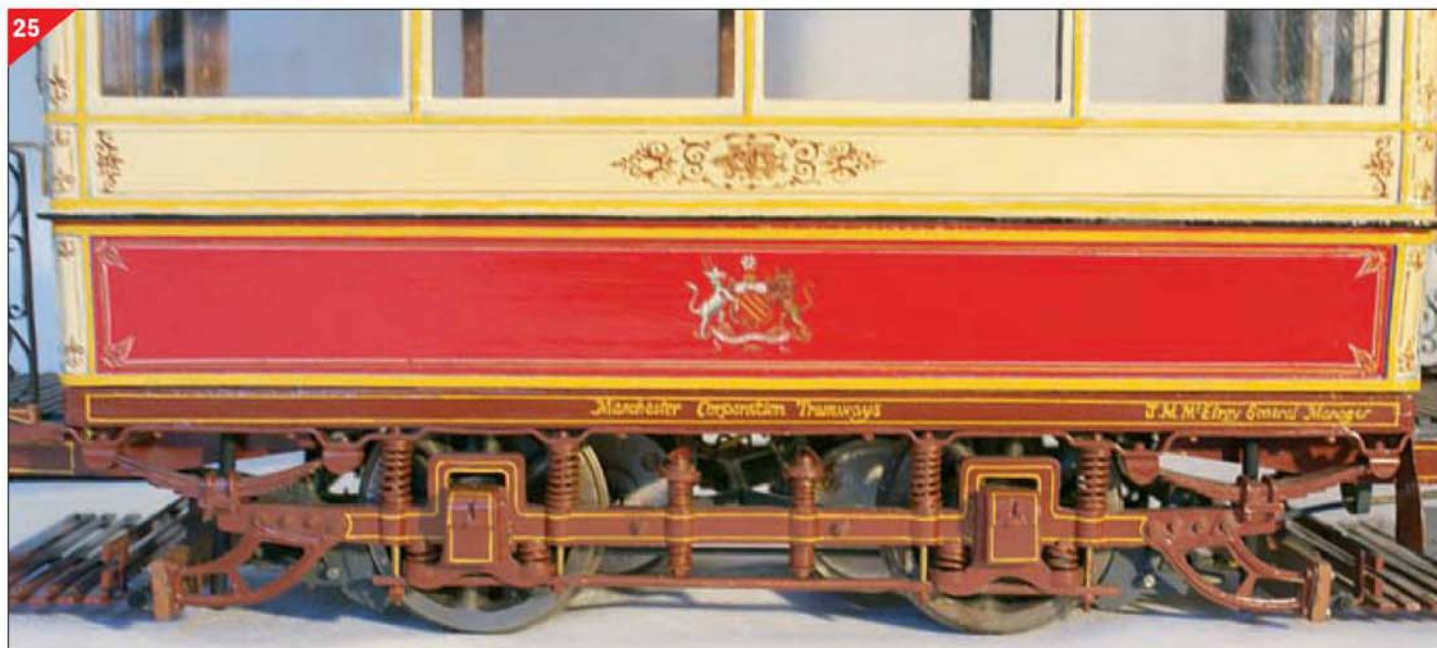
Early style Brill 21E truck with narrow axle boxes.
