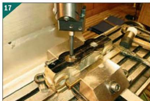
Machining a cylinder bore.
