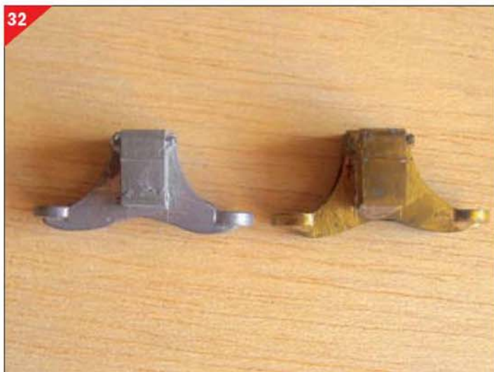
Wide wing axlebox casting and pattern.
