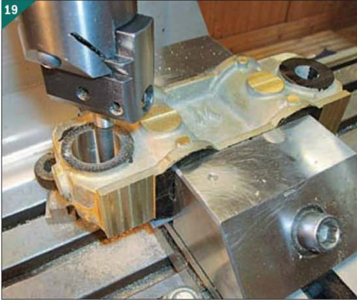
19 Boring a rotary valve hole.
