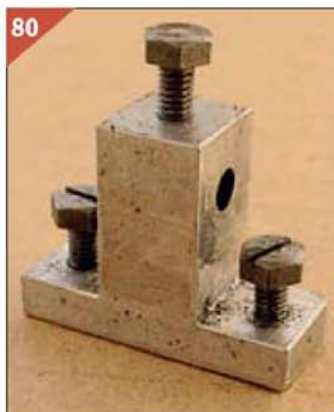
Rocker post shown with its attachment screws and the shaft clamping screw.
