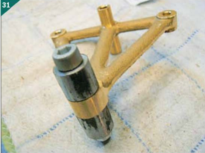
Using a filing jig to finish the radii.
