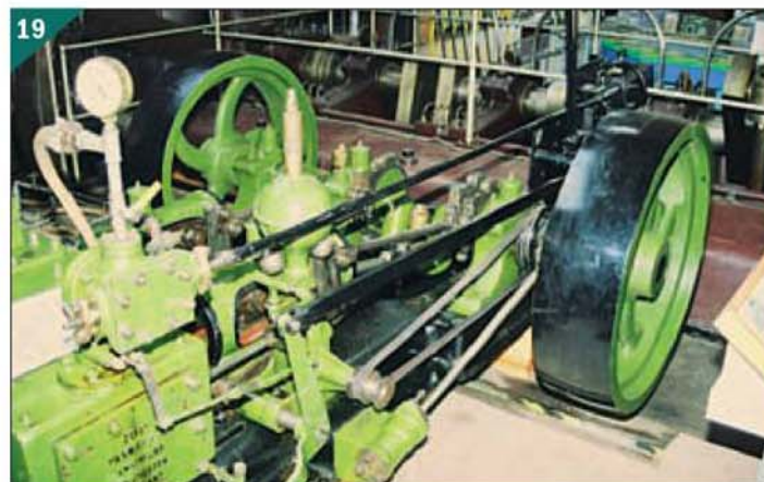
Davey Paxman horizontal compounds made in Colchester 1892. It once drove a dredger on Lake Zurich.
