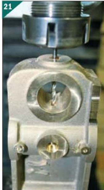
21 Drilling a steam passage.
