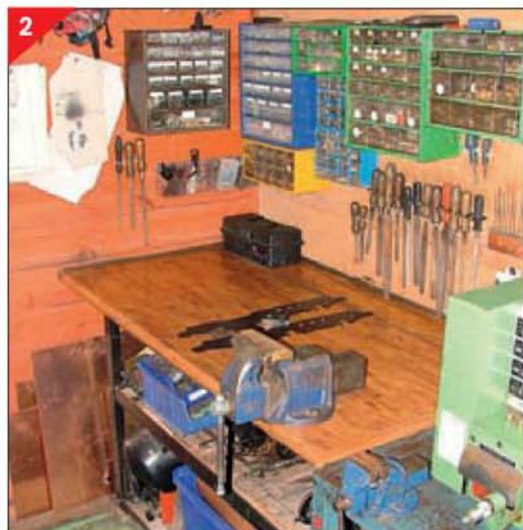
The main workbench is recycled kitchen worktop supported on 50 x 50 steel angle. Up to three 3½in. gauge tender locomotives can be stored on the shelf under the bench, with further storage underneath. Maximum bench space is preserved by having as much as possible fixed to the walls.
