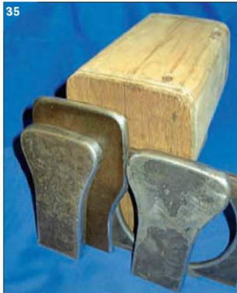
The completed former and some flanging plates.
