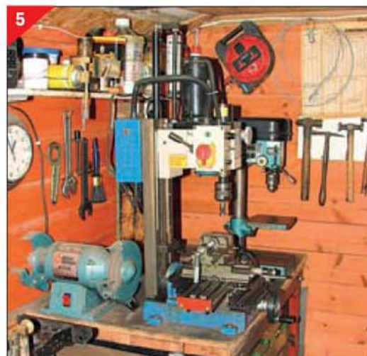
The Chester Mini-mill and Clarke ½in. pillar drill are mounted on a homemade steel-framed bench quite close together. The space underneath houses a three-drawer tool chest containing all the hand tools not attached to the walls. Taps, dies, spanners, punches, etc.
