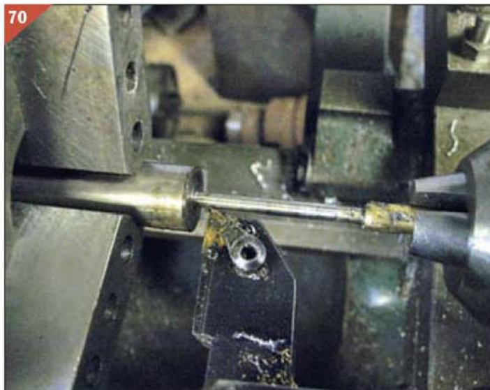
Turning valve using female centre to steady.
