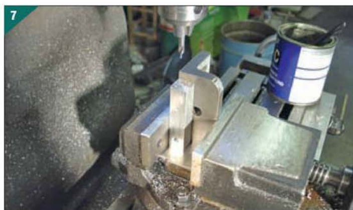
The setup for centre drilling the valve port positions.
