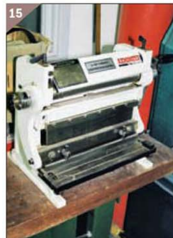
15 Bending machine - used in making boxes and caskets.
