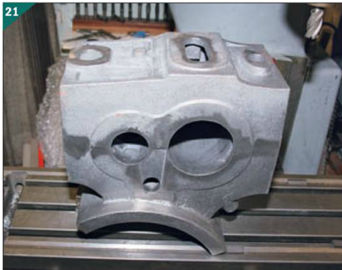
Around the back are the two cylinder bores, high and low pressure, below the HP bore is the cored hole for the LP exhaust.
