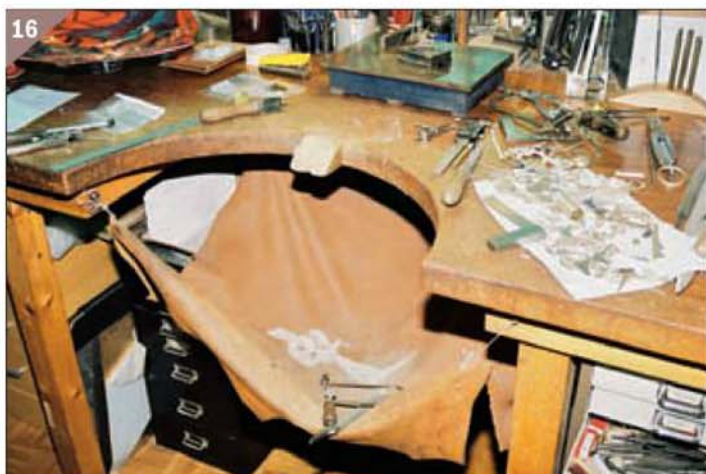
16 Gold and silversmith's workbench - the apron catches filings and scrap for recycling.
