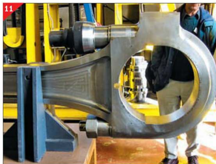
The massive big end of the inside coupling rod, minus the split bearing.
