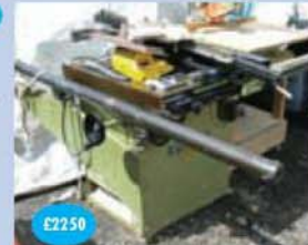
Startrite TA1250 12" full sliding table saw bench (240 volts)
