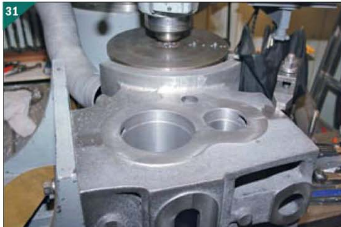
Fly cutting the underneath of the cylinder.
