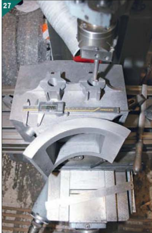
27 The cylinder is resting on the machined back face and is set axial to the table so one of the gland bores may be completed and the table then indexed along to bore the other.
