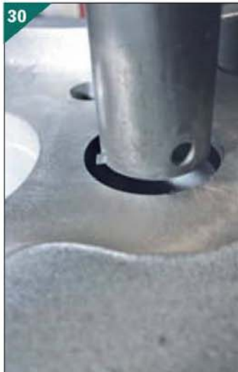
The high pressure bore is machined with as rigid a bar as may be employed, the dti is used to set the tool between cuts.
