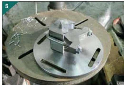
This 'Keats' type angle plate from Myford is a good way to hold this kind of stock.
