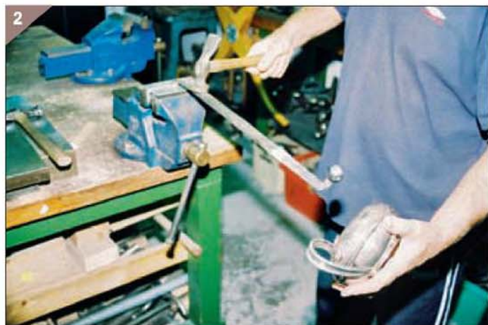
One of many unusual tools - a snarling iron used to hammer inside a raised piece.
