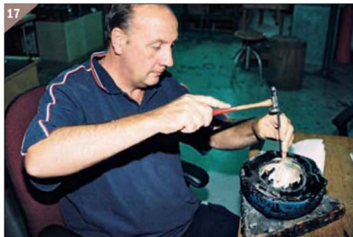
17 Steve Wager chasing a piece on a pitch block.
