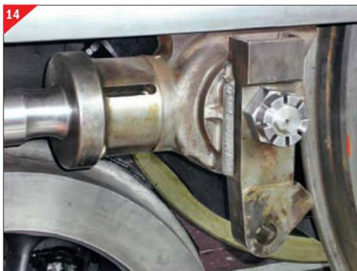
The left-hand cast steel crosshead with welded drop arm.
