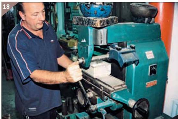
18 Gapping machine - similar to a milling machine.
