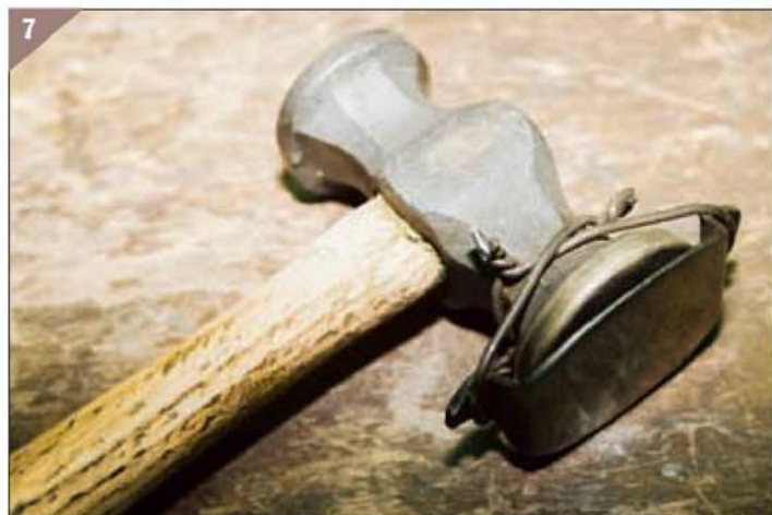
'Italian shoe' planishing hammer for flat work.
