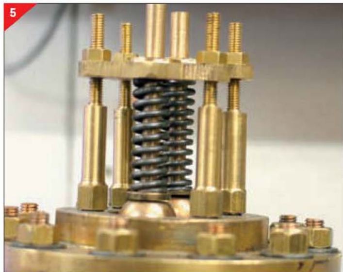
The safety valves.
