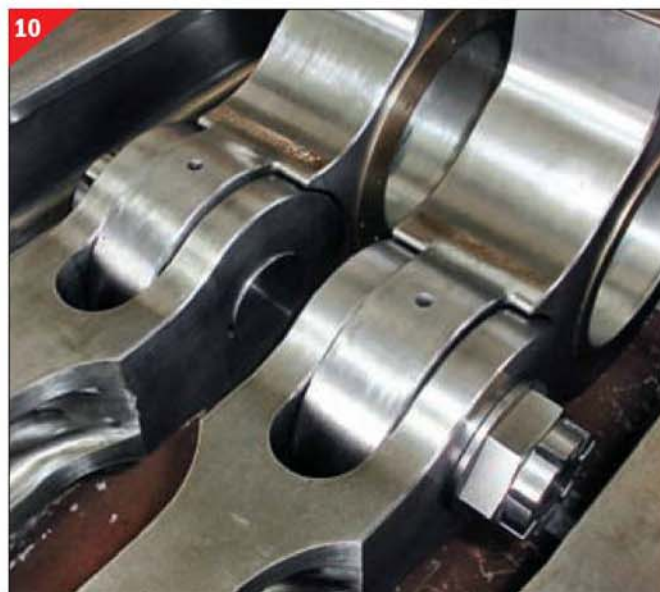
Knuckle joints on the coupling rods - sculpture in steel.
