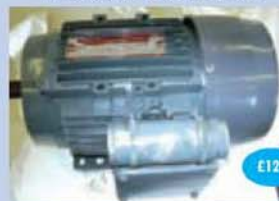
Crompton Parkinson Foot Mounted 2HP 240V / single phase 1400 revs as new.
