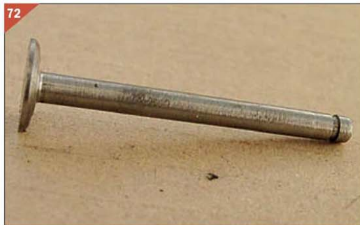
Groove is clearly visible on valve stem.
