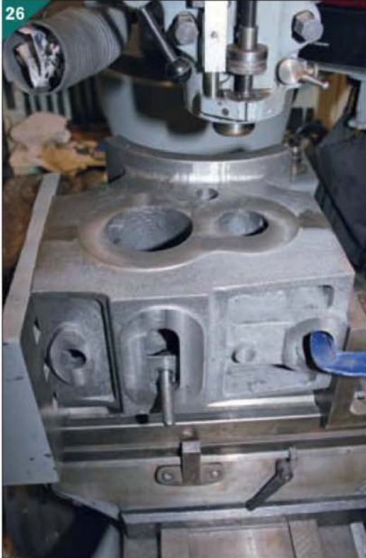
26 The back of the cylinder where the cover fits is machined. Note again that two angle plates are used for maximum rigidity. Note the stud, packer and nut still in the regulator chest from previously holding this face to an angle plate to ensure verticality.
