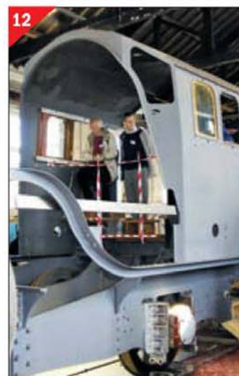
The cab structure in place.
