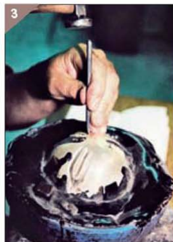
Chasing a piece on a pitch block.
