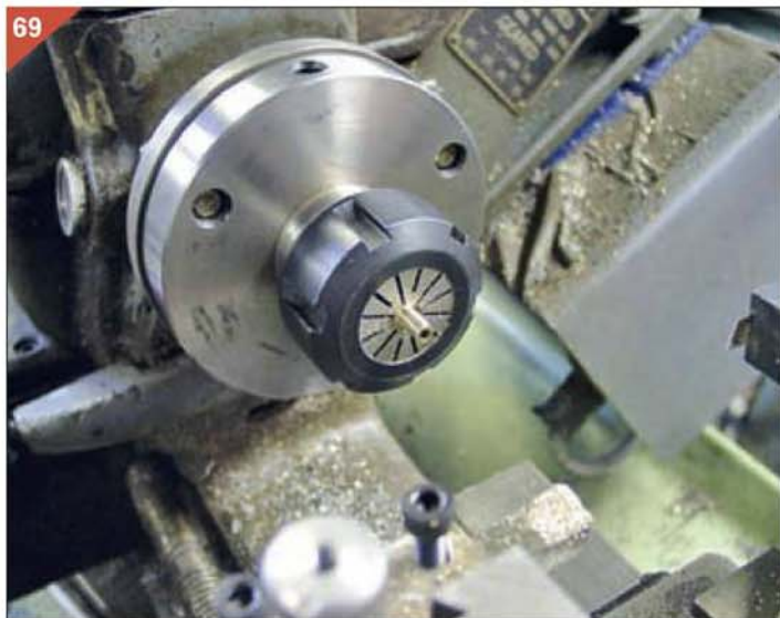
An ER collet chuck was used to turn the valve guides.
