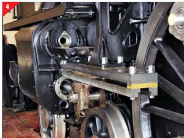
Left-hand outside cylinder and slide bar assembly.
