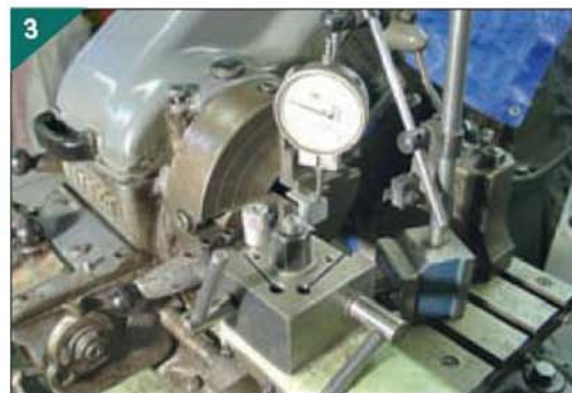
Using a 'clock' to centre the work in the 4-jaw chuck.
