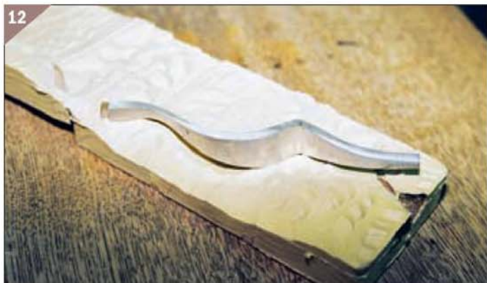
12 Silver casting in Plaster of Paris mould.
