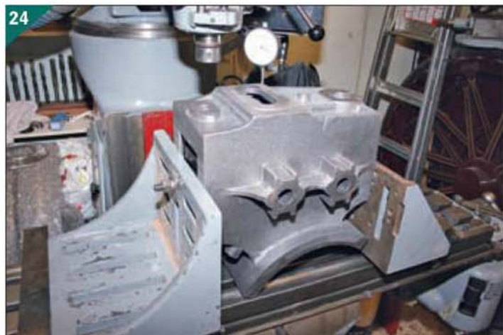
The cylinder is returned the right way up and held between two angle plates. Note the dti to establish if the top face is horizontal.
