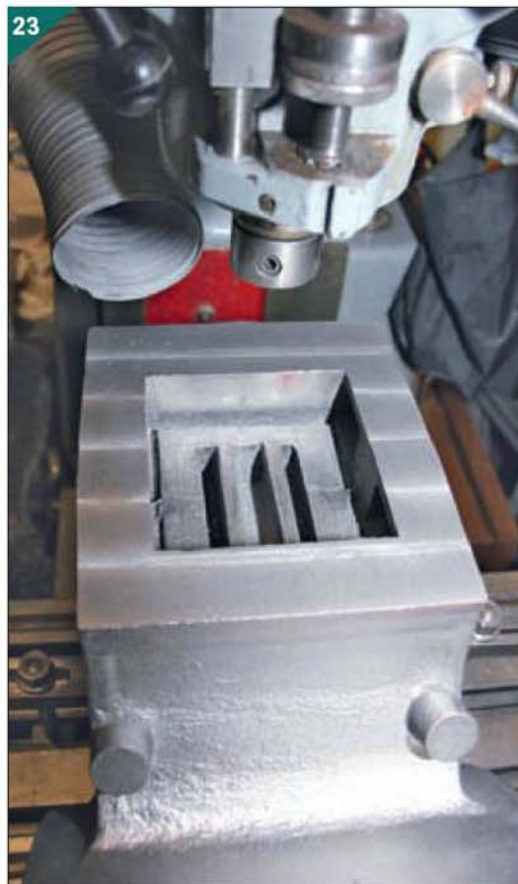
After machining the HP face the cylinder is turned over to machine the LP face. Note the two drain cock bosses cast under the LP bore.
