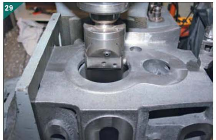
29 The low pressure bore is the easy one as both the boring head and quill will fit down the bore.
