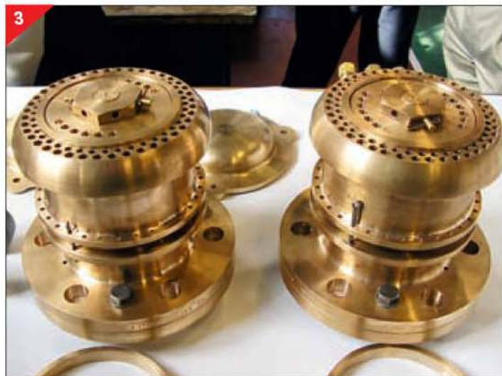
The beautifully finished safety valves.
