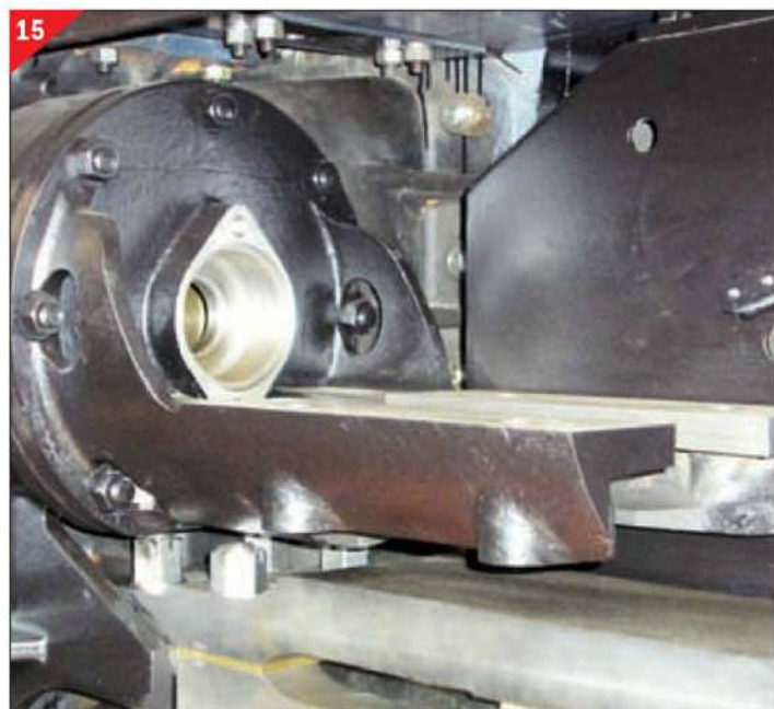
The left-hand valve rod guide casting, bolted to the cylinder block.
