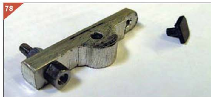
Parts of the rocker assembly, clearly a bit of tidying still needed.
