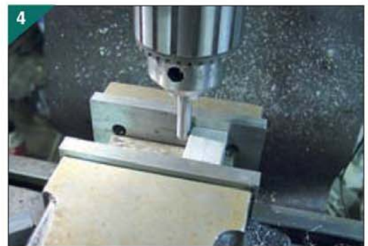
A piece of rectangular material is set against the rod to set a second axis datum.
