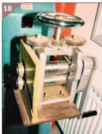
10 Roller for forming silver shapes.
