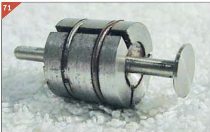
Split collet used to hold valve for later operations.
