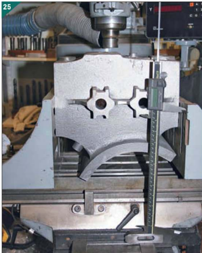
Checking that the cylinders centres are horizontal. Measurements were taken from the top and bottom of the slide bar registers and the cored gland holes.
