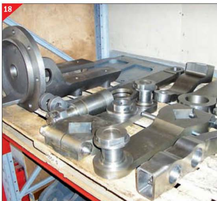
Bits and pieces of valve gear awaiting assembly. Just like a model, only bigger - and a lot heavier!
