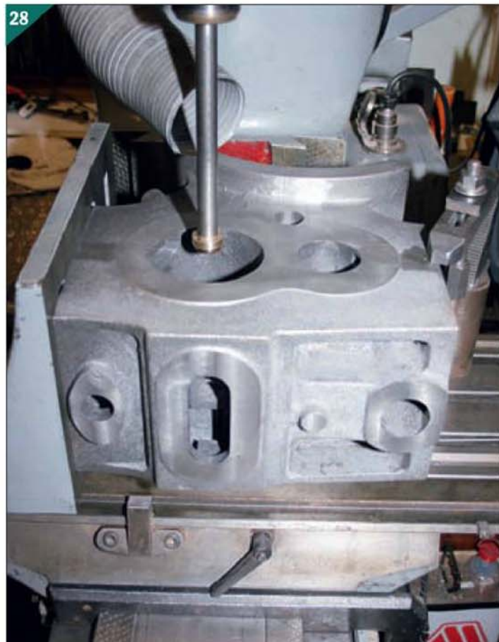
28 The extended tooling to 'pick up' the machined holes at the bottom of the bores.
