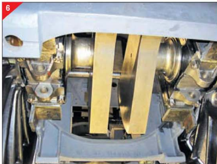
The centre coupled axle from below, showing the massive crank webs. Note the lower hornblocks with axlebox keep pins removed.
