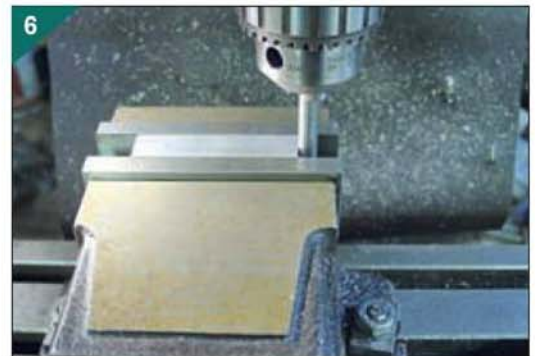
Pillar is pushed against rod then gripped.
