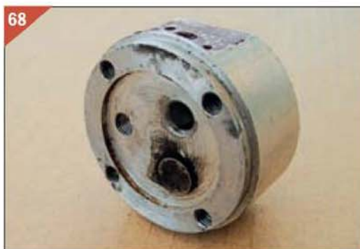
Detail of combustion chamber (exhaust valve in place).
