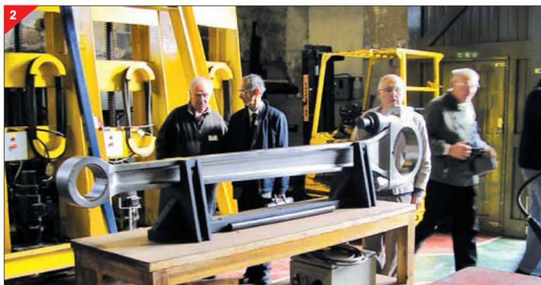
The inside connecting rod fully machined but without bearings.
