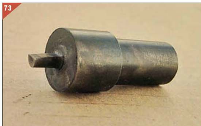
Purpose made D bit to cut recess in valve cap.
