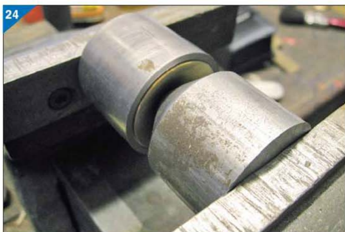
Pressing the vent cap blank in vice.
