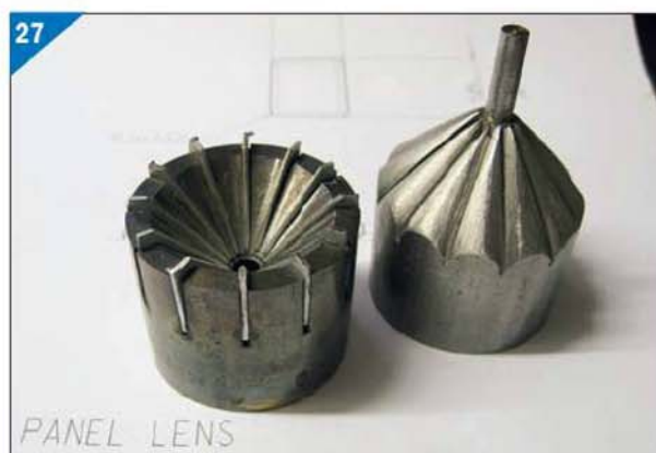
Flutes in punch and die filed to shape.
