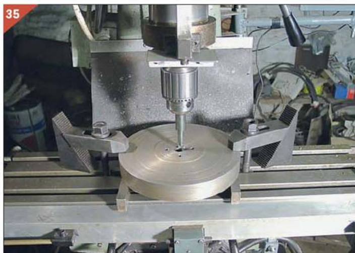
Cutting keyway in flywheel.
