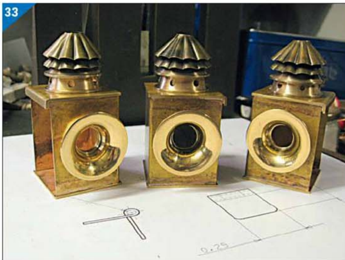
Lamp bodies, vents and lamp hoods temporarily assembled.
