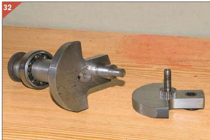
Web is keyed to main shaft by screw driven along the interface.
