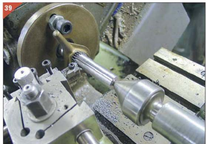
Slave shaft mounted between centres to turn bearing location diameter.
