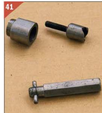
Crank driver dog and ignition cam.
