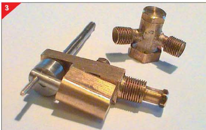
A LBSC type oil pump feed banjo fitting showing the Goodall valve.
