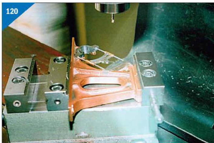
Slide bar support fixed to the side frame ready for machining to form two separate lugs.
