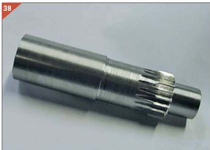
Slave shaft after cutting gear teeth.
