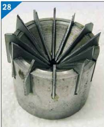
Radial blades 'Loctited' into die.
