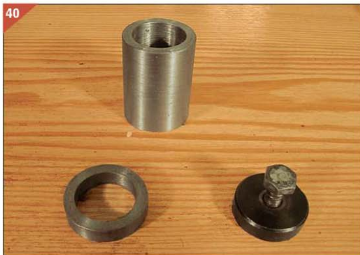
Shaft spacers with flywheel bolt and washer.
