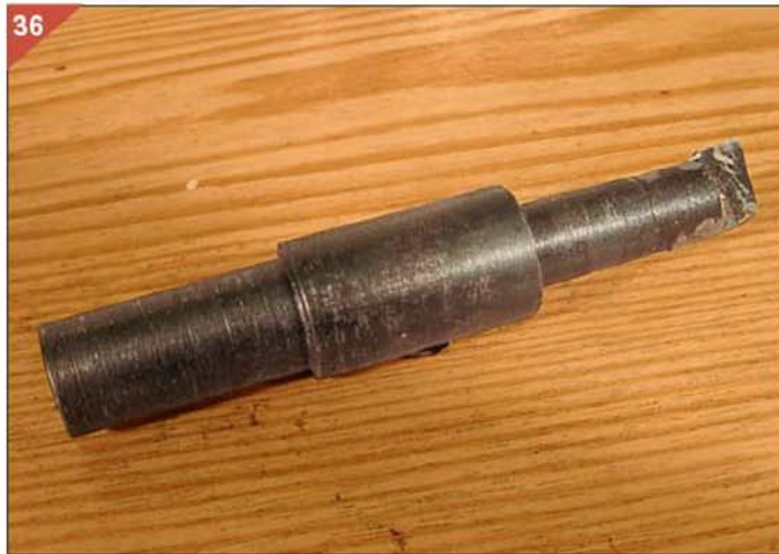
Cutter used for internal keyway.
