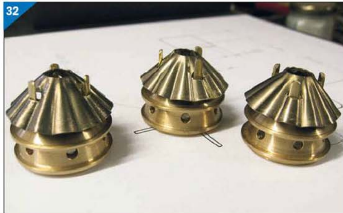
Vent bases and lower caps prior to soft-soldering.
