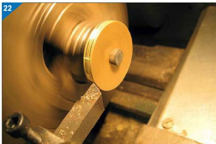
Turning vent cap blanks.
