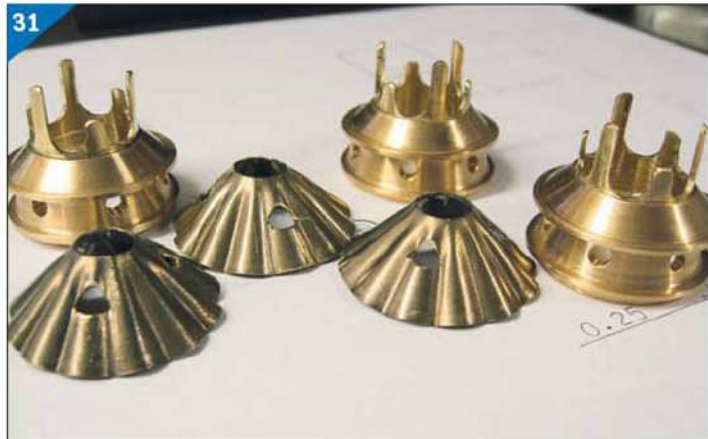
Vent bases and caps prior to assembly.
