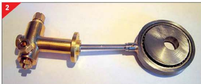
The assembled axle-driven feed pump.
