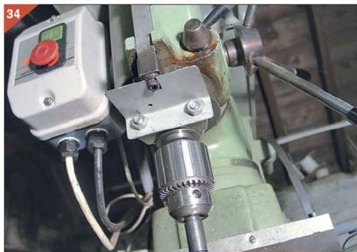
Mill spindle lock arrangement for cutting internal keyway.
