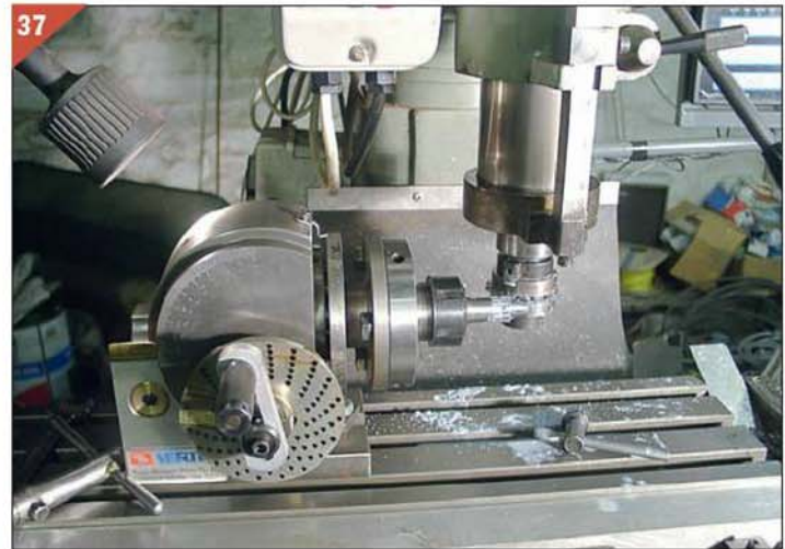
Set up for cutting gear teeth.
