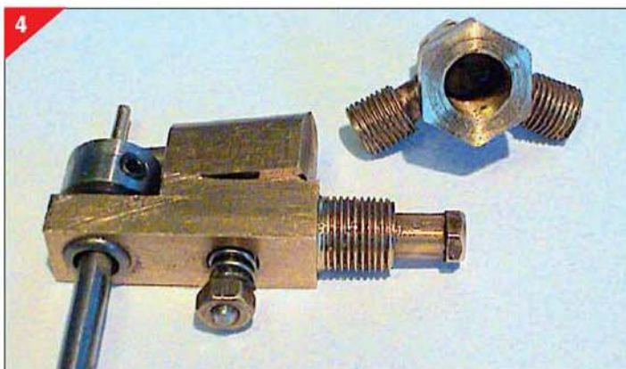
Another view of the LBSC type feed pump.
