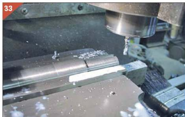
Milling key in shaft for flywheel.
