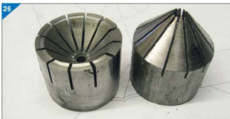
Radial slots cut in punch and die.
