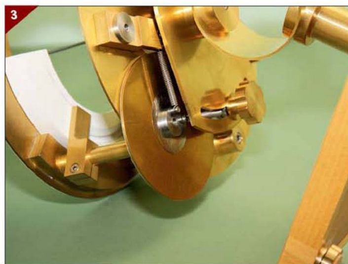
Underside view showing the EoT cam and the thumbscrew for longitude adjustment.
