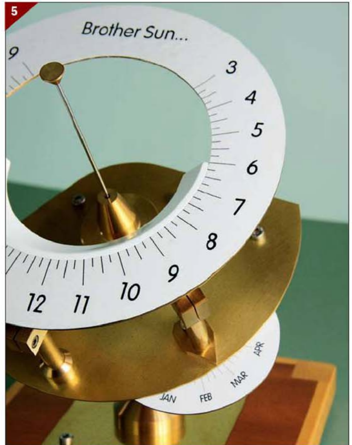
Month dial fitted to the EoT cam.
