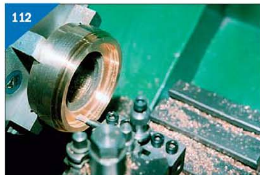
Turning a ring to make the die block and crosshead clamping piece.
