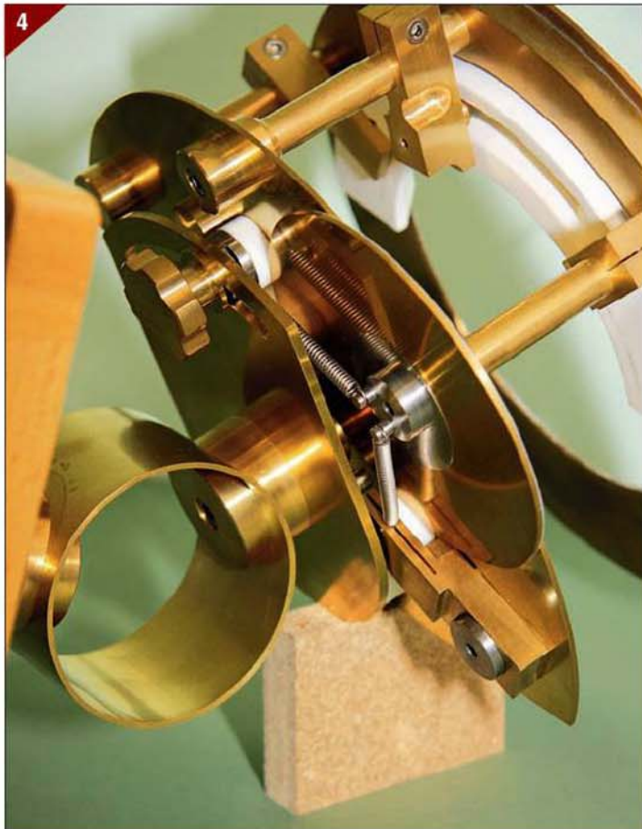
Spring-loaded follower to provide balancing action for the EoT cam.
