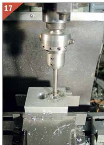
Boring bearing locations for slave shaft and camshaft.
