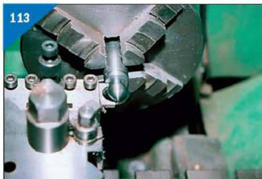
Using a form tool to turn the governor balls.
