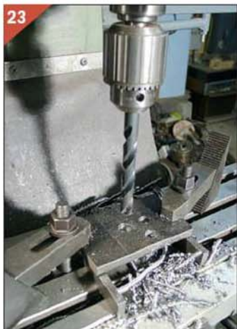
Starting work on the first crank web.
