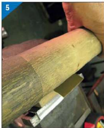
Bending using a wooden roller.
