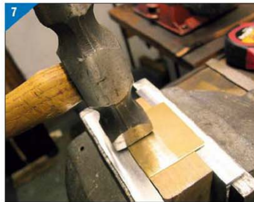
Using a flat-faced hammer to 'sharpen' the bend.
