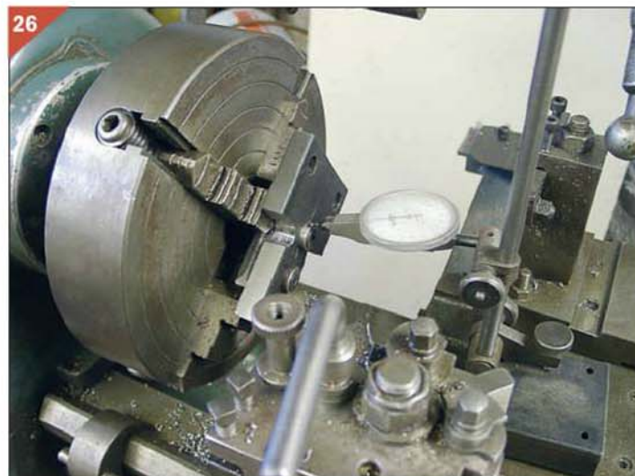
Work is centred by reference to the button.
