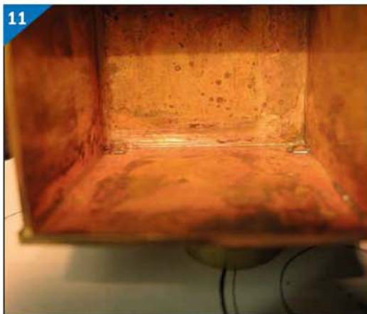
Silver solder joint along inside of seams.
