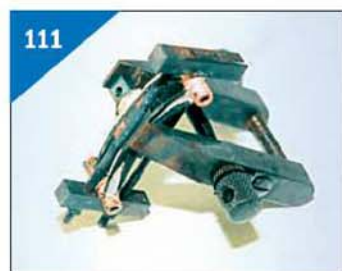
Crosshead after soldering with the clamps still in place.
