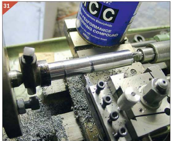
31 Diameter between bearings is slightly reduced to make fitting easier.
