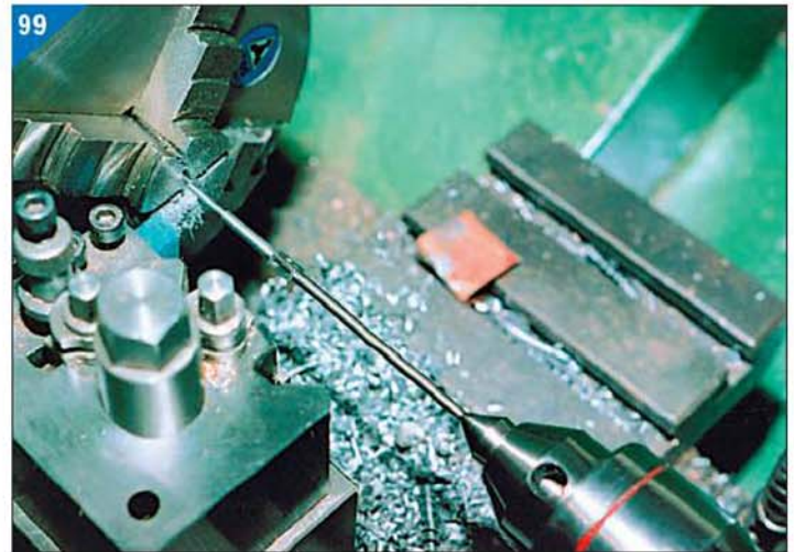
99. Machining the upper pivot of the governor column.
