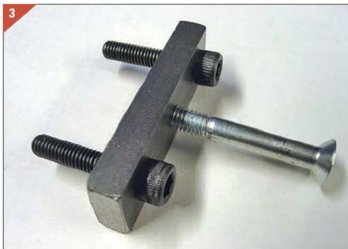
3. Simple puller for flywheel removal.
