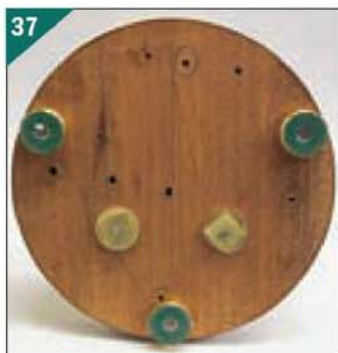
37. Underside of the base with securing nuts and washers.
