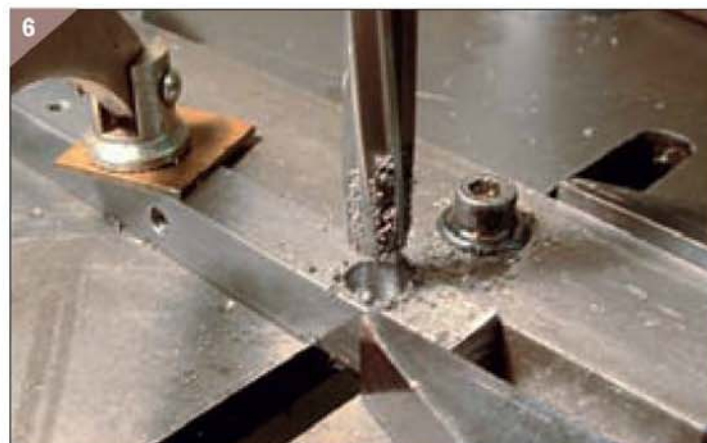
6. Reaming a previously drilled hole for the split cotters.
