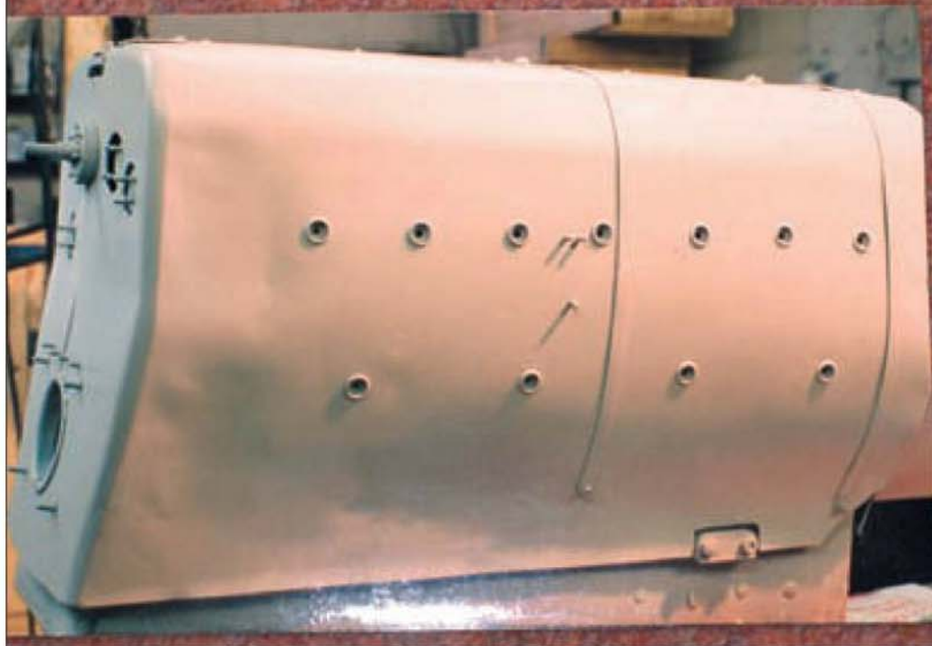
3. Cleating of the firebox side of the King boiler.
