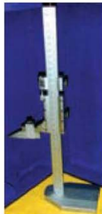
Moore & Wright 12"/300mm Vernier Height Gauge, Matt Chrome Easy to Read Scales, Excellent Condition, Case, £85.00 plus vat.
