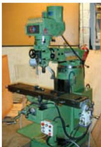
Europa Milltech 2000 Turret Mill, R8 Spindle, Power Feed Table, Tooling, Variable Speed Head, VGC, 3ph, £2750.00 plus vat.
