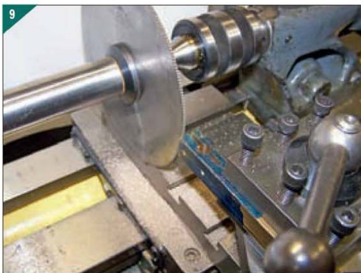
7. Ornamental brass tubing 8. Drilling the letter 'J' holes 9. Making the saw cut in the Myford lathe. 10. Large washers at the base can be formed from off cut pieces of 1/8in. brass. 11. Completed pillars mounted on the finished base taken at a later stage of the construction.
