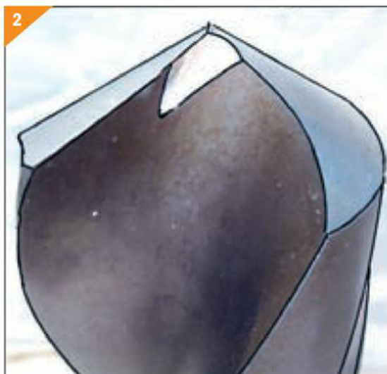
1. Top view of a drill with a thinned web which was done on an off-hand grinder. 2. Side view of the drill showing the comparatively small 'notch' cut on the web to thin it.
