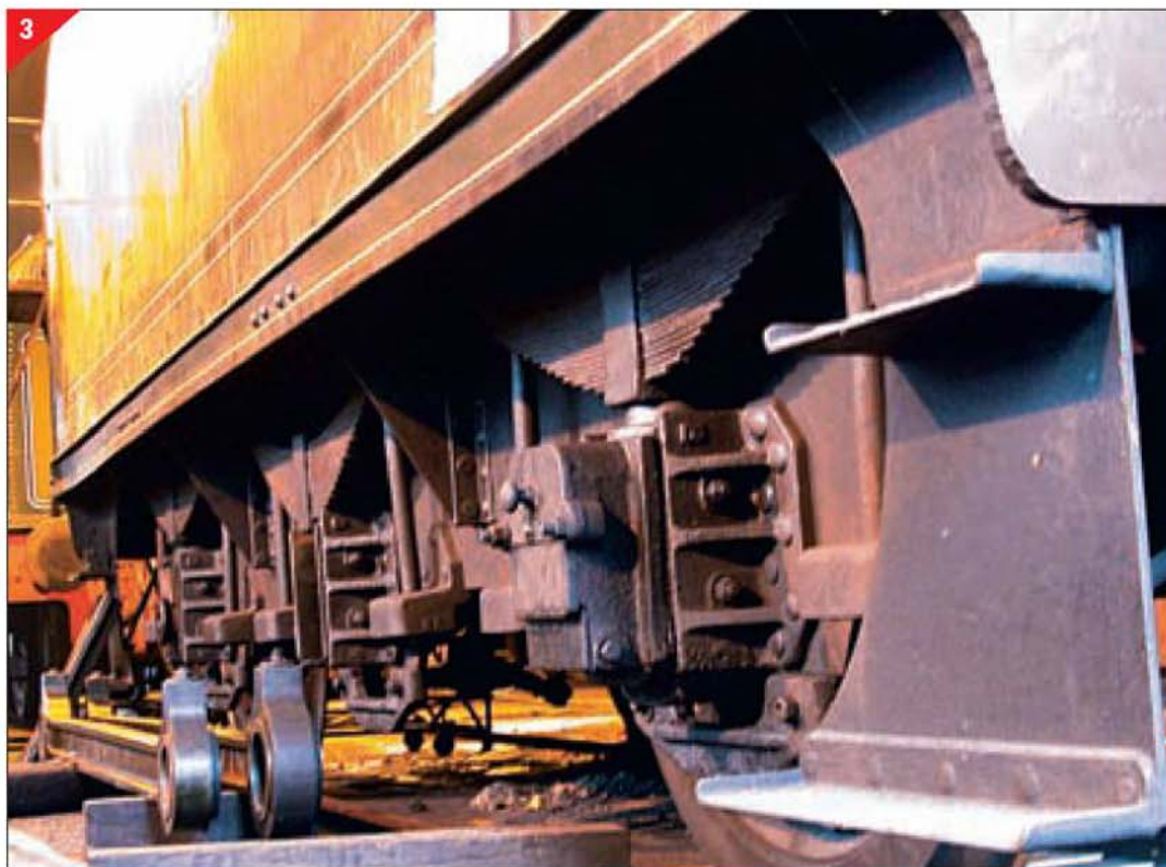
3. View of axleboxes plus a good photograph of the rear steps.
