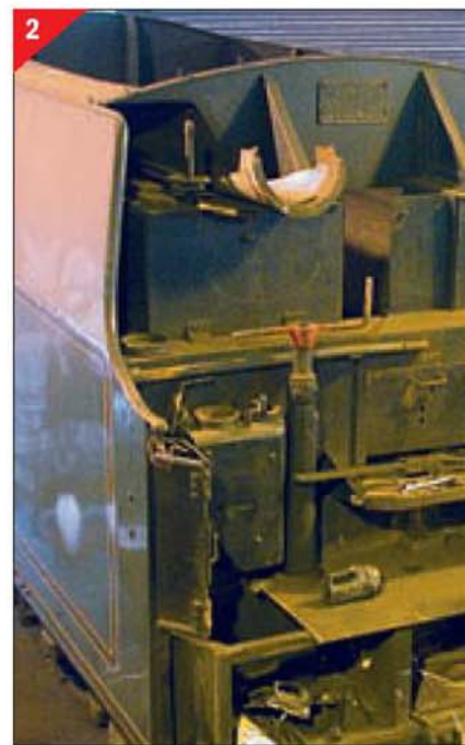
2. Tender front. This is a high-sided tender as fitted to Repton on the North Yorkshire Moors Railway.
