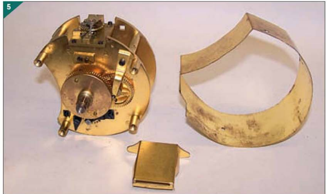
5. Movement after removal from the case with its two dust covers.
