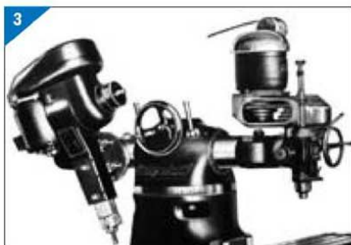
5. The Moog Hydra-point, three axis, numerically-controlled system.
