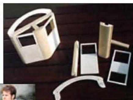
End panel parts for an electric locomotive designed and engineered to be made in wood.
