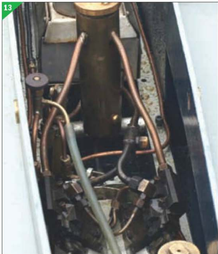
13. The V4 engine in Phil Abbott's flash steamer.
