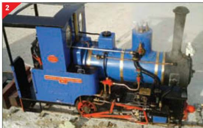
2. An Injector of the author's design fitted to his 5in. gauge Barclay well tank locomotive.
