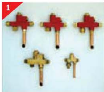
1. A selection of injectors made by the author. Tested and passed ones have been painted; those unfinished await testing and adjustment.
