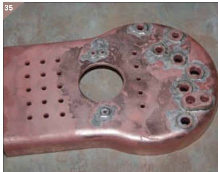
32. Machining the injector bush. 33. Nice solder fillets on outside of blind bushes. 34. Doubtful solder penetration on inside of one bush. 35. Backhead with bushes soldered in place.
