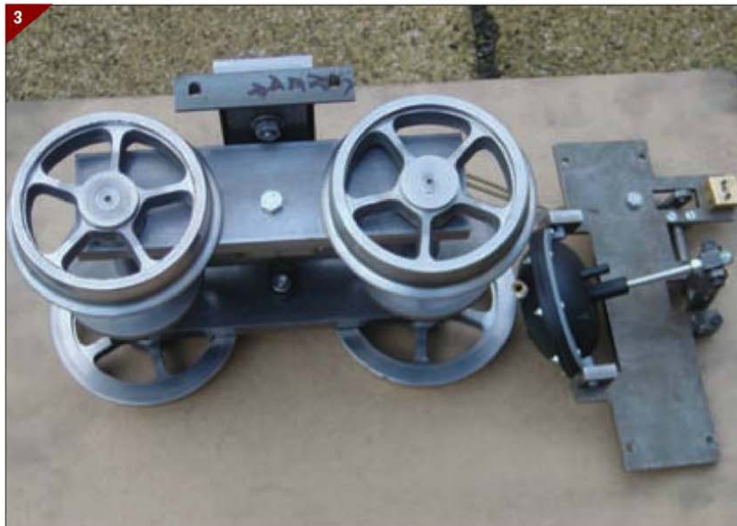
3. Rear bogie from low down on one side; the bolts holding the side frames apart are maintained not tight, to allow bogie equalisation. The inverted brake platform illustrates the smaller anchor, ready for the front Bowden cables.
