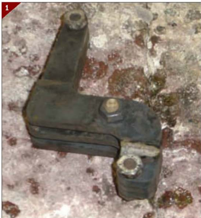
1. Fabricating the brake callipers from three pieces, the middle of the sandwich being a one-piece calliper, whose middle hole is used to locate the holes in the fabricated bridge pieces.
