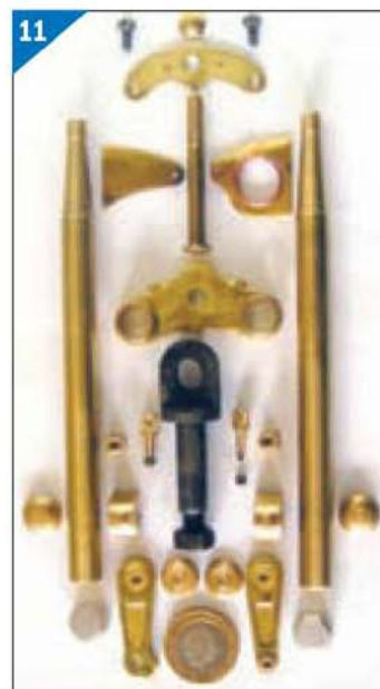
11 shows the various parts together with a full-size reaction link and a £2 coin (28.40mm dia.) for size comparison.
