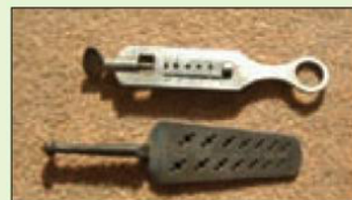
The small tap holder and screw plate sent by John Day.
