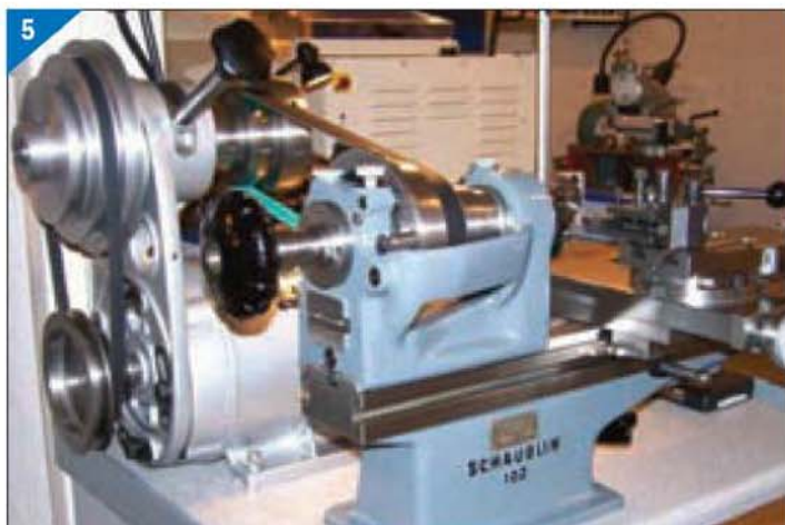
5. 102 Lathe with rear drive and overhung bed.
