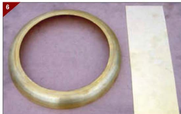
6. A spun bezel and offcut of brass to form the vertical legs.
