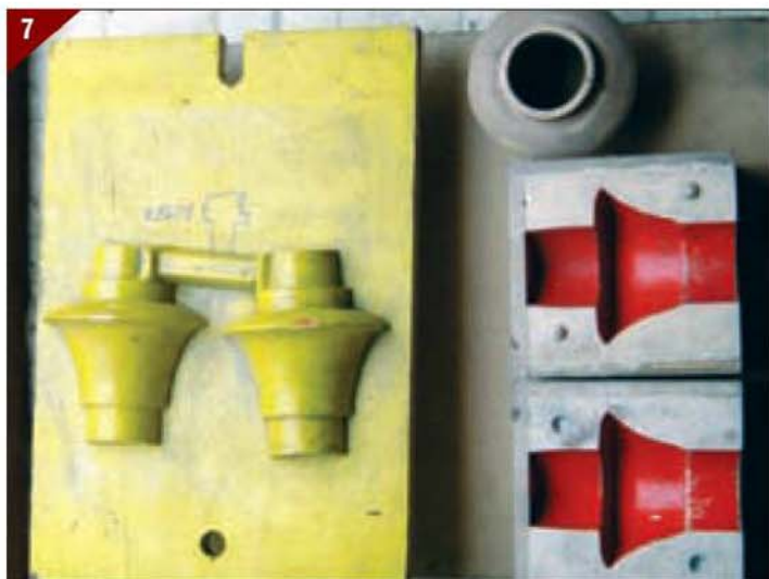
7. Foundry pattern and corebox for chimney casting, with chimney at top. 8. Machining the groove in a cab handrail. 9. Water tank filler support - saddle tank pictured.
