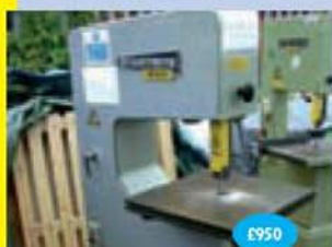
Startrite 18-5-5 240 volts bandsaw; 18" throat / 5 speed / non ferrous
