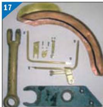
17. Front mudguard components with full-size equivalents for scale.
