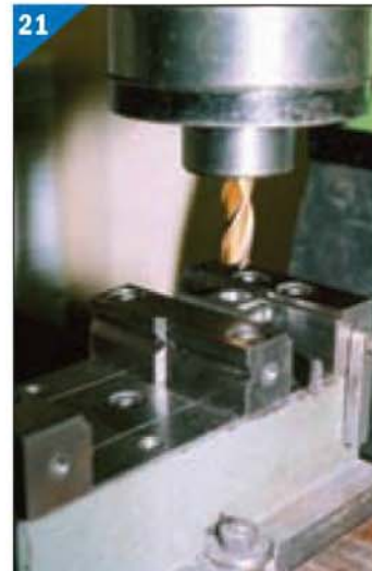
18. Machining the rebates either side of the stud holes. 19. Turning a boss on a bearing cap. 20. Machining the outside of an oil reservoir. 21. Cleaning up the bore of a bearing pedestal. 22. Bearing pedestals and bearing caps at various stages of machining.
