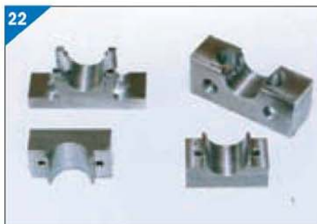
18. Machining the rebates either side of the stud holes. 19. Turning a boss on a bearing cap. 20. Machining the outside of an oil reservoir. 21. Cleaning up the bore of a bearing pedestal. 22. Bearing pedestals and bearing caps at various stages of machining.
