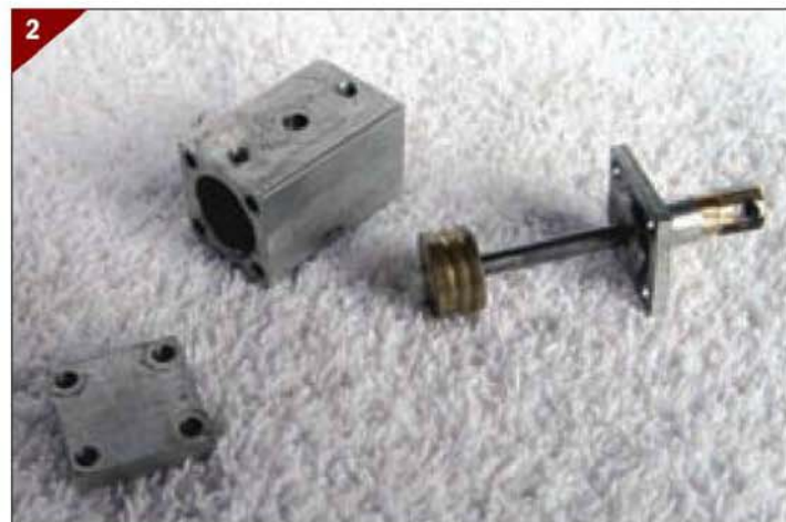
1. Motor complete with red rubber band. 2. Component parts of cylinder assembly.
