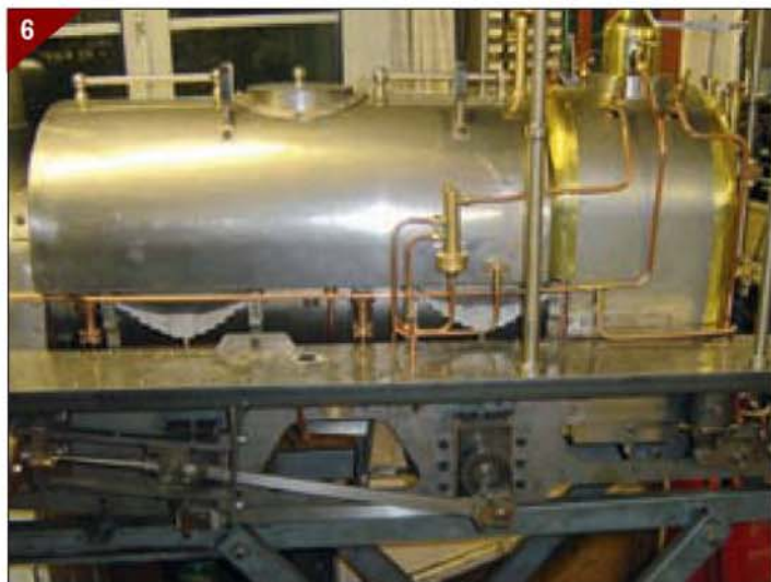
6. Broadside view of left pipework. 7. Left view of complete locomotive. 8. Nested valve gear components in four different thicknesses from the laser cutter.
