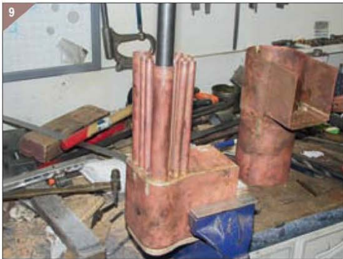
9. Carefully pulling the tubes back in-line.
