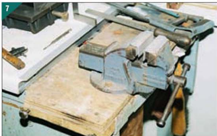
7. Attachment to allow metalworking on a woodwork bench. Bolts lock the vice to the bench.
