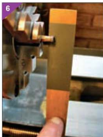
6. Polishing the circumference of a screw head.
