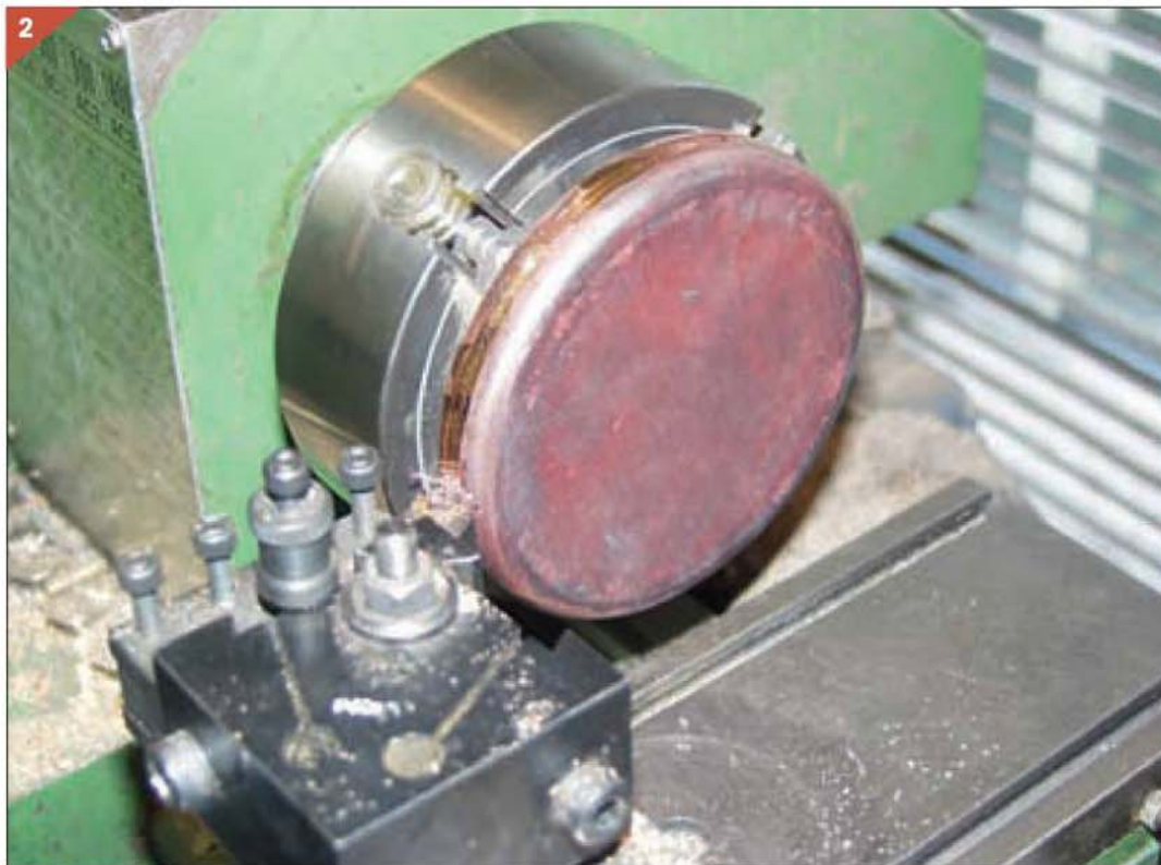
2. Trimming front tube plate to size. 3. Trial assembly. 4. Throat plate attached to barrel. 5. The 'valley' is not filled but there is a fillet of silver solder. 6. The clamp invention that caused a lot of grief.
