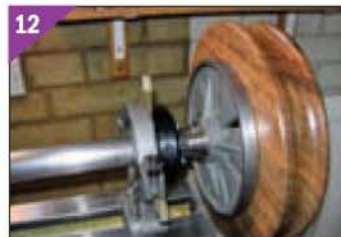
11. The magnetic circuit, finished in black. 12 Extending the mandrel of the Myford to turn the wooden base.
