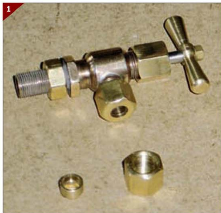
1. A finished steam valve, with spare union nut and nipple.
