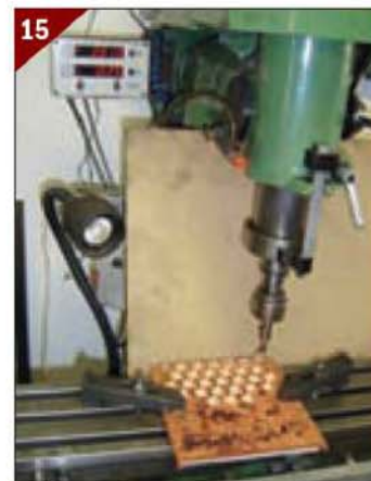
15. Boring the tube holes to size.
