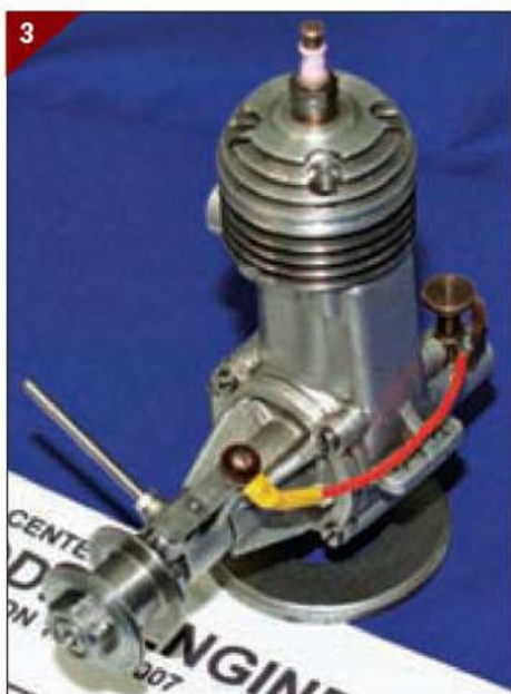
3. The ever-popular Atom Minor 2-stroke engine.
