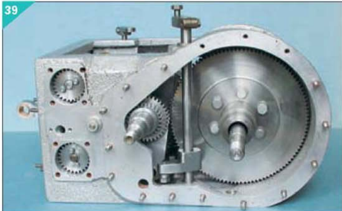
39. Engine assembly, feed pump side.
