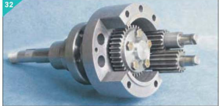
32. View of half the differential assembly. 33. The built up crankshaft assembly. 34. Piston rod, con-rod, crosshead and associated parts.
