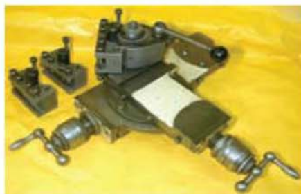
Pultra Compound Slide with Multifix Toolpost, £350.00 plus vat.
