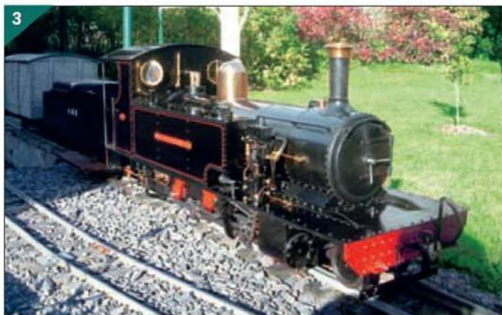
3. The steam operated air-pump is visible on the running boards of Aquila. Its performance was prototypical until the steam pipe was lagged (see text).
