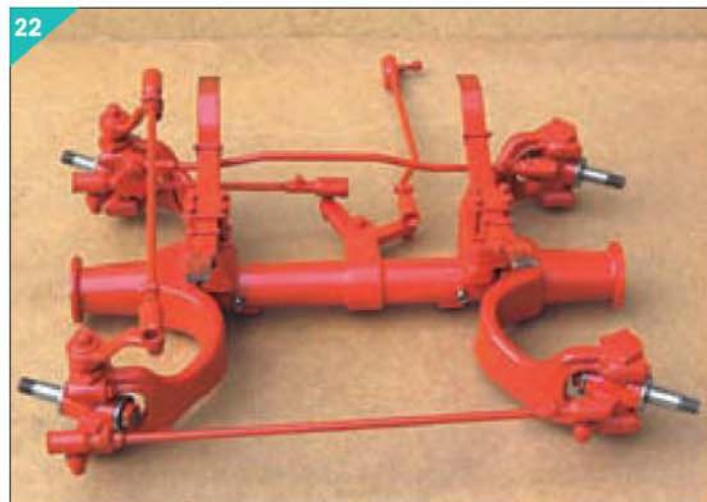
22. The complex front steering bogie assembly shown without its road wheels.
