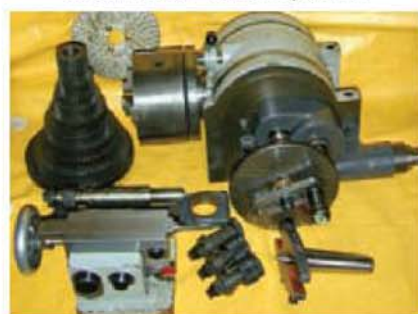
Elliott 4 1/2" Universal Dividing Head & Tailstock, Chuck, Gears Etc, VGC, £525.00 plus vat
