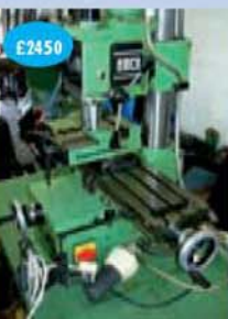
Emco FB2 vertical precision Austrian milling machine complete with stand, power feed, vice and drill chuck
