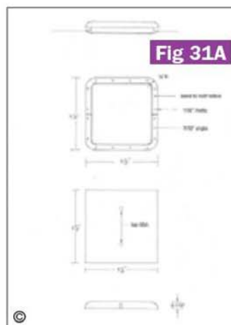
Fig 31. Cab lookout beading and handrail details.
