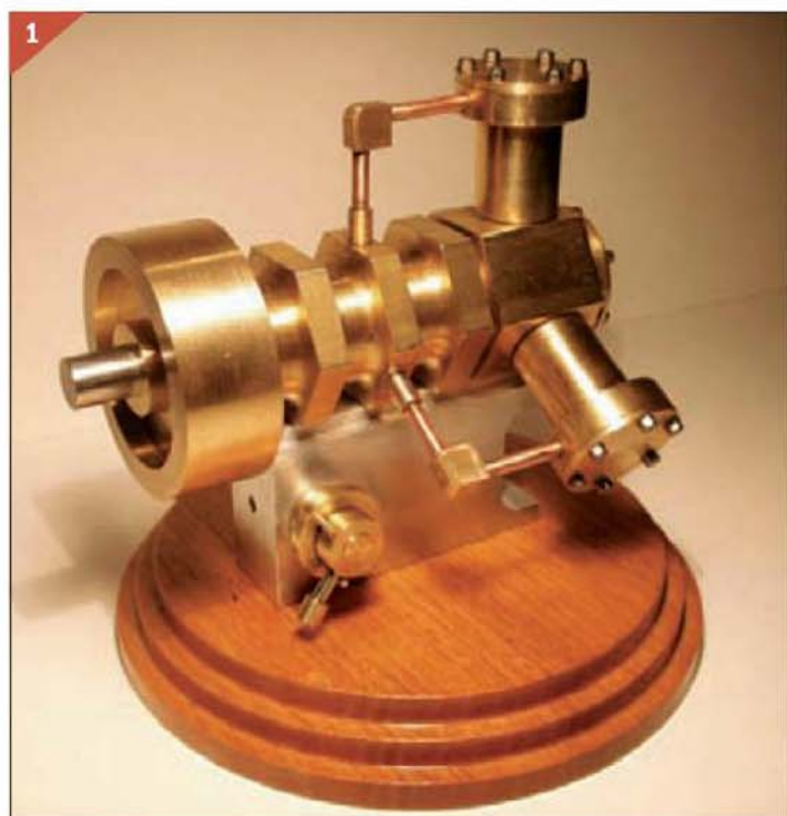
1 to 3. Three views of the 3-cylinder radial engine built by the author.
