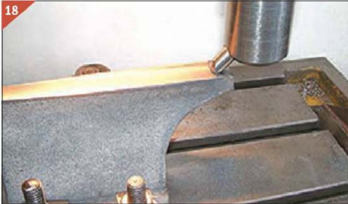
18. With the rough surfaces cleaned up a fly cutter was used to obtain the required finish on the top frame.
