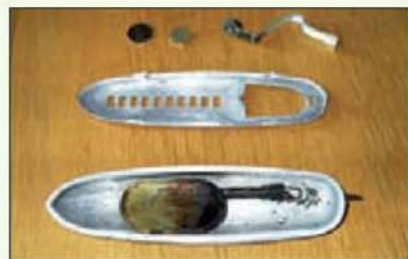
Chris Finn's pop-pop boat showing the motor unit with its single pipe outlet.
