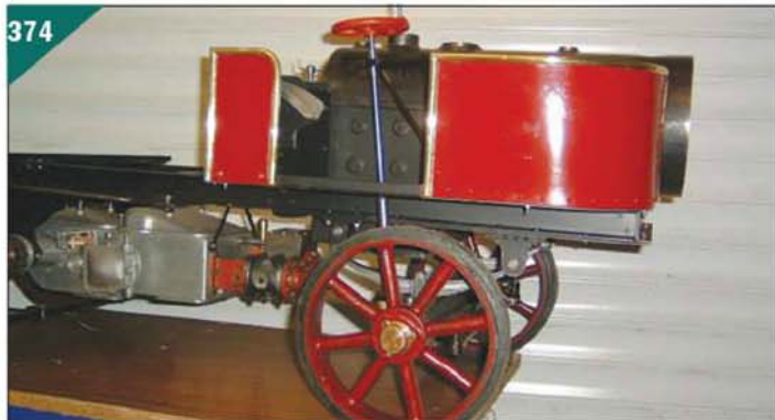
374. On the locomotive version the steering shaft leans back. (photo: Stan Nilper).
