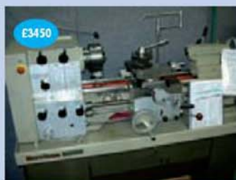
Harrison M300 lathe 6" x 24" complete with gearbox, power cross feed and cabinet stand
