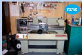
Harrison M250 lathe, 5" x 30" (long bed) complete with gearbox, power cross feed and cabinet stand
