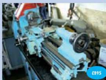
Viceroy 5" x 24" precision screwcutting lathe, 240 volts
