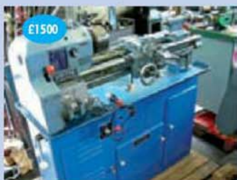
Boxford AUD lathe, 4 1/2" x 22" centres complete with gearbox, power cross feed and tooling and cabinet stand
