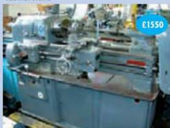
Harrison L6 lathe 6" x 24" complete with gearbox, power cross feed and cabinet stand
