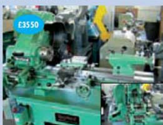
Myford Super 7B lathe complete with gearbox, power cross feed and cabinet stand
