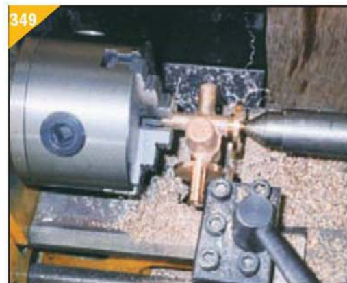
349. The back face of the feed water flange being carefully machined for the fixings (photo: John Thompson).
