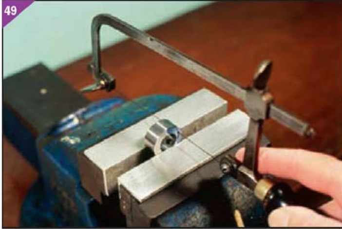
49. Using a piercing saw to cut between the holes.
