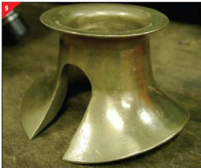
9. The highly-recognisable GWR safety valve cover as a lost-wax casting.
