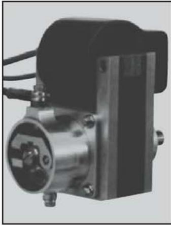
One of the miniature magnetos produced from the Minimag Co. kit. The same coil can be used in a battery ignition system.
