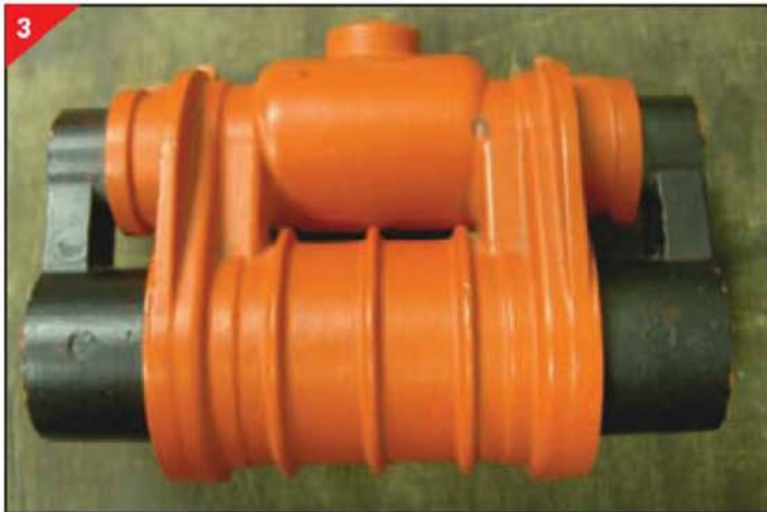
3. Penrhos Grange cylinder pattern showing fine details in reinforcing ribs around the cylinder.
