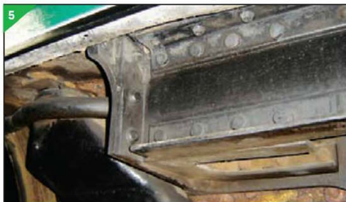
3. Top of rear footstep. Note the angle brace bolted to the buffer beam.
