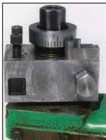
Completed micrometer adjusted toolpost.
