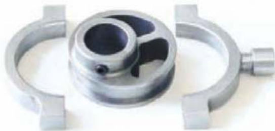
34. The eccentric strap and sheave after all machining operations had been completed.
